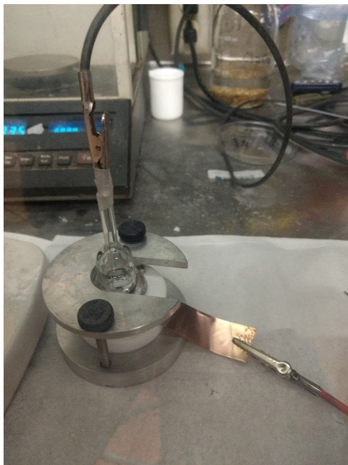
Figure 4-5. Open cell set up for electrografting of olefins onto porous silicon. The copper working electrode is shown on the bottom, while the platinum wire counter electrode is passed through the top and subsequently wrapped in parafilm to prevent electrolyte evaporation.
