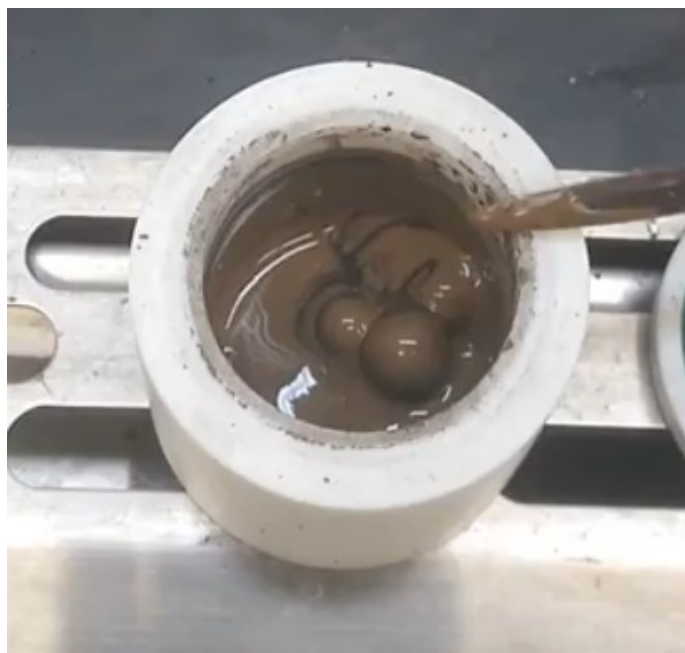
Figure 3-42. A slurry of Si-dodecyl functionalized nanoparticles in water. Light brown particles can be seen suspended above the darker brown slurry underneath.
