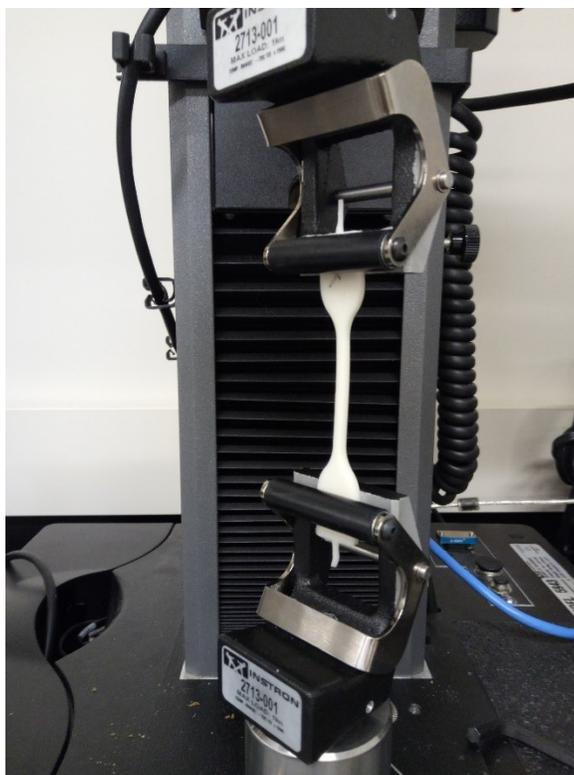
*Figure 3-2: the tensile test system used for studying the basic mechanical properties in the experiment.*
