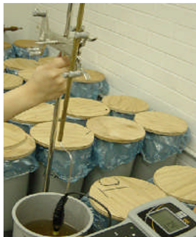
Fig. 3.7 DO Measurement Using a Supporting Stand
