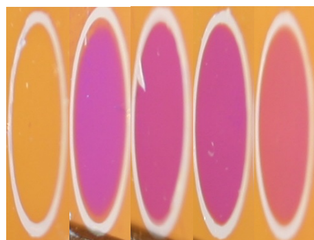
Figure 8.14. Alumina surface with exposure to (left to right) Ca and EDTA, prothrombin with Ca, prothrombin with Ca and EDTA, prothrombin control, and prothrombin with EDTA. All solutions of prothrombin were at concentrations of 0.1 mg/ml with constituents of 1 mM Ca and 1 mM EDTA.
