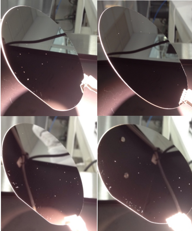
Figure 7.22. Wafers viewed in a bright box to examine tantalum coatings deposited in the NAIT sputter system.
