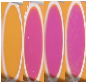
Figure 8.20. The alumina surface exposed to (left to right) Mg/Ca ions in solution, prothrombin with Mg/Ca ions, prothrombin control, and prothrombin followed by Mg/Ca ion solution. All prothrombin solutions were at 0.1 mg/ml, Mg ion solutions were at 1 mM, and Ca ion solutions were at 2.5 mM.
