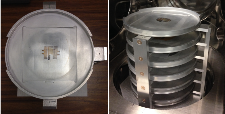
Figure 3.4. The six-platen shelf holder that is loaded into the Floyd load-lock with substrates prior to deposition. The image contains top (left) and side views (right).
