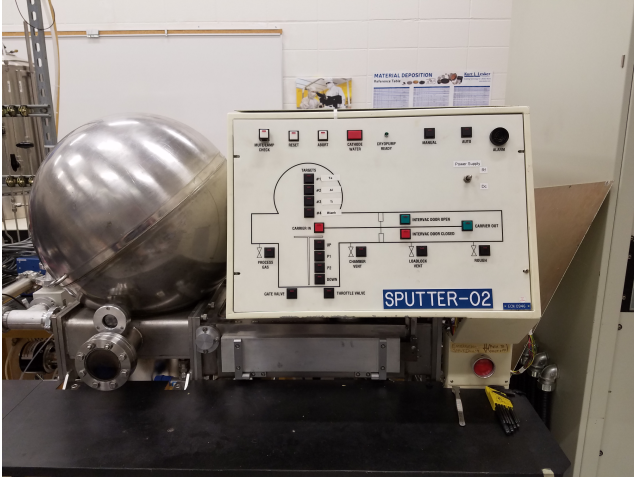
Figure 3.5. NAIT magnetron sputter system used for the deposition of tantalum onto wafers.
