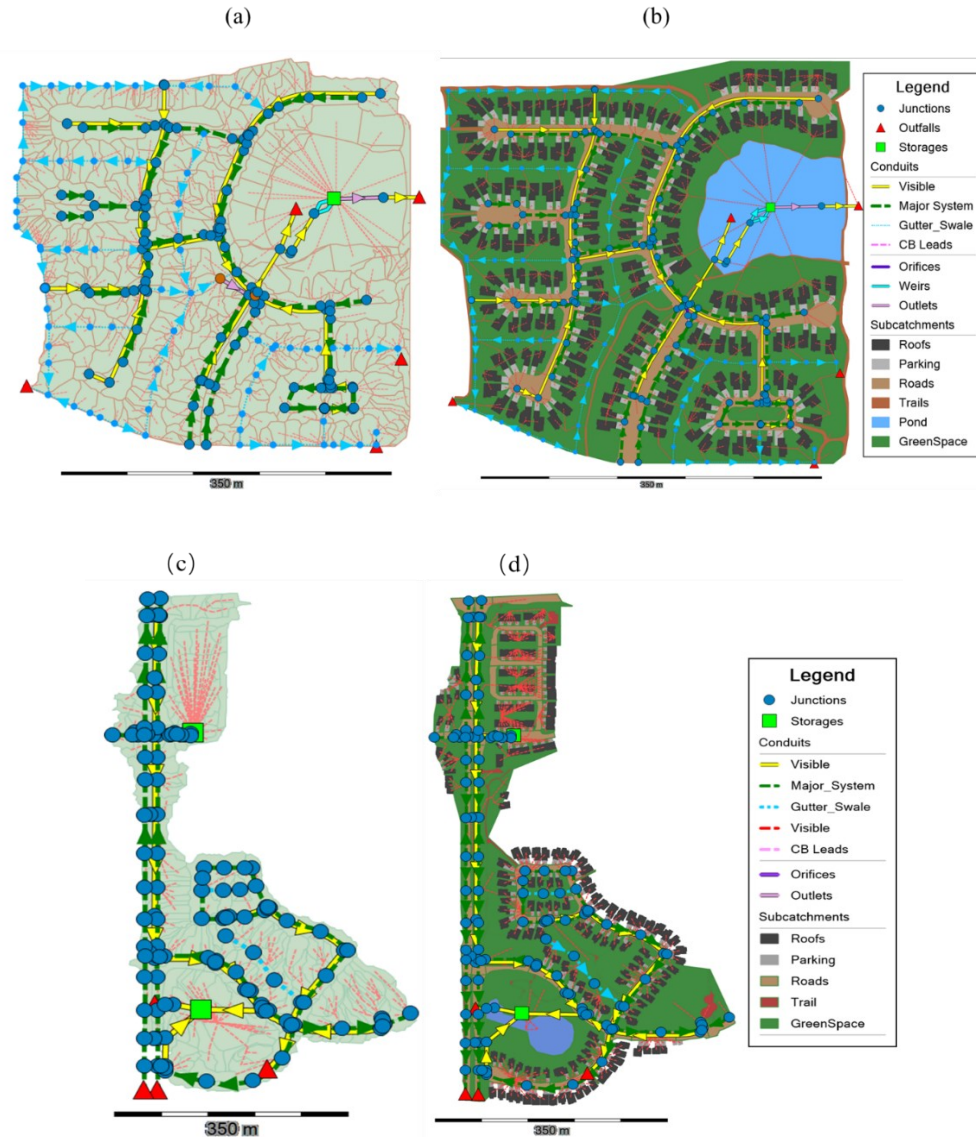
Fig. 3-1. WDT and LCB approach configurations for RR and RO catchment: (a-b) WDT approach and LCB approach for RR; (c-d) WDT approach and LCB approach for RO.
