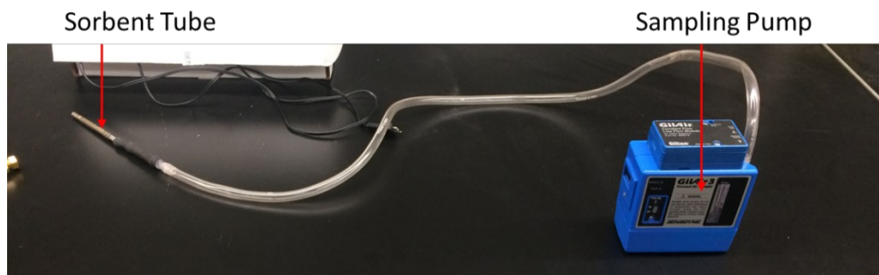
Figure 3.1: Example Sampling Set up Using Sorbent Tubes via Active Sampling for VOCs in the Air
