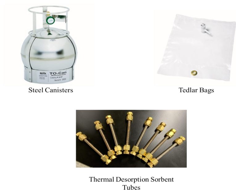
Figure 1.2: Image of Common Air Sampling Devices Including Steel Cannisters, Tedlar Bags and Sorbent Tubes
