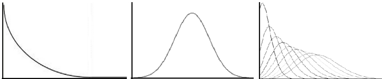
Figure 6. Examples of Power Law, Normal, and Poisson distributions. Each is displayed on a frequency graph. A normal distribution (center) is a distribution for a range of options when the average is the most likely to occur. This type of distribution will typically describe the frequencies of human heights, or test scores in a large class. The Poisson distribution (right) is an adaptation of the normal distribution used for when the mean is already known, and each possible outcome should be equally rare. Each separate line is representative of a different mean. This distribution was originally used in 1898 in a study of how many soldiers had been accidentally killed by kicking horses. The power law (left), which is what is followed by the degree spread in a network, is used to describe populations where most outcomes are the same, but there are extremes that would skew the data if represented in a normal distribution. The power law was first used to describe the distribution of wealth in the United States, demonstrating ‘The Rich get Richer’ effect. In other words, most families have similar incomes but some are incredibly rich and some are incredibly poor.
