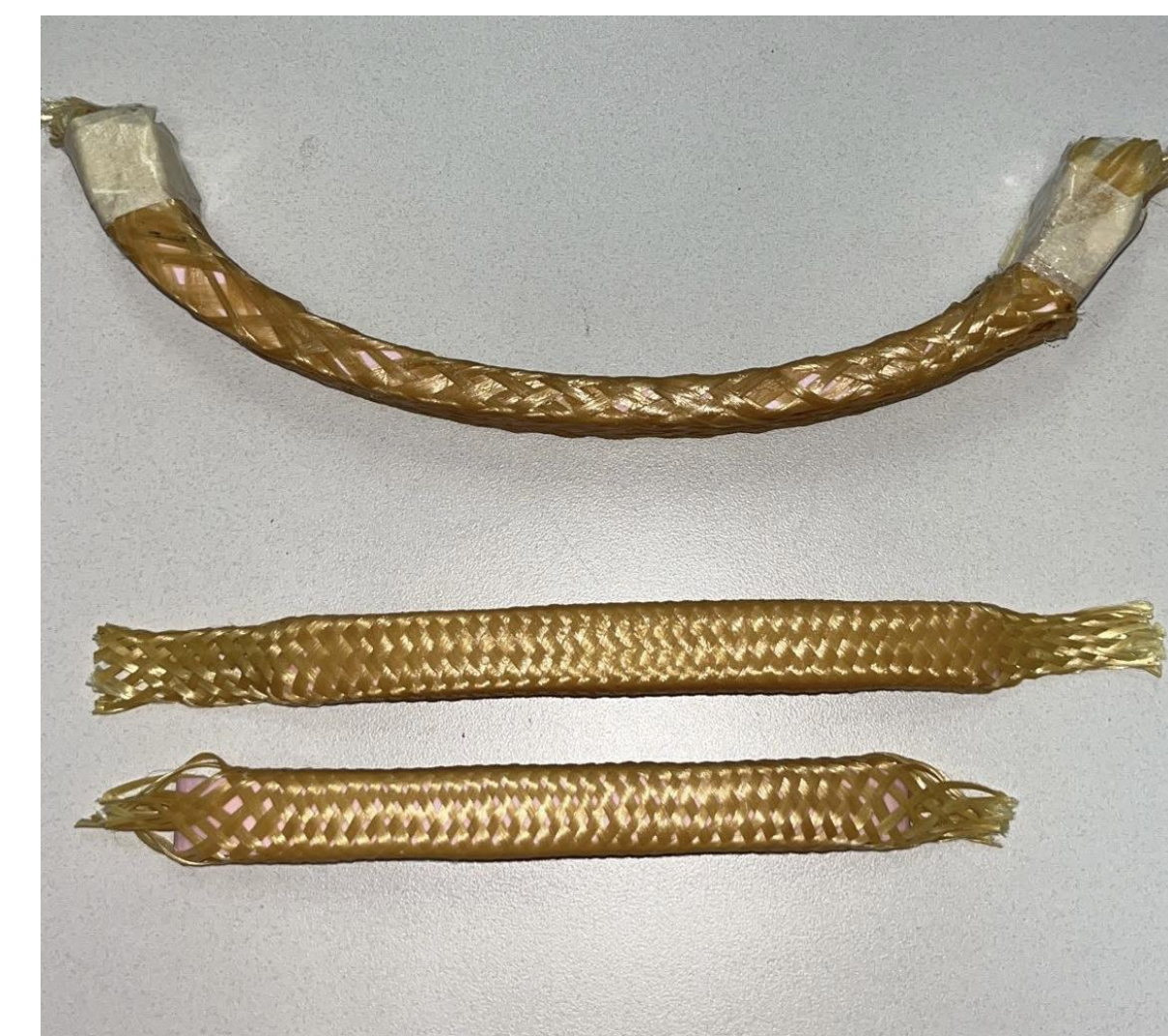
Figure 5: Braids being cured in cold-cure epoxy.
