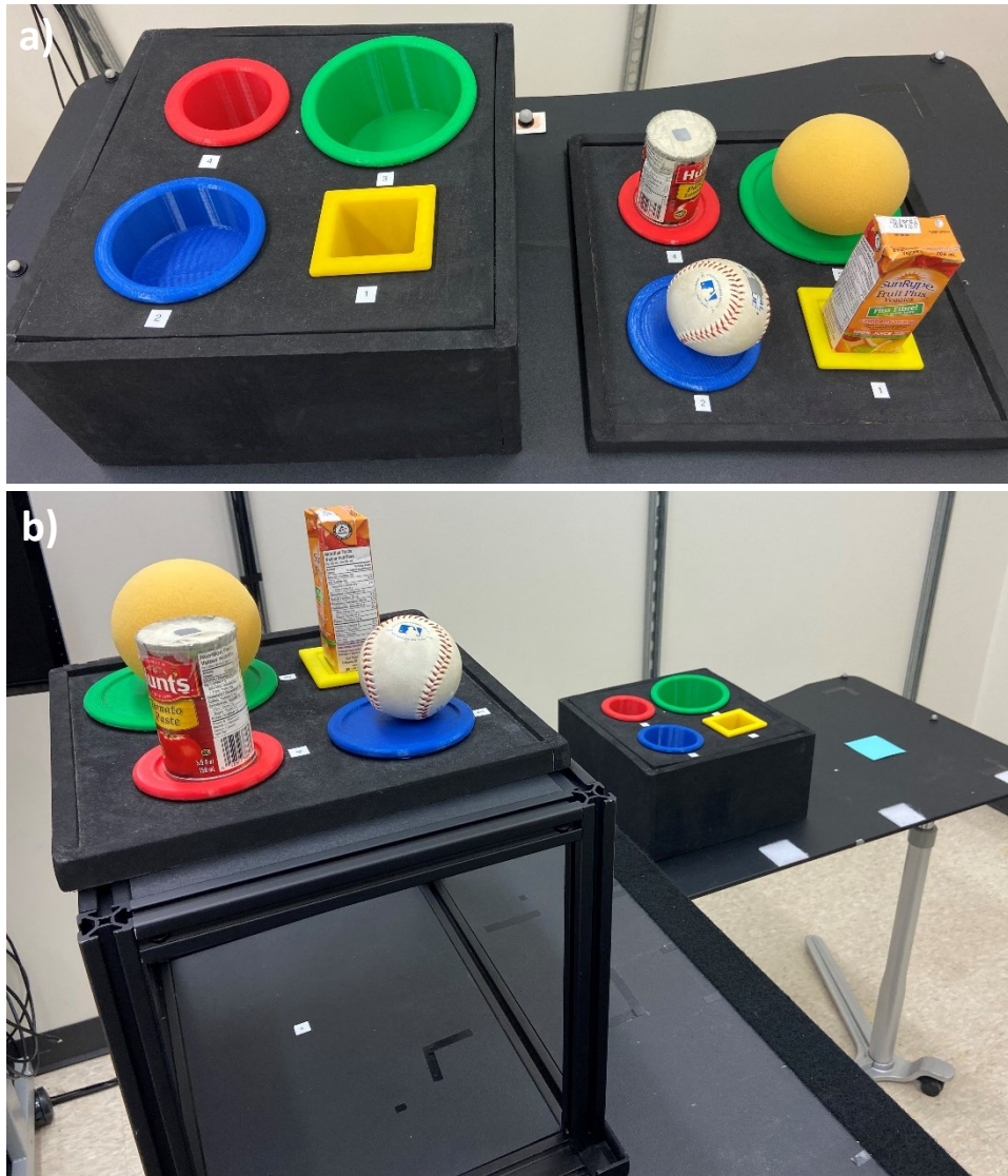
Figure D-1: (a) Each object is picked up and placed into the corresponding well; (b) objects are then picked up from a shelf on the centre cart and placed into the corresponding well.
