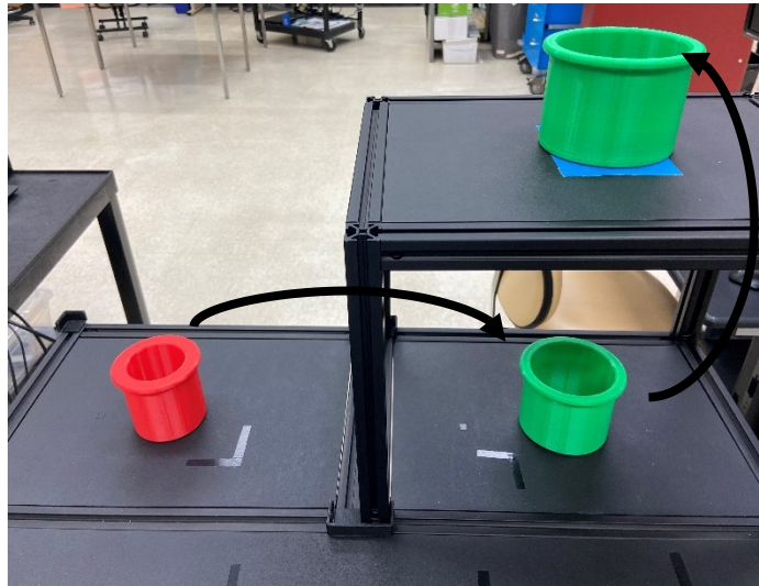
Figure D-4: The small cup is placed into the medium cup, then both cups are placed into the large cup.
