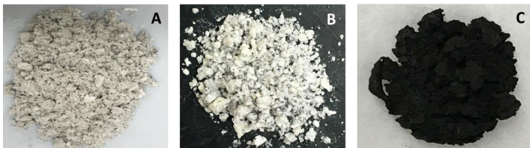
Figure 6.2. Physical appearance of ash powders from barley flour (A), alkali-treated starch (B), and electrolysed starch at 15 V, 120 min (C).
