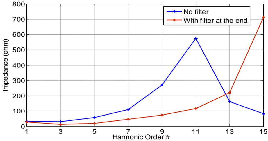
Figure 4.29 Zero sequence frequency scan observed at “Location 3” with filter at end of the feeder
