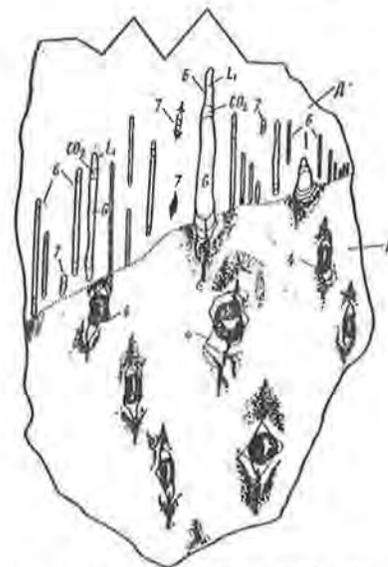
Fig. 31. Crossing of various-age fractures, next healed, with decrepitated (I-I) and polyphase (II-II) inclusions filled to various degrees. Absence of cloudy halo around refilled inclusion A points the earlier refilling than decrepitation.
