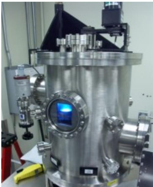
A planar magnetron sputter system with three sources. The gun/substrate configuration is designed for sequential sputtering. The third source can be used for magnetic materials.
