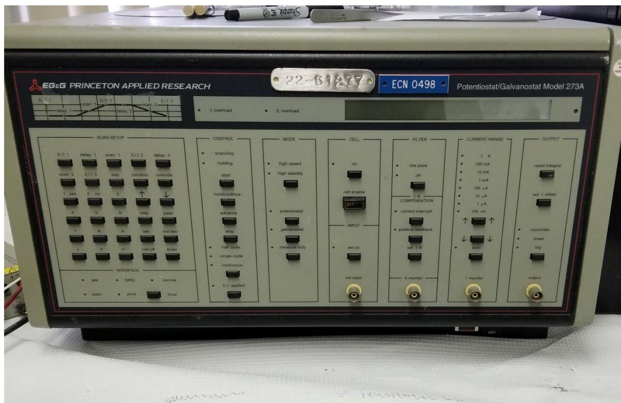
Figure 22. The Princeton Applied Research Potentiostat used for all anodizations.
