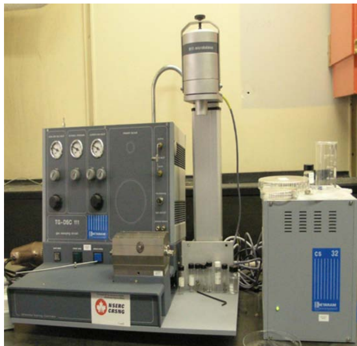
Figure III.9 : The TG-DSC 111 thermoanalyzer used in the worl by Bazyleva, A.B., et al. [16]
