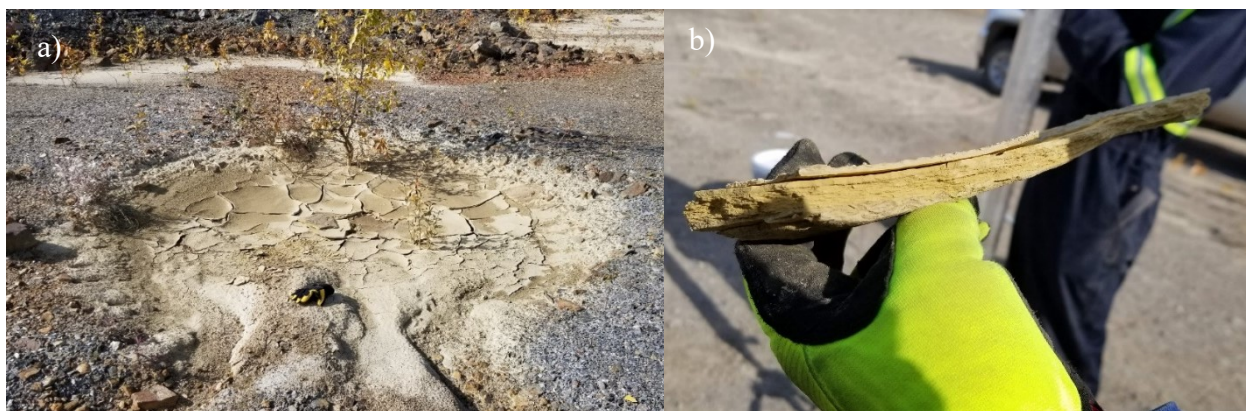
Figure 3.1.4 - a) Preferential Flow Near UW17-BH2 on the Main Dump East, b) Layered Fine Sediment Forming on the Flow Feature
