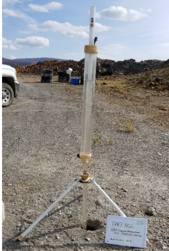
Figure 3.1.6 - Guelph Permeameter Test Conducted at UW17-BH2
