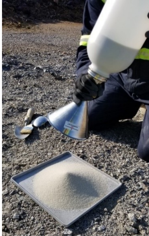
Figure 3.1.7 - In-Situ Density Measurement at UA19-TL1
