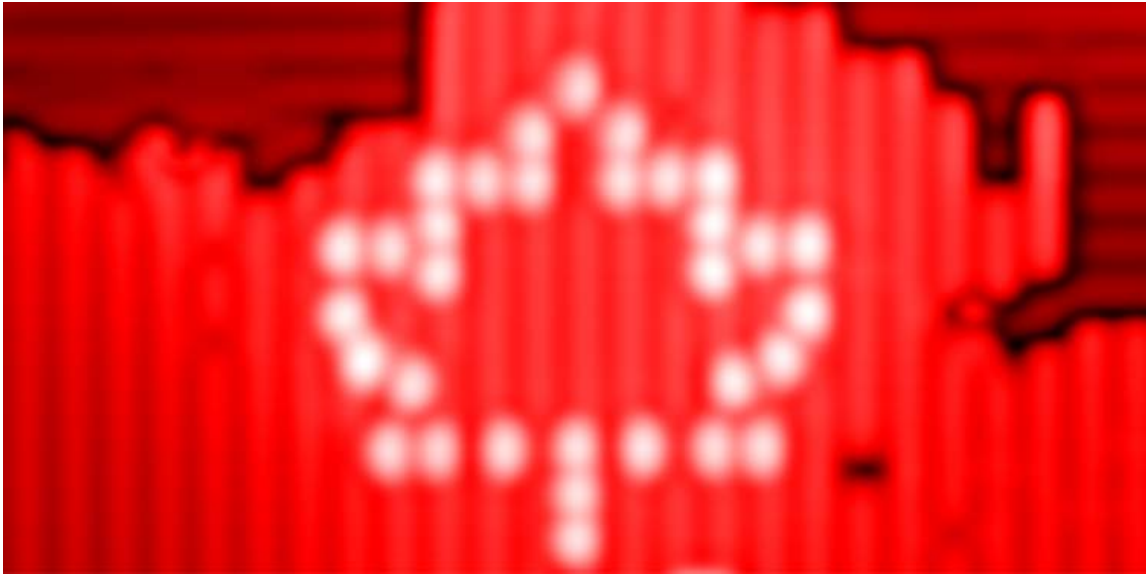
Figure B.3: Perfection ( V = -1.6 V, I = 50 pA, T = 4.5 K, 11 \times 22 nm 2 ). This image is representative of the state of HL in 2017, after the development of HR. Now it was possible to repair the one or two erroneous DBs to achieve perfect large DB structures. The leaf consists of 32 DBs, and it is one of my favorite images.
