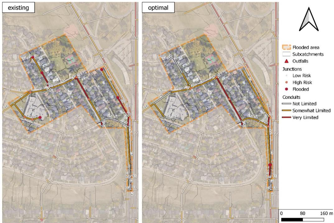
**Figure A18** The comparison of Flooded Area 17 in the study area before (left) and after (right) optimization, under Scenario 1 by using the 1D model.
