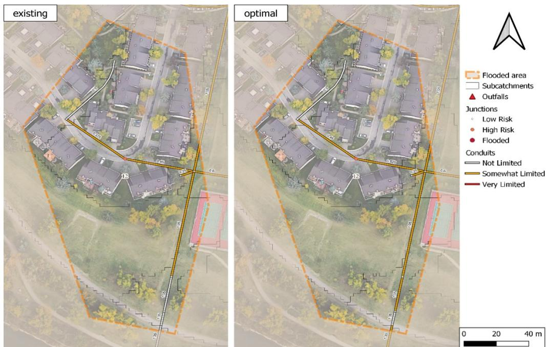
**Figure A13** The comparison of Flooded Area 12 in the study area before (left) and after (right) optimization, under Scenario 1 by using the 1D model.
