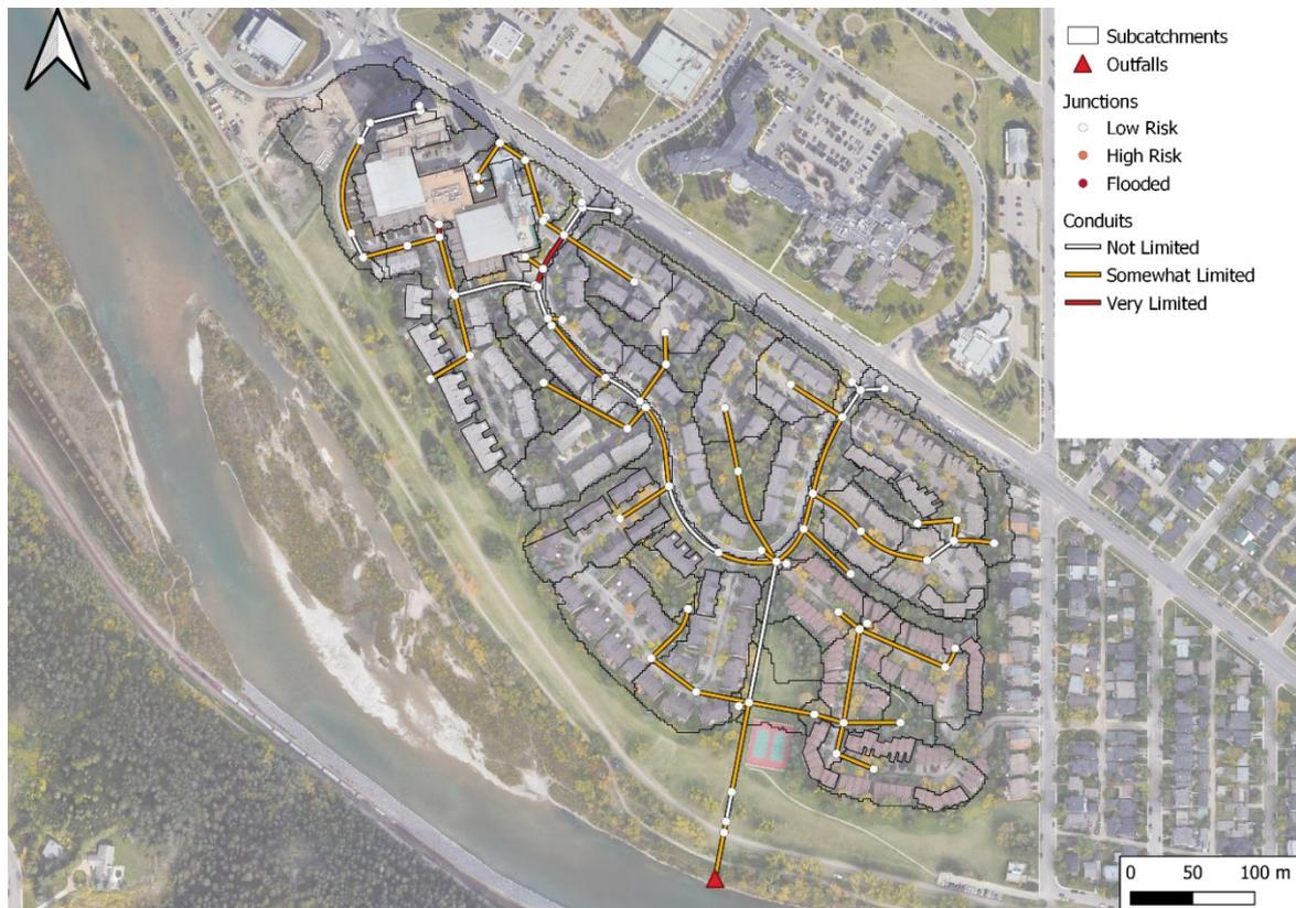
**Figure 4.14** After optimization: manhole flooding risks and storm sewer conduit (pipe) conditions in the test area.
