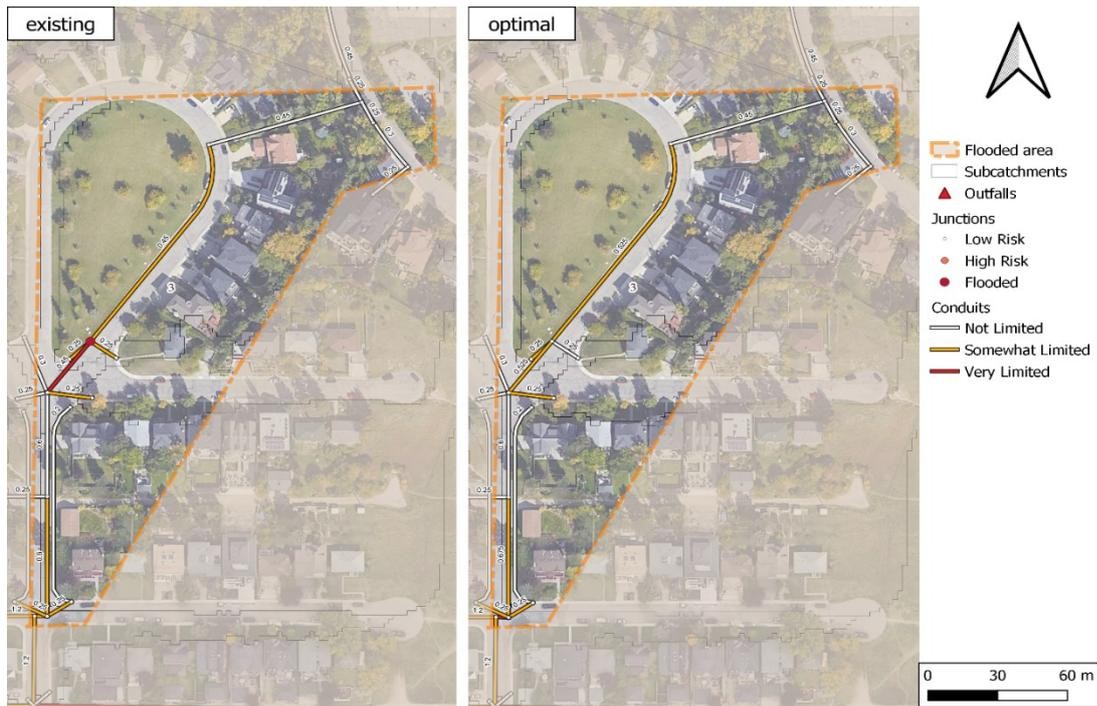
**Figure A4** The comparison of Flooded Area 3 in the study area before (left) and after (right) optimization, under Scenario 1 by using the 1D model.
