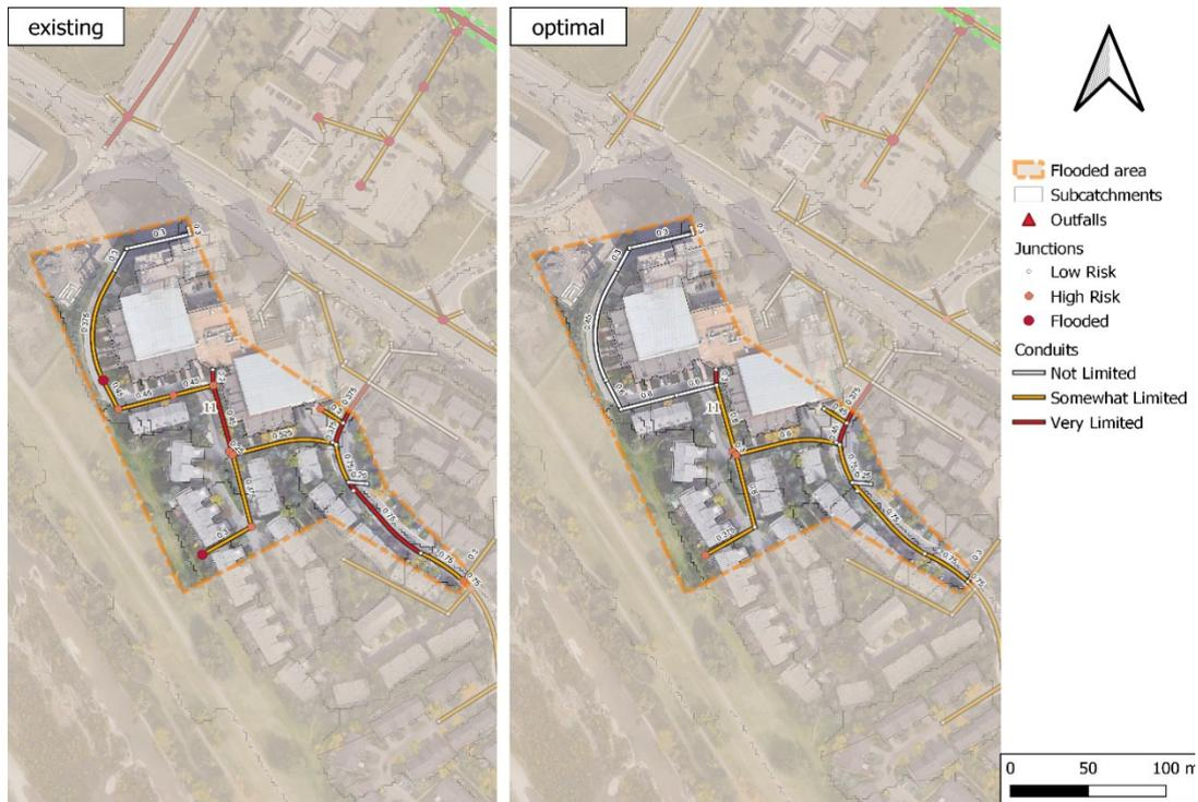
**Figure A12** The comparison of Flooded Area 11 in the study area before (left) and after (right) optimization, under Scenario 1 by using the 1D model.
