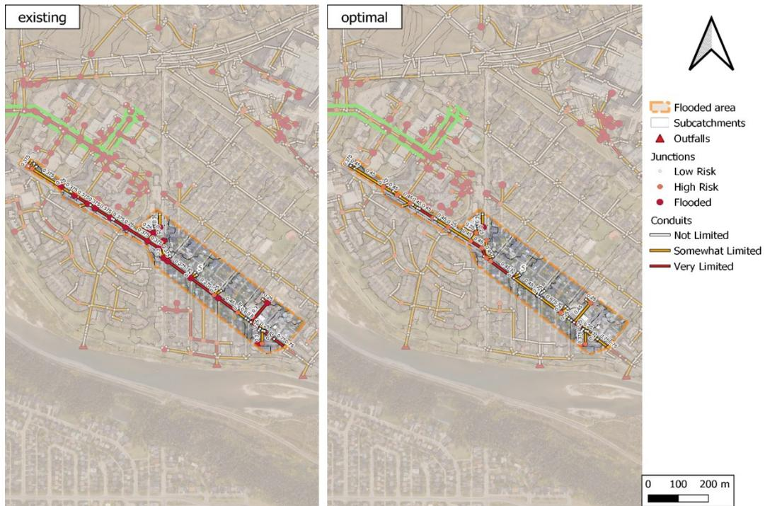
**Figure A6** The comparison of Flooded Area 5 in the study area before (left) and after (right) optimization, under Scenario 1 by using the 1D model.
