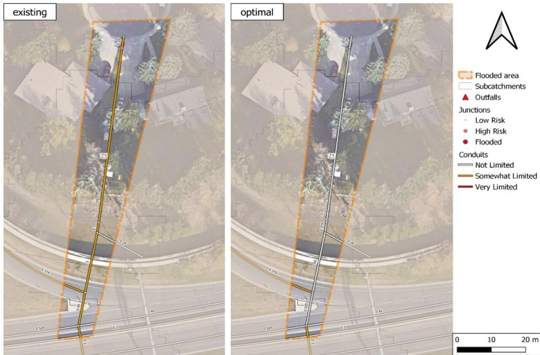
**Figure A26** The comparison of Flooded Area 25 in the study area before (left) and after (right) optimization, under Scenario 1 by using the 1D model.
