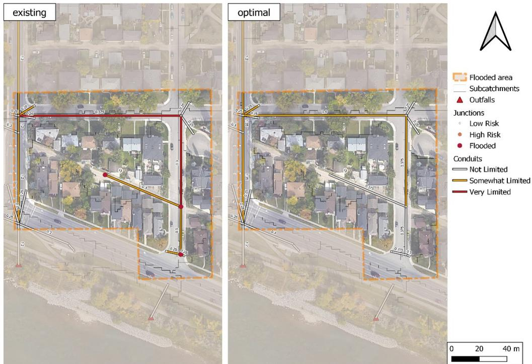
**Figure A10** The comparison of Flooded Area 9 in the study area before (left) and after (right) optimization, under Scenario 1 by using the 1D model.
