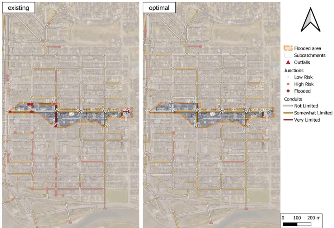
**Figure A34** The comparison of Flooded Area 33 in the study area before (left) and after (right) optimization, under Scenario 1 by using the 1D model.
