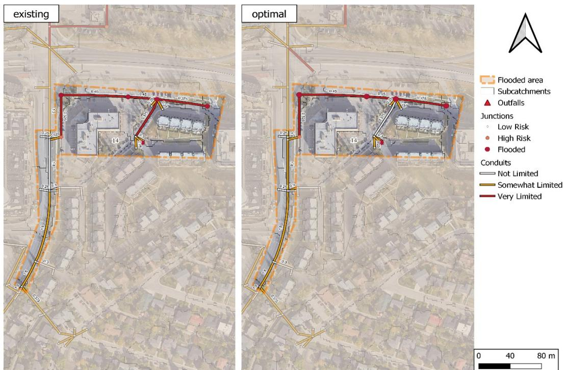
**Figure A15** The comparison of Flooded Area 14 in the study area before (left) and after (right) optimization, under Scenario 1 by using the 1D model.
