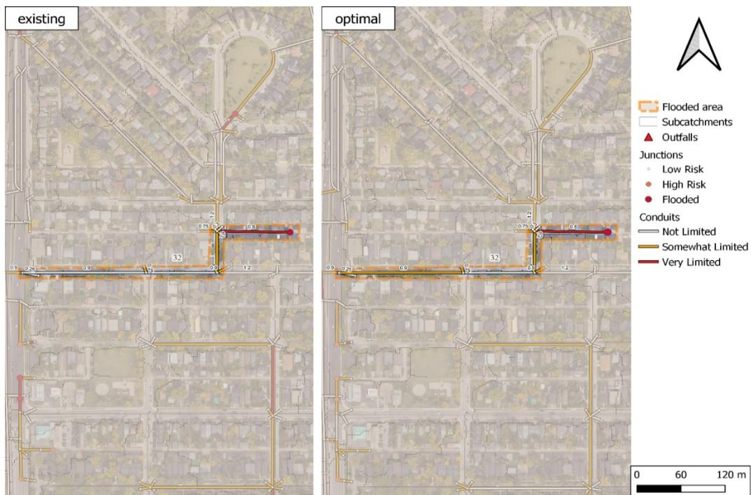
**Figure A33** The comparison of Flooded Area 32 in the study area before (left) and after (right) optimization, under Scenario 1 by using the 1D model.
