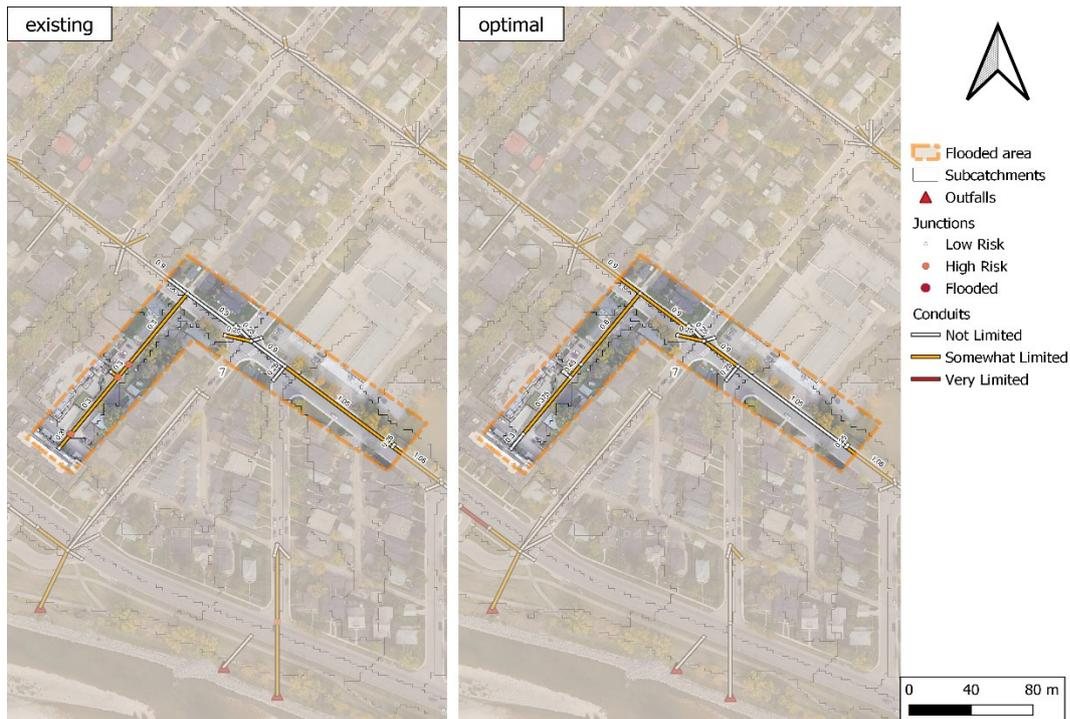
**Figure A8** The comparison of Flooded Area 7 in the study area before (left) and after (right) optimization, under Scenario 1 by using the 1D model.
