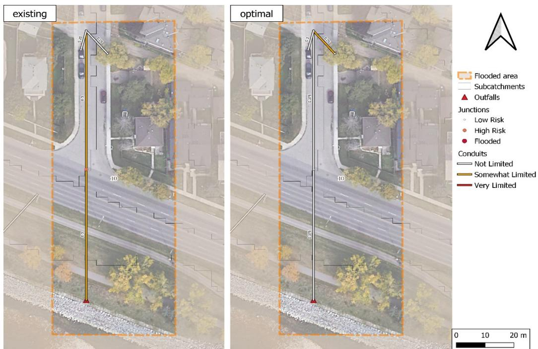
**Figure A11** The comparison of Flooded Area 10 in the study area before (left) and after (right) optimization, under Scenario 1 by using the 1D model.
