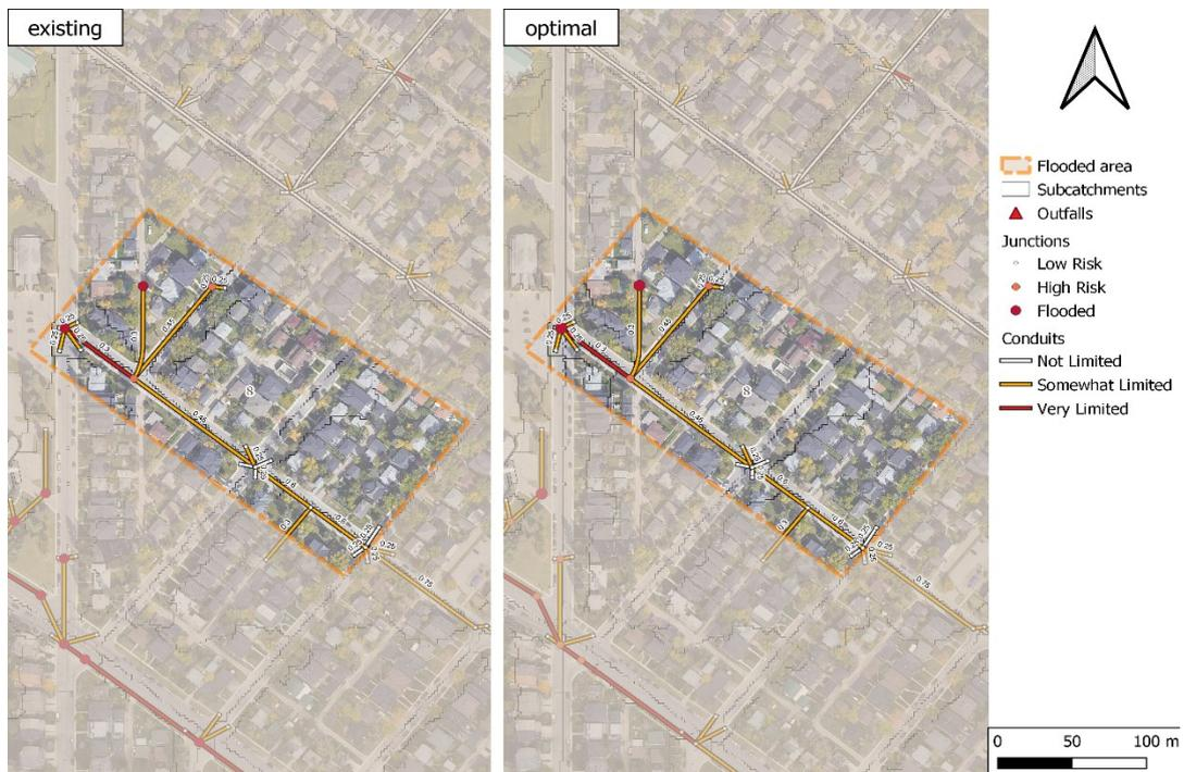
**Figure A9** The comparison of Flooded Area 8 in the study area before (left) and after (right) optimization, under Scenario 1 by using the 1D model.
