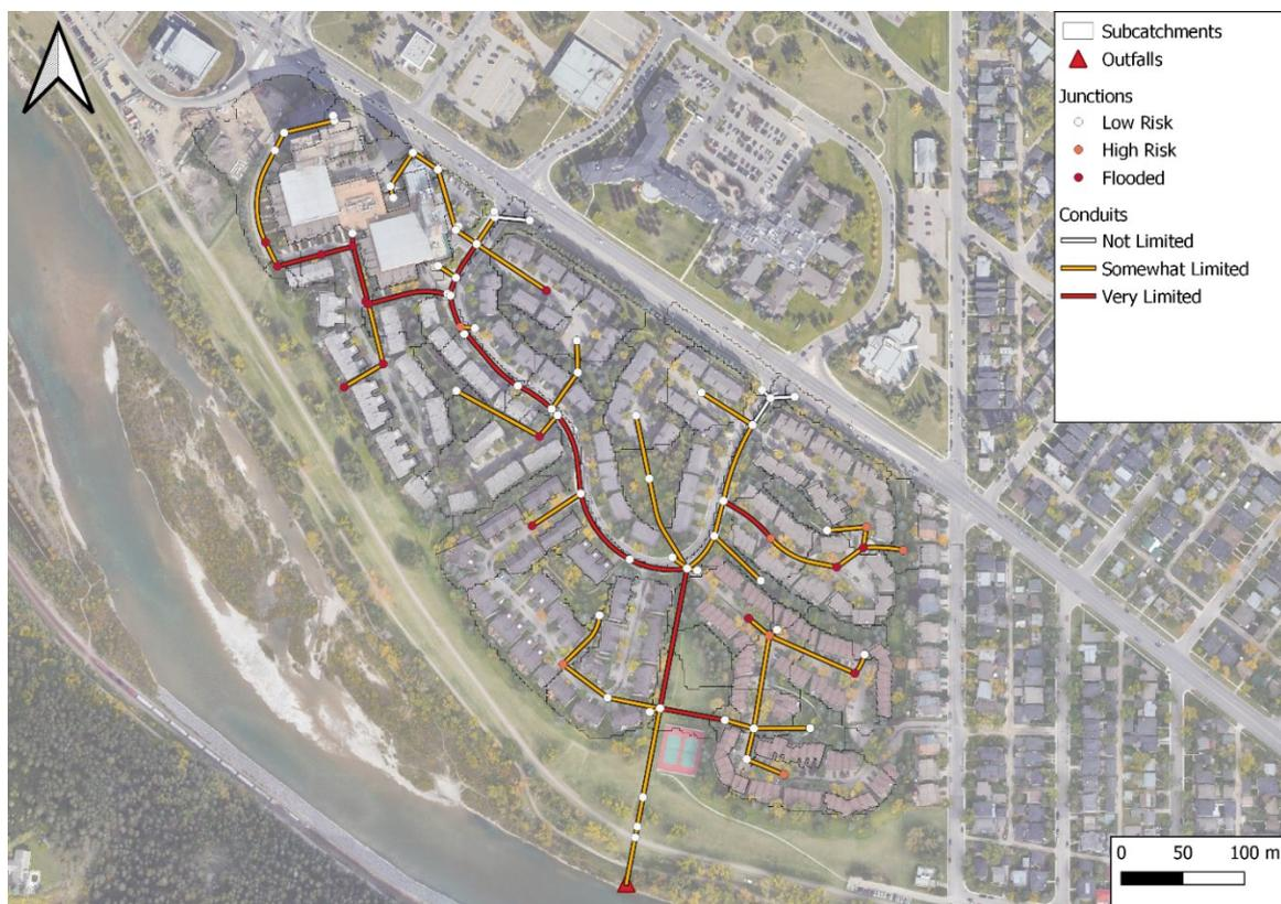
**Figure 4.13** Before optimization: existing manhole flooding risks and storm sewer conduit (pipe) conditions in the test area.
