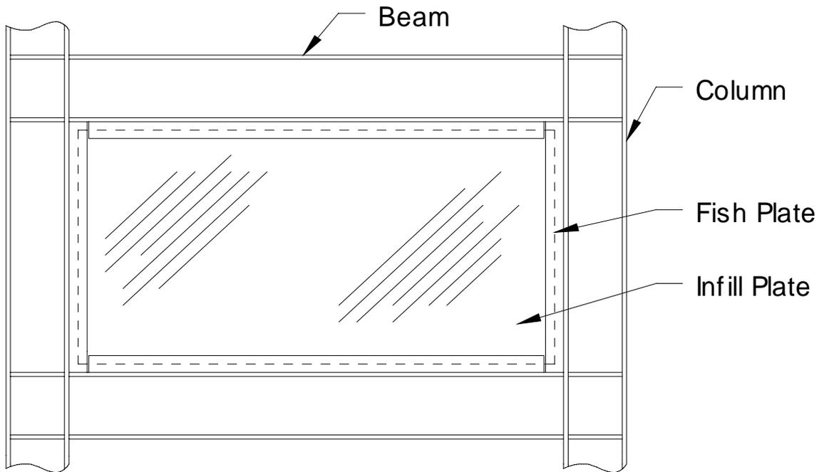
**Figure 3.1** One Storey of Driver et al. [1997] Four-Storey Steel Plate Shear Wall
