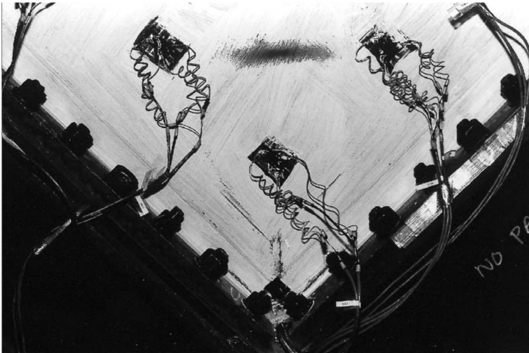
**Figure 4.2** Yielding of Specimen 4 Due to Buckling
