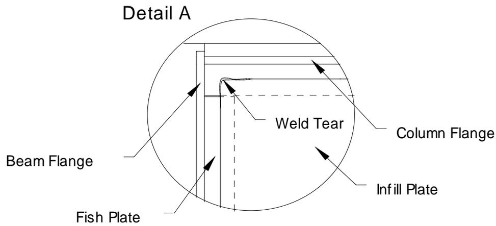
**Figure 2.4** Tear Observed in Timler and Kulak [1983] Specimen
