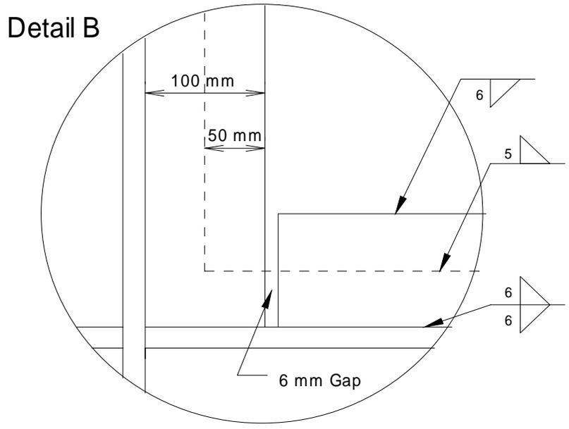
**Figure 3.5** Infill Plate Connection Specimen 2
