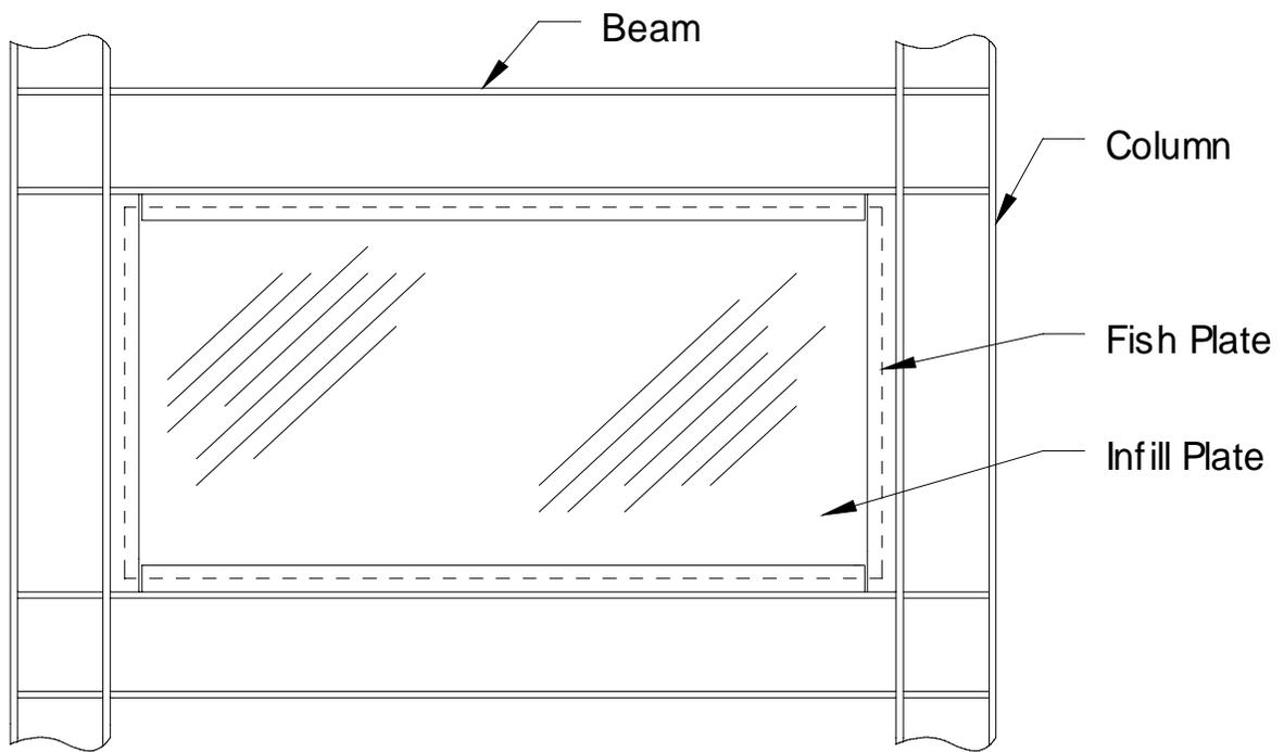
**Figure 1.1** Steel Plate Shear Wall Panel Using Fish Plates
