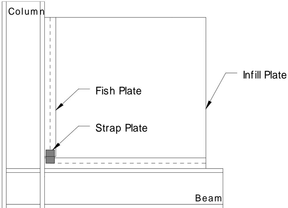
**Figure 2.7** Corner Detail Specimen (Driver *et al.*, 1997)
