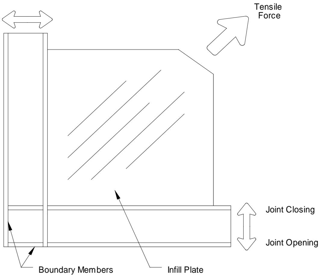
**Figure 3.3** Loading Concept for Infill Plate Connection Tests
