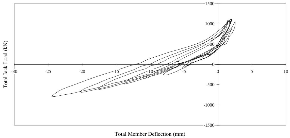
**Figure 4.6** Hysteresis Curves for Specimen 4
