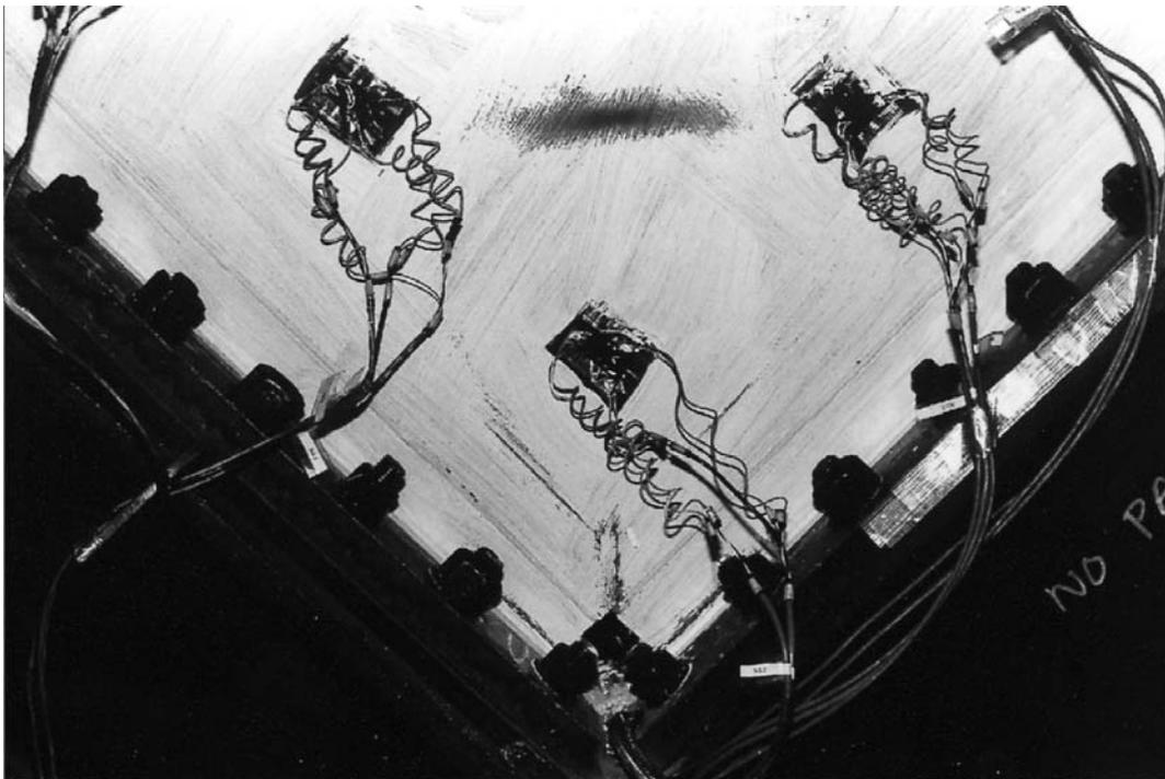
**Figure 4.15** Specimen 4 Corner Detail at End of Testing
