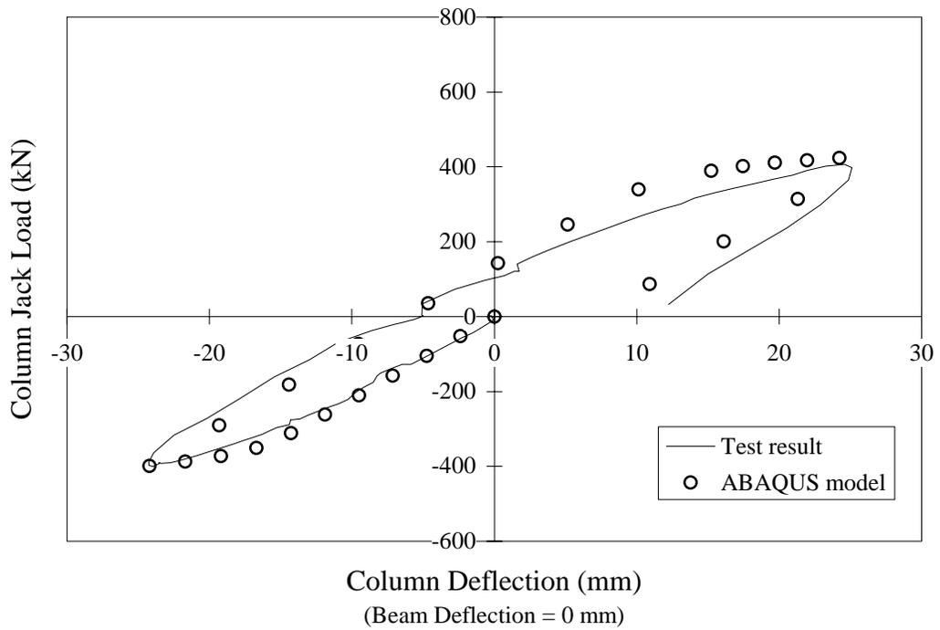
**Figure 5.5** V-Frame Stiffness — Experimental Versus Analytical
