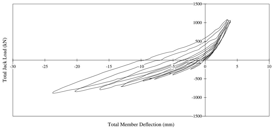
**Figure 4.4** Hysteresis Curves for Specimen 2
