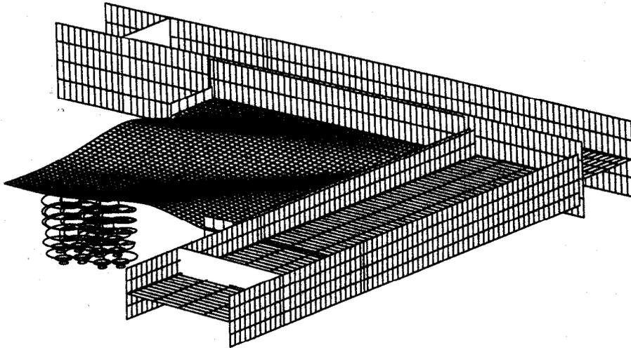
**Figure 6.4** Test Specimen 2 – Comparison of the Observed Deformed Shape with the Predicted Deformed Shape
