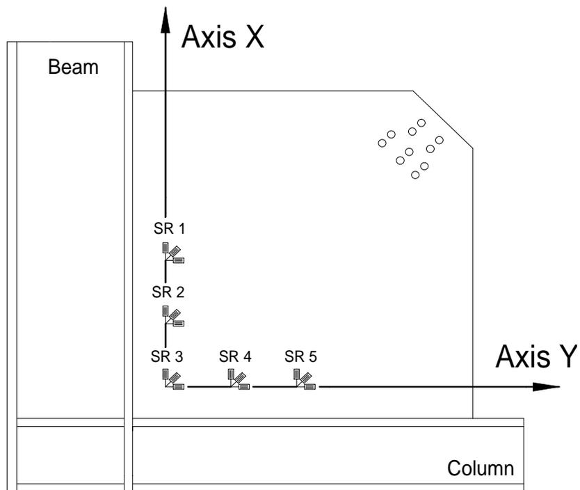
**Figure 4.16** Axes for Strain Orientation
