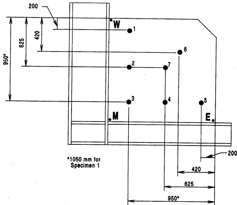
**Figure B.1** Location of Demec Points on Specimens
