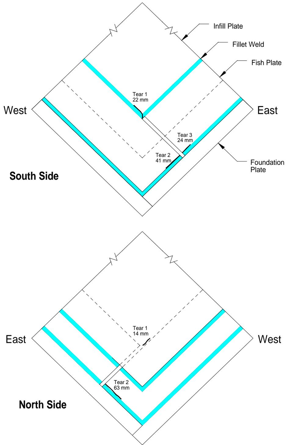
**Figure 4.10** Tears Noted on Specimen 2
