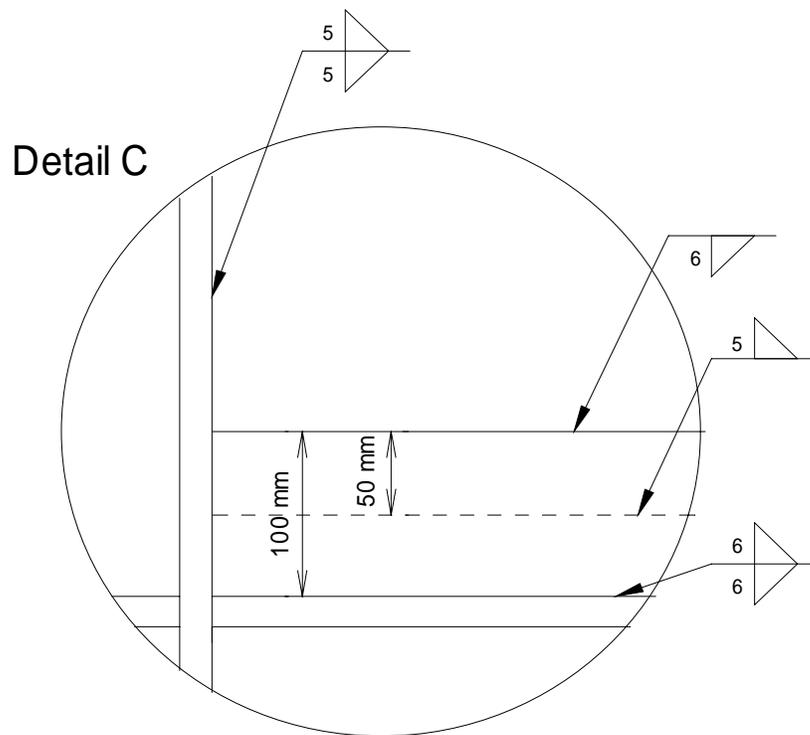
**Figure 3.6** Infill Plate Connection Specimen 3
