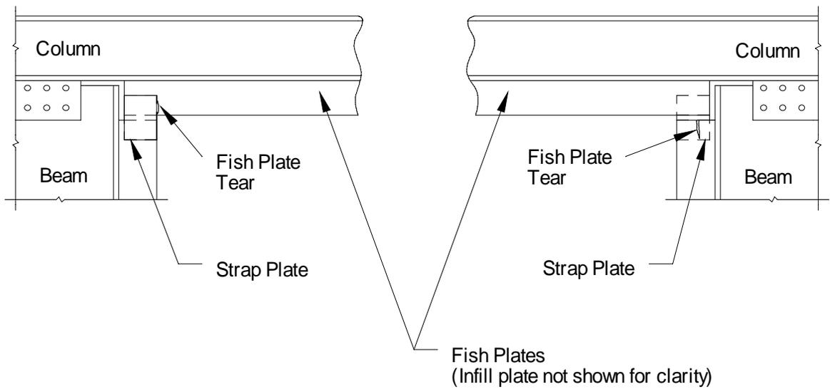
**Figure 2.6** Tear Observed in Tromposch and Kulak [1987] Specimen
