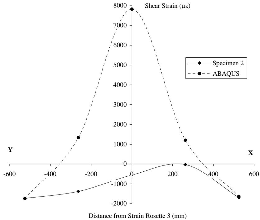
**Figure 6.6** Strain Comparison at Outward V-Frame Displacement
