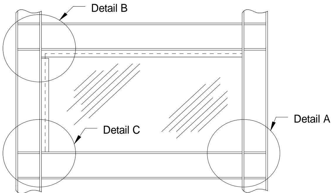
**Figure 3.2** Steel Plate Shear Wall Panel Using Two Fish Plates
