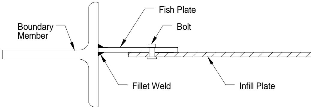
**Figure 2.1** Bolted Infill Plate Connection Details
