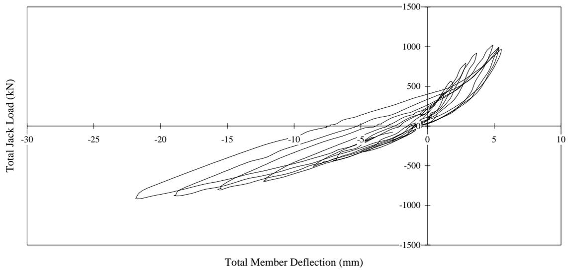
**Figure 4.5** Hysteresis Curves for Specimen 3
