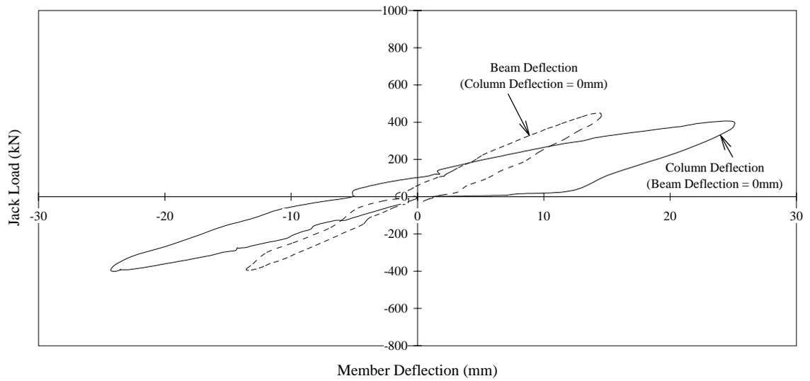
**Figure 4.7** V-Frame Load Versus Displacement Response
