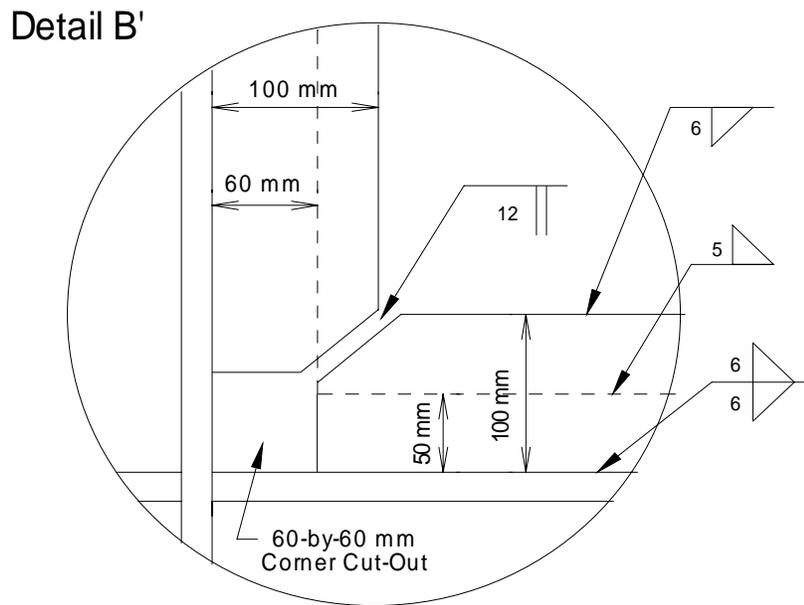
**Figure 3.7** Infill Plate Connection Specimen 4
