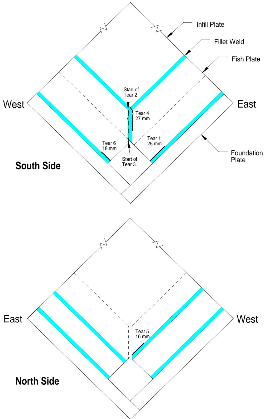
**Figure 4.14** Tears Noted on Specimen 4
