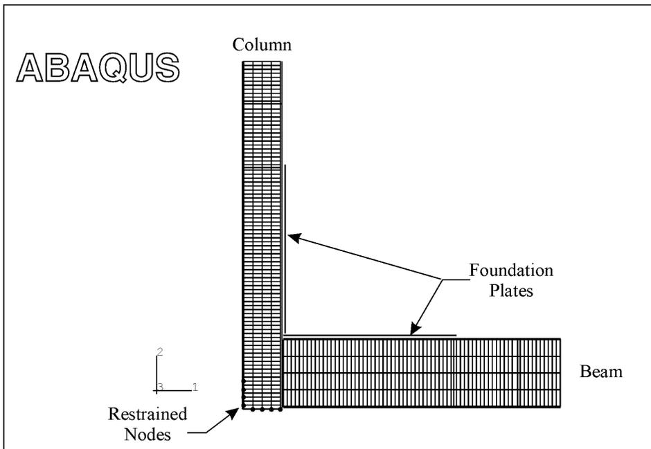
**Figure 5.1** V-Frame Finite Element Model
