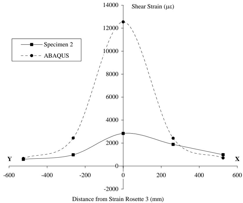
**Figure 6.5** Strain Comparison at Inward V-Frame Displacement
