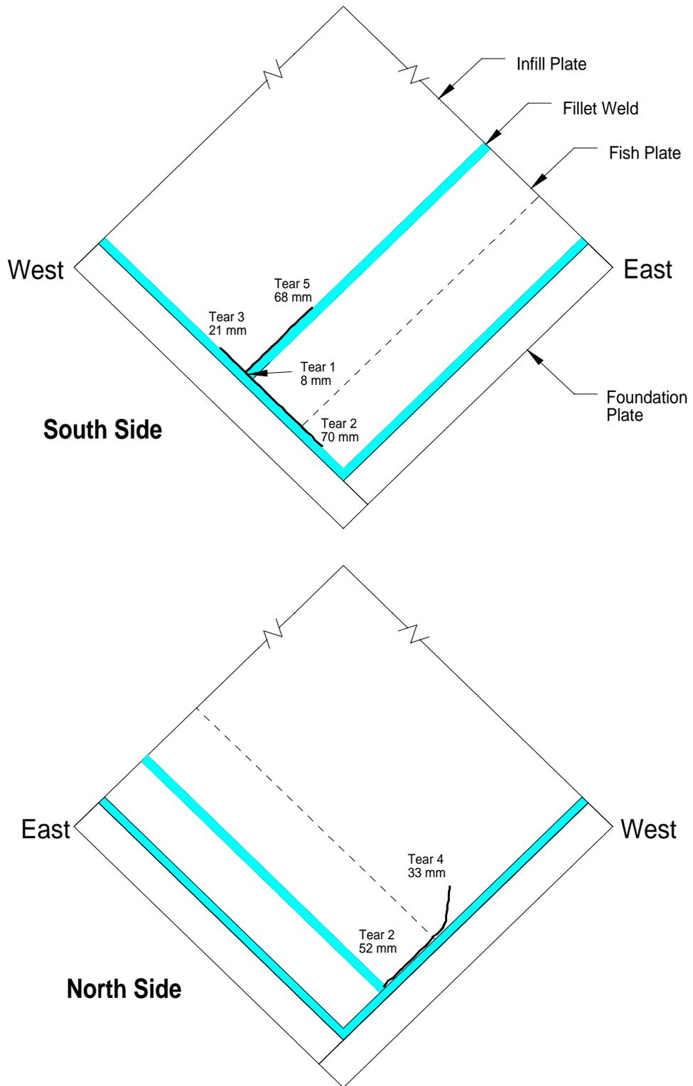
**Figure 4.12** Tears Noted on Specimen 3
