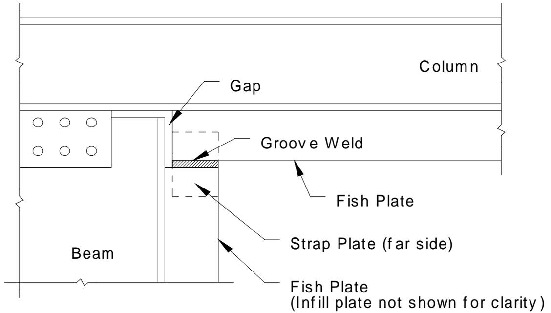
**Figure 2.5** Tromposch and Kulak [1987] Corner Detail
