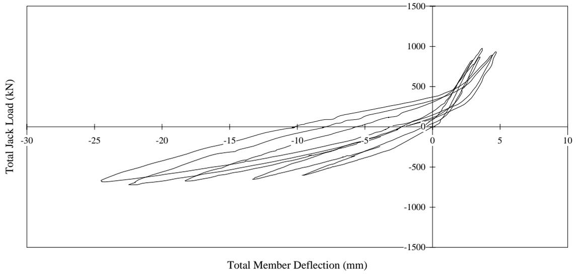
**Figure 4.3** Hysteresis Curves for Specimen 1
