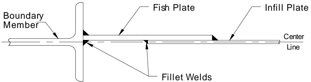
**Figure 2.2** Welded Infill Plate Connection Detail
