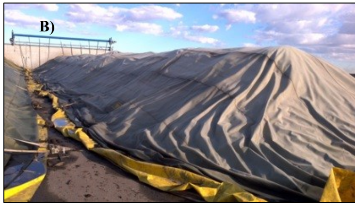
Figure 5-1. A view of experimental pile: a) the process of the aerated static pile building with the vertical mixer; b) the final set-up of the pile after it is covered with the selective membrane
