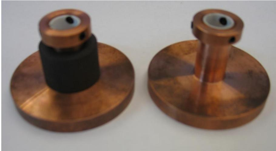
Figure 3.4: OFC headpiece, insulating Macor insert, and Graphalloy bushing used to facilitate heat transfer from the LN<sub>2</sub> cooling block to the substrate holder, while allowing for  $\phi$  rotation. Three set screws are used to secure the headpiece to the rotational shaft.
