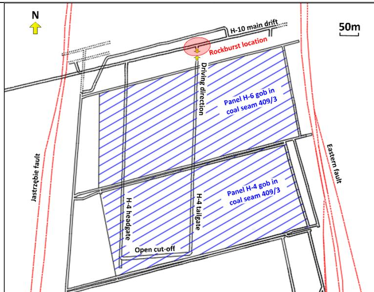
Figure 3.3 Location of the rockburst event and layout of mining works.
