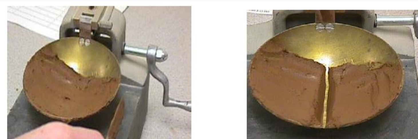
Figure 2: Liquid limit apparatus with soil - before and after cutting the groove (Pic Courtesy: ASTM 4318)
