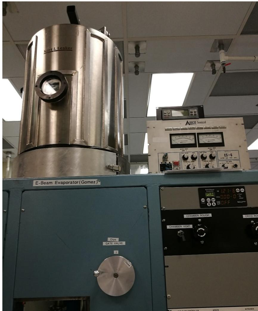
Figure 2.10 The EBPVD system used for material deposition in the experiment.
