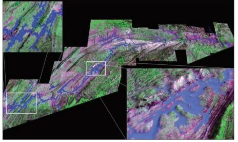
**Figure 3.** Model-generated image of the Three Gorges Reservoir Inundated Area, showing the spatial distribution of new islands, assuming that the water level is raised to 200 meters. The DEM used has 50-meter contour intervals.
