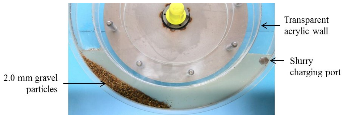
Figure 3.7. A partial view of the ATW in operation; N = 60 \text{ RPM} ; d_{50} = 2 \text{ mm} ; C_s = 10\%
