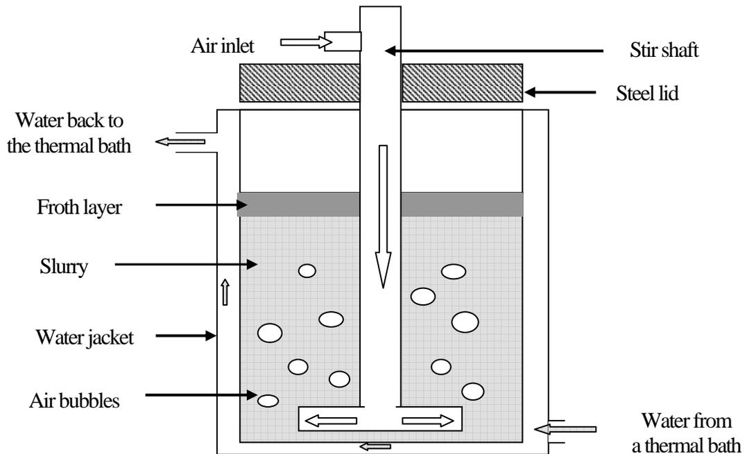
Figure 4.1 A schematic of the modified Denver flotation cell.
