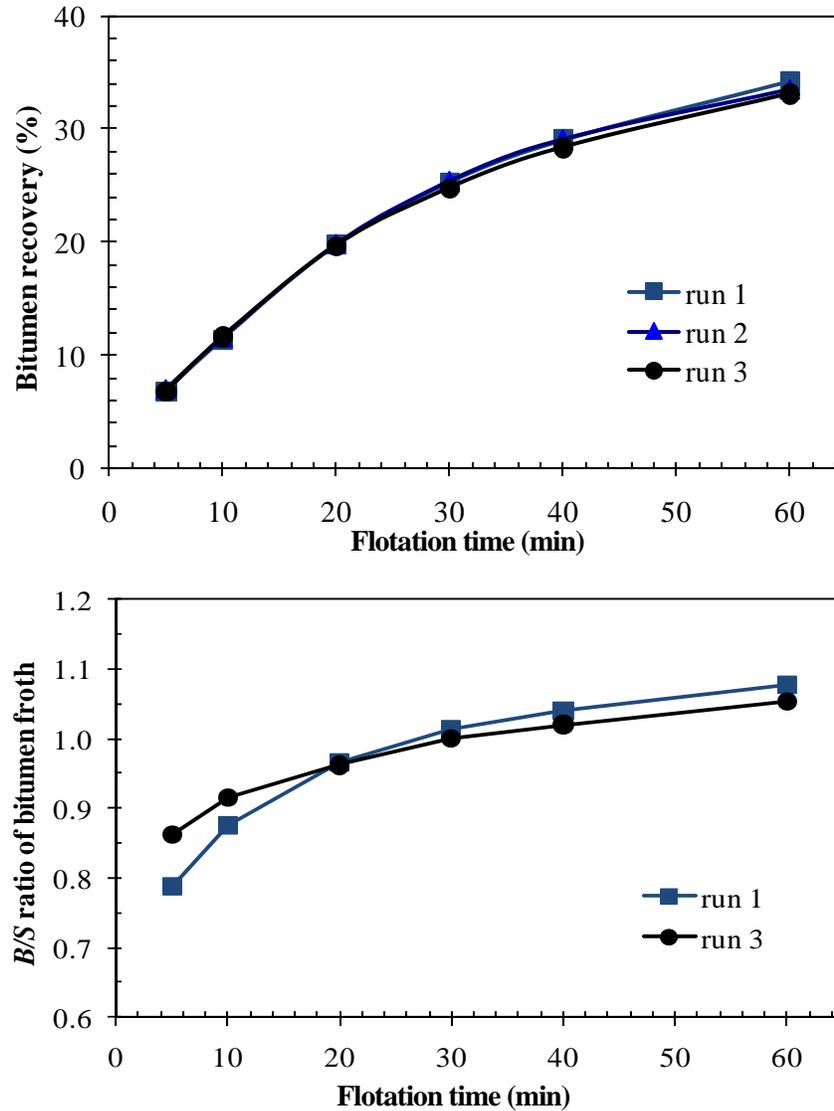
Figure D.1 Repeatability of the flotation tests on the LHES: (a) bitumen recovery and (b)  $B/S$  ratio of bitumen froth, using 1 kg Syn704 ore, 45 °C, 3 m/s, no conditioning prior to flotation at air injection rate of 200 mL/min.
