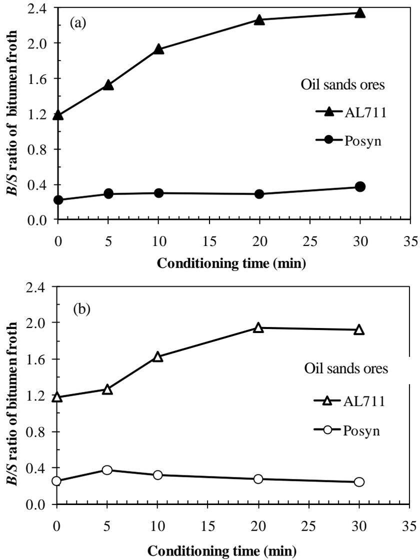
Figure G.2B Effect of conditioning time on  $B/S$  ratio of bitumen froth for good (AL711) and poor (Posyn) processing ores tested in Denver flotation cell at 45 °C and 1500 rpm with sealed cell conditioning prior to flotation at air injection rate of 75 mL/min for (a) 5 min (solid symbols) and (b) 20 min (open symbols).
