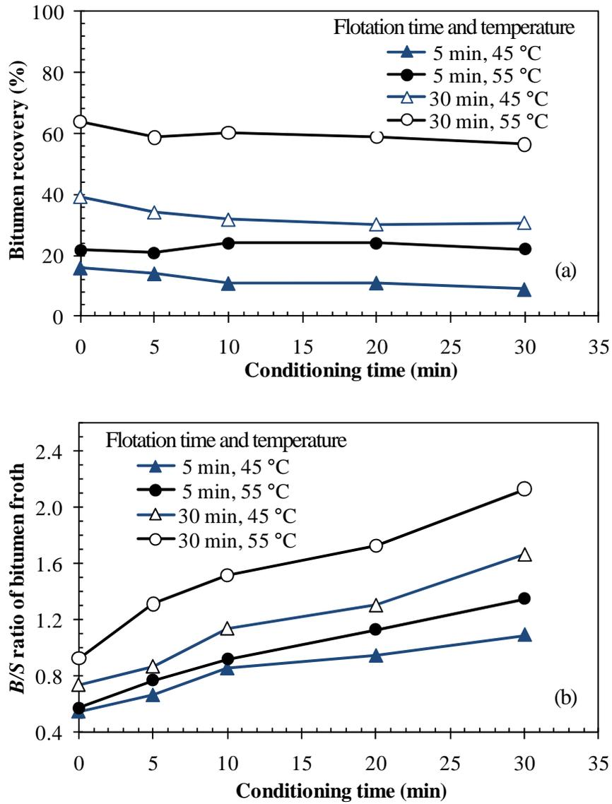
Figure 3.12 Effect of slurry temperature on (a) bitumen recovery and (b) *B/S* ratio of bitumen froth for the good processing ore (AL711) tested in the LHES, using 1 kg ore tested at 45 °C (triangles) or 55 °C (circles) and 3.0 m/s slurry flow velocity with flotation at air injection rate of 500 mL/min for 5 min (solid symbols) and 30 min (open symbols).
