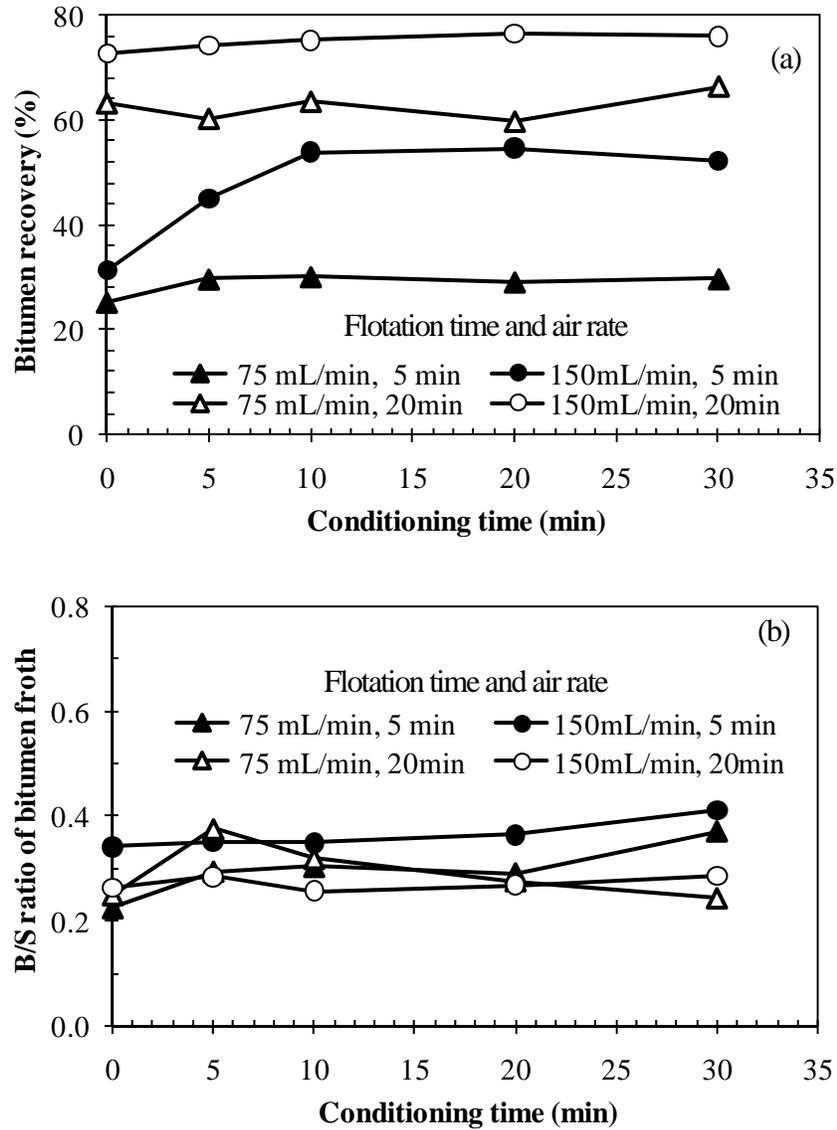
Figure 4.6 Effect of air injection rate on (a) bitumen recovery and (b)  $B/S$  ratio of bitumen froth for the poor processing ore (Posyn) extracted in Denver flotation cell, using 300 g ore tested at 45 °C and 1500 rpm with sealed cell conditioning prior to flotation at air injection rate of 75 mL/min (triangles) and 150 mL/min (circles) for 5 min (solid symbols) and 20 min (open symbols), respectively.
