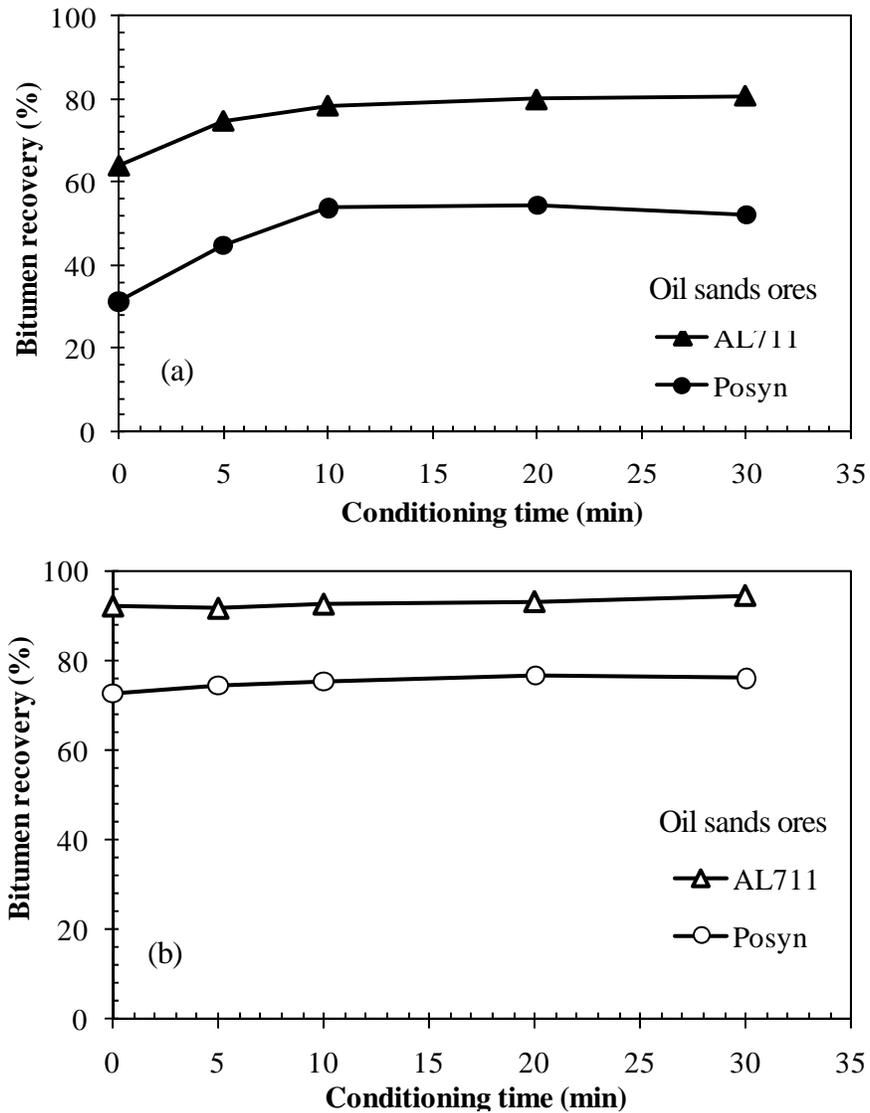
Figure G.1A Effect of conditioning time on bitumen recovery of good (AL711) and poor (Posyn) processing ores tested in Denver flotation cell at 45 °C and 1500 rpm with sealed cell conditioning prior to flotation at air injection rate of 150 mL/min for (a) 5 min (solid symbols) and (b) 20 min (open symbols).
