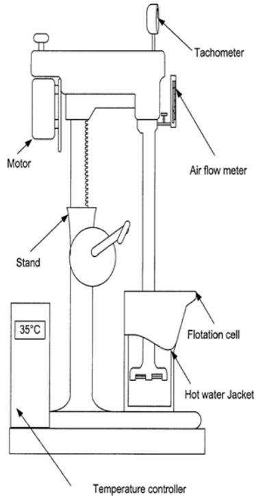
Figure 2.1 Schematic of a laboratory Denver flotation cell (Kasongo, 2000).
