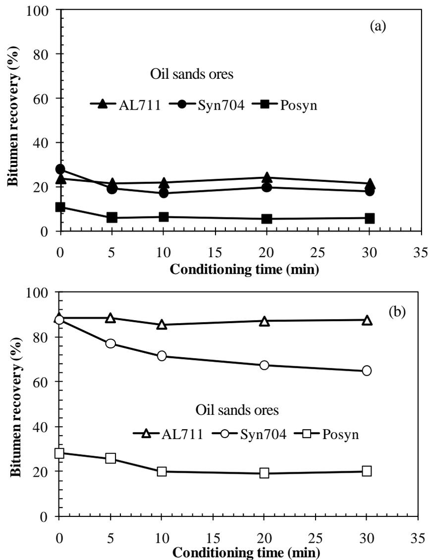
Figure E.2A Effect of conditioning time on bitumen recovery of good (AL711), transition (Syn704) and poor (Posyn) processing ores tested in the LHES at 45 °C, 4.5 m/s and 500 mL/min for flotation time of (a) 5 min (solid symbols) and (b) 30 min (open symbols).
