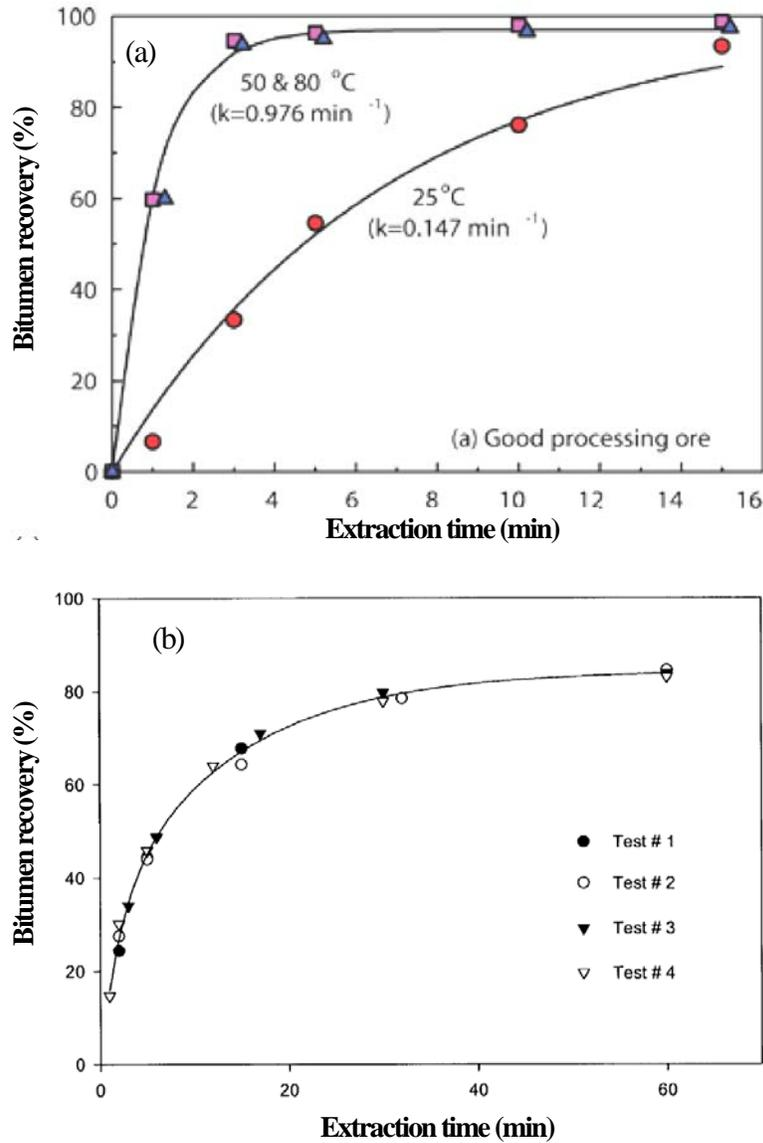
Figure 2.8 Bitumen recovery as a function of extraction time at 50 °C, using (a) a Denver flotation cell (Zhou, et al., 2004b) and (b) a LHES loop (Wallwork, et al., 2004).
