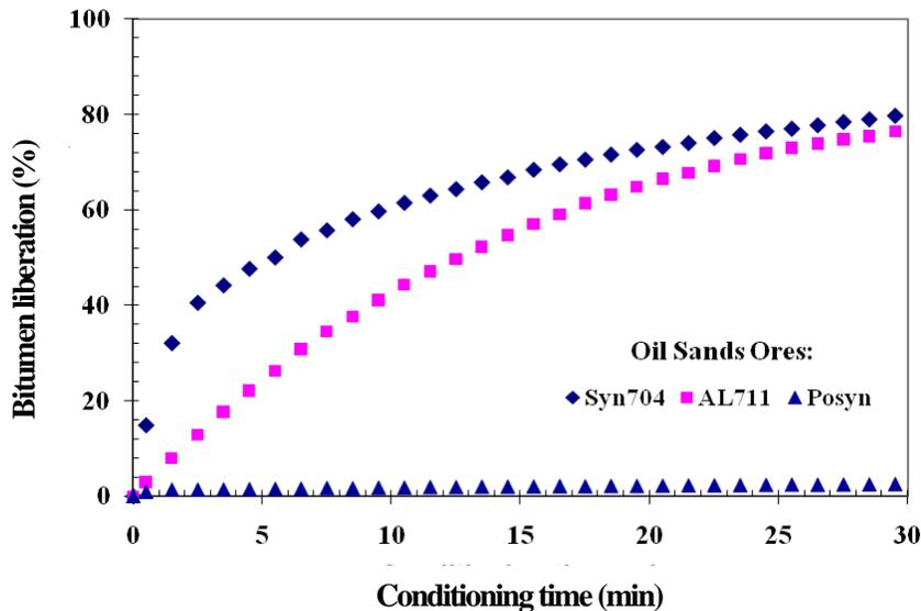
Figure 3.3 Bitumen liberation rates versa conditioning time for transition (Syn704), good (AL711) and poor (Posyn) processing ores, respectively, tested in the LHES. Experimental conditions: 45 °C and 3 m/s slurry flow velocity, no air injected (i.e., 0 min flotation time).
