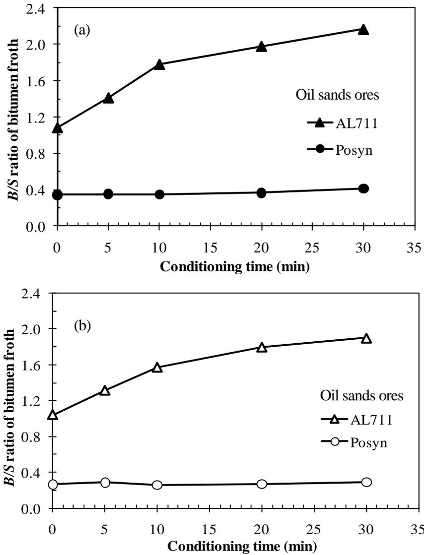
Figure G.1B Effect of conditioning time on  $B/S$  ratio of bitumen froth for good (AL711) and poor (Posyn) processing ores tested in Denver flotation cell at 45 °C and 1500 rpm with sealed cell conditioning prior to flotation at air injection rate of 150 mL/min (a) 5 min (solid symbols) and (b) 20 min (open symbols).
