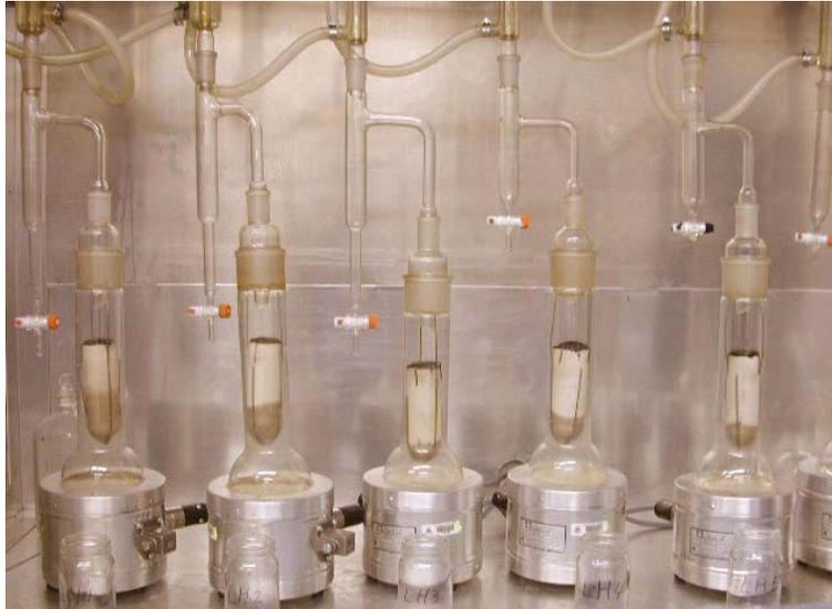
Figure B.1 Dean Stark apparatus set-up for oil/water/solids analysis (Wallwork, 2003).
