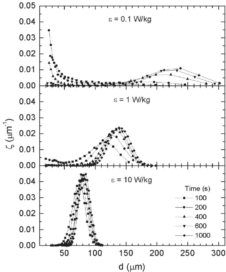
Figure 2.10 Size distribution of unaerated bitumen drops depending on the energy dissipation rate and slurring time prior to aeration, where  $\zeta$  is volumetric fraction of drops with specific diameter  $d$  ( $\mu\text{m}^{-1}$ ),  $\varepsilon$  the average turbulence strength (W/kg) (Friesen and Dabros, 2004a).
