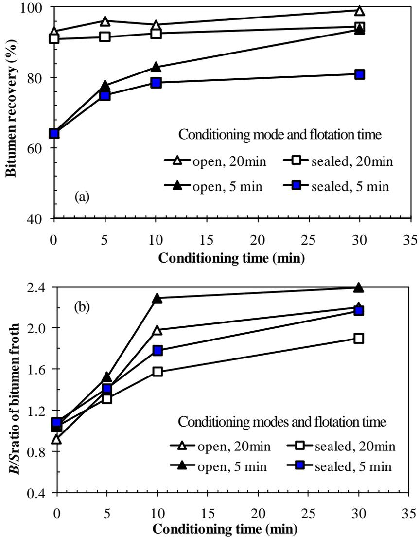
Figure 4.2 Effect of conditioning modes on (a) bitumen recovery and (b)  $B/S$  ratio of bitumen froth for the good processing ore (AL711) tested in Denver flotation cell, using 300g ore tested at 45 °C and 1500 rpm with conditioning in open cell (triangles) or sealed cell (squares), prior to flotation at air injection rate of 150 mL/min for 5 min (solid symbols) and 20 min (open symbols).
