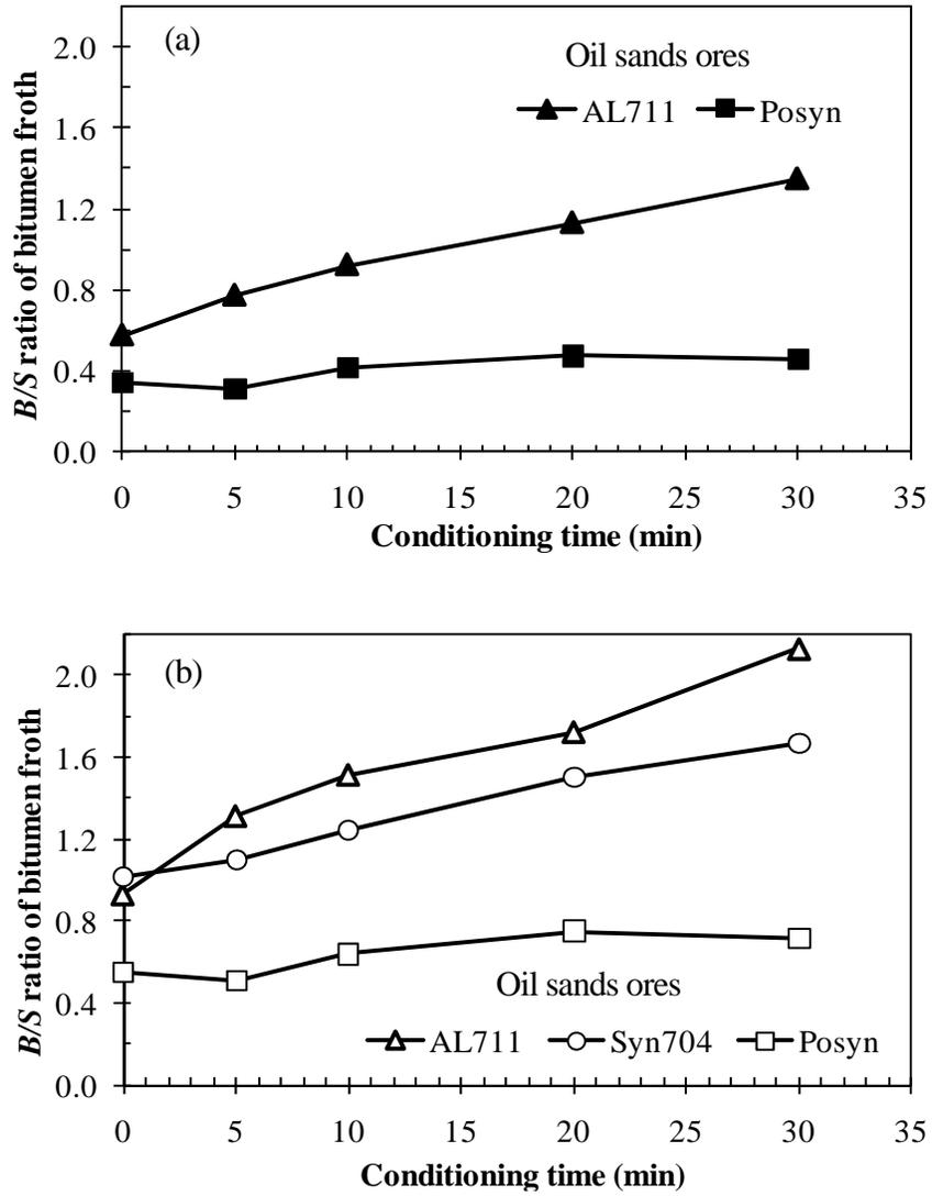
Figure E.3B Effect of conditioning time on  $B/S$  ratio of bitumen froth for good (AL711), transition (Syn704) and poor (Posyn) processing ores tested in the LHES at 55 °C, 3.0 m/s and 500 mL/min for flotation time of (a) 5 min (solid symbols) and (b) 30 min (open symbols).
