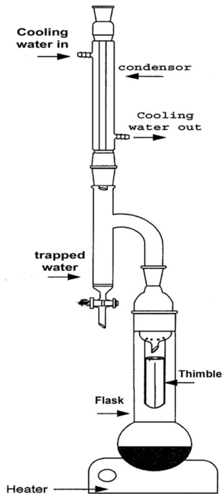
Figure 3.1 A schematic of the Dean Stark device (Bulmer, et al., 1979; Jha, 2007).
