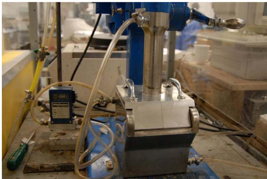
Figure F.2 Photograph of Denver flotation cell in use for slurry conditioning.
