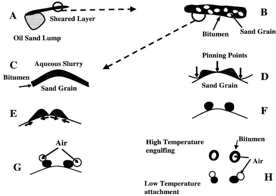
Figure 1.3 Conceptual stages for bitumen liberation and aeration (Masliyah, 2006).
