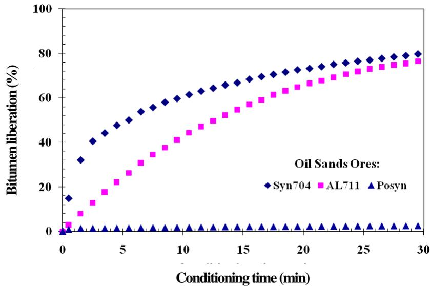
Figure 3.3 Bitumen liberation rates versus conditioning time for transition (Syn704), good (AL711) and poor (Posyn) processing ores, respectively, tested in the LHES. Experimental conditions: 45 °C and 3 m/s slurry flow velocity, no air injected (i.e., 0 min flotation time).
