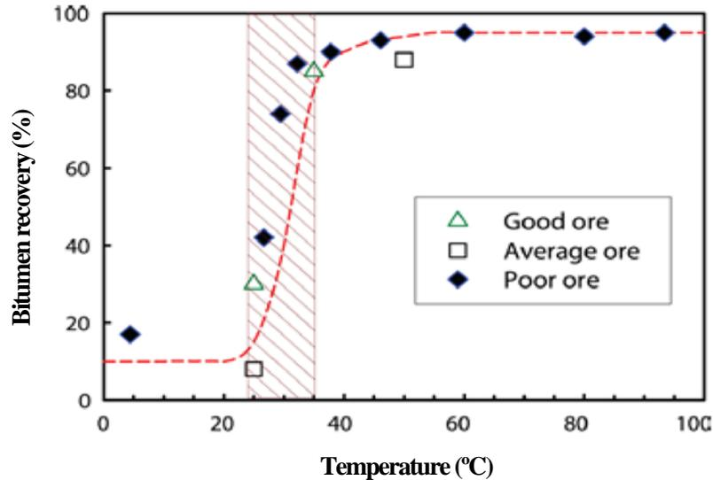
Figure 2.4 Effect of processing temperature on bitumen recovery in bench scale tests (Long, et al. 2007).
