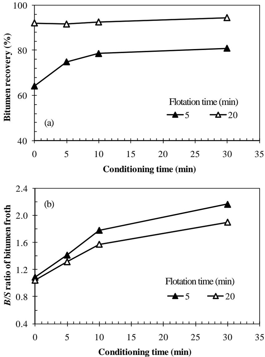
Figure 4.3 Effect of conditioning time on (a) bitumen recovery and (b) *B/S* ratio of bitumen froth for the good processing ore (AL711) tested in Denver flotation cell, using 300 g ore tested at 45 °C and 1500 rpm and with sealed cell conditioning prior to air addition at 150 mL/min for 5 min (solid triangles) or 20 min (open triangles).
