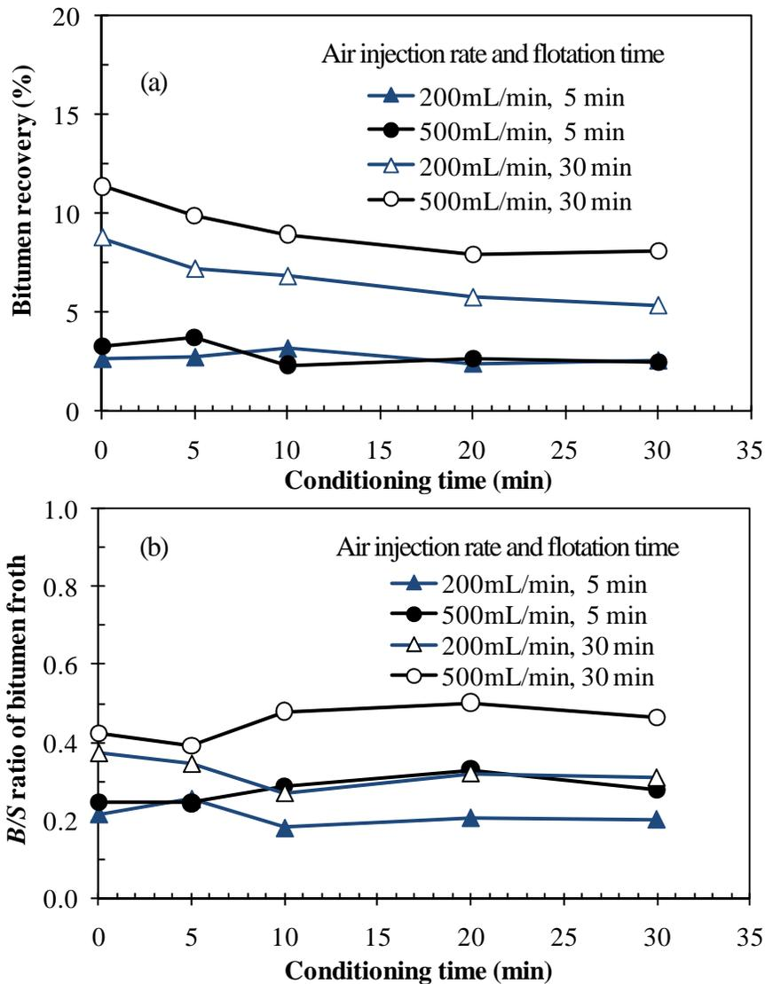
Figure 3.9 Effect of air injection rate on (a) bitumen recovery and (b) *B/S* ratio of bitumen froth using 1 kg poor processing ore (Posyn) tested in the LHES. Experimental conditions: at 45 °C and 3.0 m/s with slurry conditioning prior to flotation for flotation time of 5 min (solid symbols) and 30 min (open symbols) at 200 mL/min (triangles) or 500 mL/min (circles).
