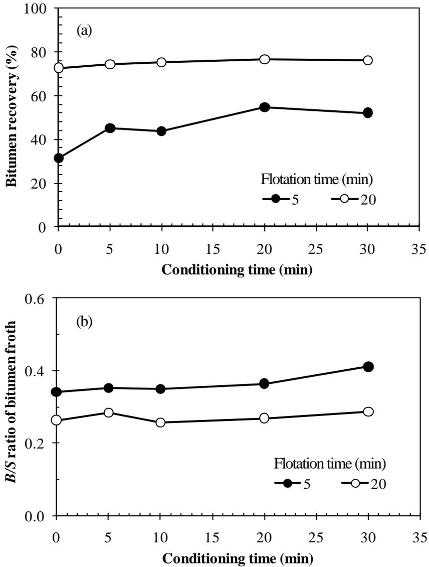
Figure 4.4 Effect of conditioning time on (a) bitumen recovery and (b)  $B/S$  ratio of bitumen froth, for the poor processing ore (Posyn) tested in Denver flotation cell, using 300 g ore tested at 45 °C and 1500 rpm and with conditioning in sealed cell prior to flotation at air injection rate of 150 mL/min for 5 min (solid circles) and 20 min (open circles), respectively.
