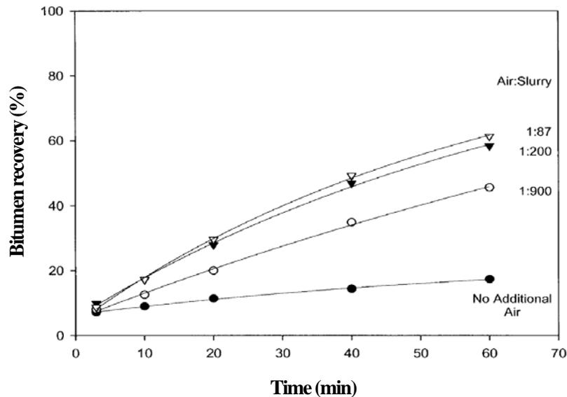
Figure 2.6 Effect of air injection on bitumen recovery of high fines ore, extracted at 35 °C using the LHES loop (Wallwork, et al., 2004).
