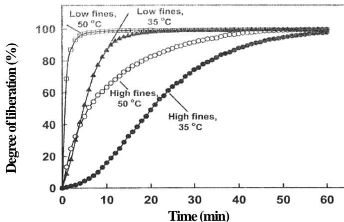
Figure 2.7 Effect of temperature and fines content on bitumen liberation from sand grains (Wallwork,
