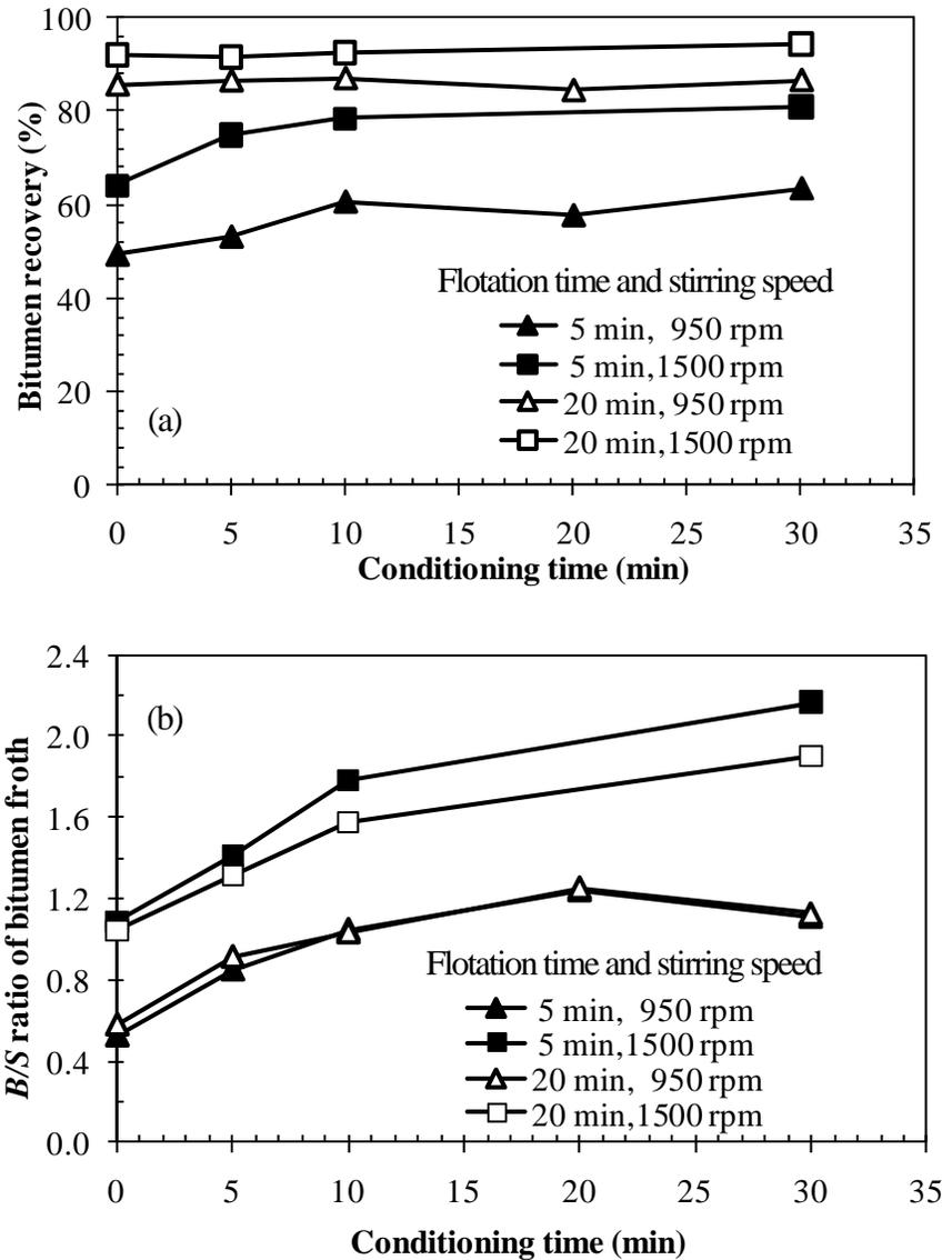
Figure 4.7 Effect of stirring speed on (a) bitumen recovery and (b) *B/S* ratio of bitumen froth for the good processing ore (AL711) tested in Denver flotation cell, using 300 g ore tested at 45 °C and 950 rpm (triangles) and 1500 rpm (circles) with sealed cell conditioning prior to flotation at air injection rate of 150 mL/min for 5 min (solid symbols) and 20 min (open symbols).
