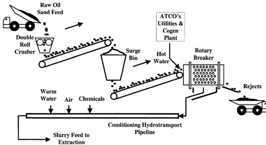
Figure 2.3 Ore preparation and slurry conditioning (cited by Masliyah, et al., 2004).
