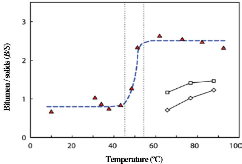
Figure 2.5 Effect of temperature on bitumen froth quality measured by bitumen to solids mass ratio ( $B/S$ ) (Bichard, 1987). The filled triangles represent a poor processing ore.
