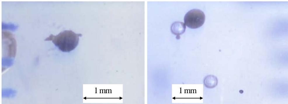
Figure 3.14 Microphotographs of bubbles/aggregates rising in the Luba tube at 1 min flotation time in the LHES using 1 kg AL711 ore tested at 45 °C (left) and 55 °C (right) with 30 min conditioning time, 4.5 m/s slurry flow velocity and 500 mL/min air injection rate.
