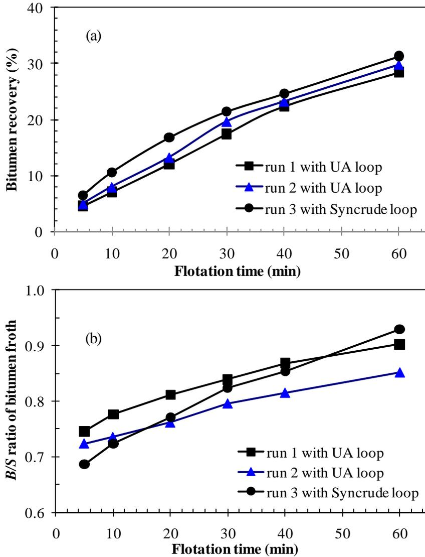
Figure 3.2 Repeatability test of the LHES: (a) bitumen recovery and (b)  $B/S$  ratio of bitumen froth, using 1 kg transition ore (Syn704) at temperature of 35 °C, air injection rate of 200 mL/min, slurry flow velocity of 3 m/s and conditioning for 5 minutes.
