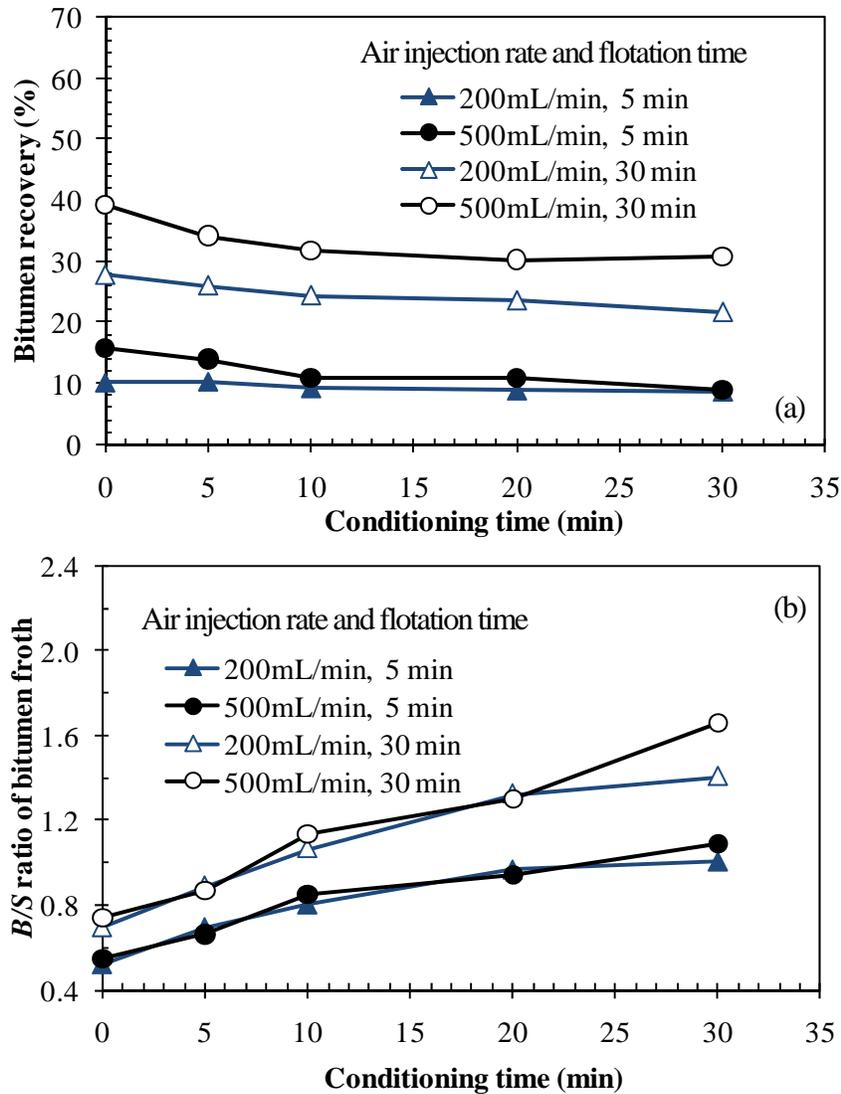
Figure 3.8 Effect of air injection rate on (a) bitumen recovery and (b) *B/S* ratio of bitumen froth for good processing ore (AL711) tested in the LHES. Experimental conditions: 1 kg ore tested at 45 °C and 3.0 m/s with slurry conditioning prior to flotation at air rate of 200 m L/min (triangles) and 500 m L/min (circles) for flotation time of 5 min (solid symbols) and 30 min (open symbols).
