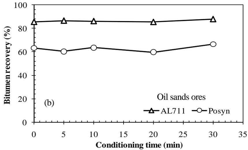
Figure G.2A Effect of conditioning time on bitumen recovery of good (AL711) and poor processing (Posyn) ores tested in Denver flotation cell at 45 °C and 1500 rpm with sealed cell conditioning prior to flotation at air injection rate of 75 mL/min (a) 5 min (solid symbols) and (b) 20 min (open symbols).
