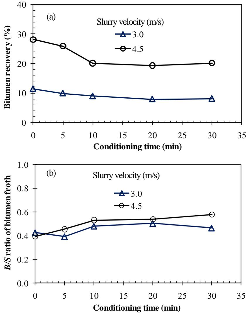
Figure 3.17 Effect of slurry velocity on (a) bitumen recovery and (b) *B/S* ratio of bitumen froth for the poor processing ore (Posyn) tested in the LHES. Experimental conditions: 1 kg ore tested at 45 °C, 3.0 m/s (triangles) or 4.5 m/s (circles) slurry flow velocity and air injection rate 500 mL/min for 30 min.
