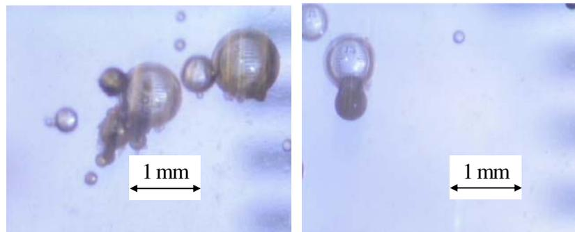
Figure 3.6 Microphotographs of the bubbles/aggregates rising in the Luba tube at air injection, using 1 kg AL711 ore tested at 55 °C and 4.5 m/s slurry flow velocity in the LHES. The slurry was conditioned for 0 min (left) and 30 min (right) prior to flotation at air injection rate of 500 mL/min.
