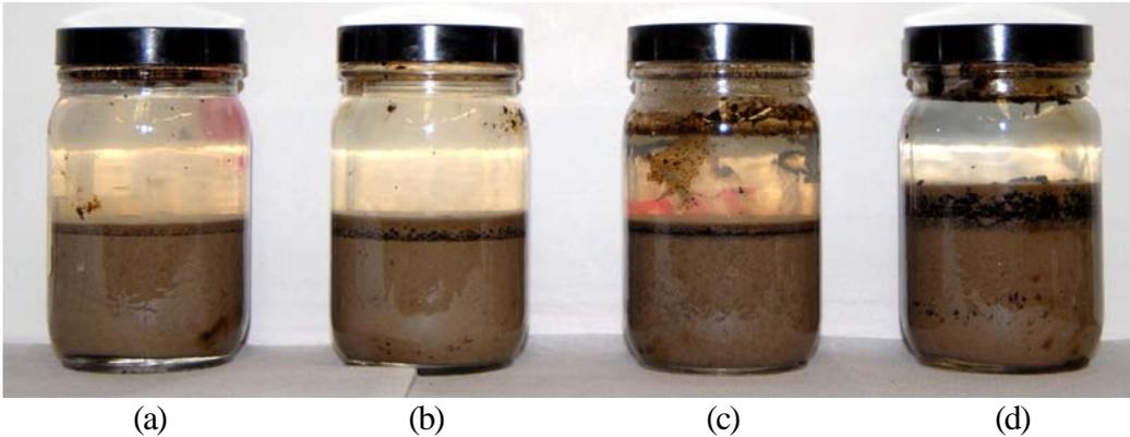
Figure 3.5 Photographs of tailings for tests with conditioning time of (a) 0 min, (b) 5 min, (c) 10 min and (d) 30 min, using 1 kg transition ore (Syn704) at 45 °C, 3.0 m/s slurry flow velocity and 60 min flotation time at 200 mL/min air injection rate in the LHES.
