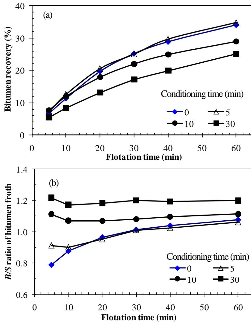
Figure 3.4 Effect of slurry conditioning time on (a) bitumen recovery and (b) *B/S* ratio of bitumen froth for the transition ore (Syn704) tested in the LHES, using 1 kg ore tested at 45 °C, 200 mL/min air
