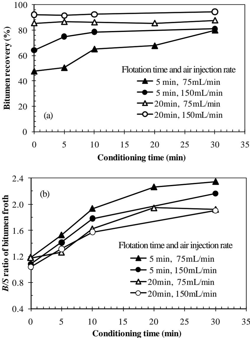
Figure 4.5 Effect of air injection rate on (a) bitumen recovery and (b) *B/S* ratio of bitumen froth for the good processing ore (AL711) tested in Denver flotation cell, using 300 g ore tested at 45 °C and 1500 rpm with sealed cell conditioning prior to flotation at air injection rate of 75 mL/min (triangles) and 150 mL/min (circles) for 5 min (solid symbols) and 20 min (open symbols), respectively.
