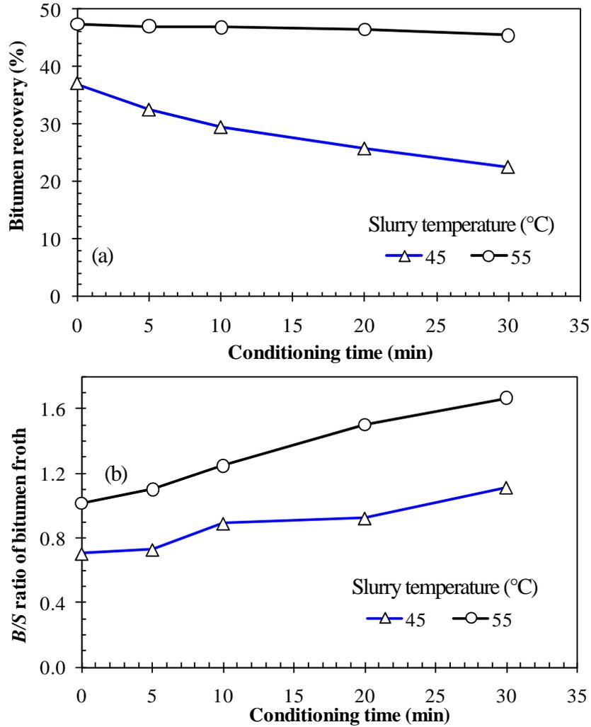
Figure 3.11 Effect of slurry temperature on (a) bitumen recovery and (b)  $B/S$  ratio of bitumen froth for the transition ore (Syn704) tested in the LHES, using 1 kg ore tested at 45 °C (triangles) or 55 °C (circles), 3.0 m/s slurry velocity and with 30 min flotation time at 500 mL/min.
