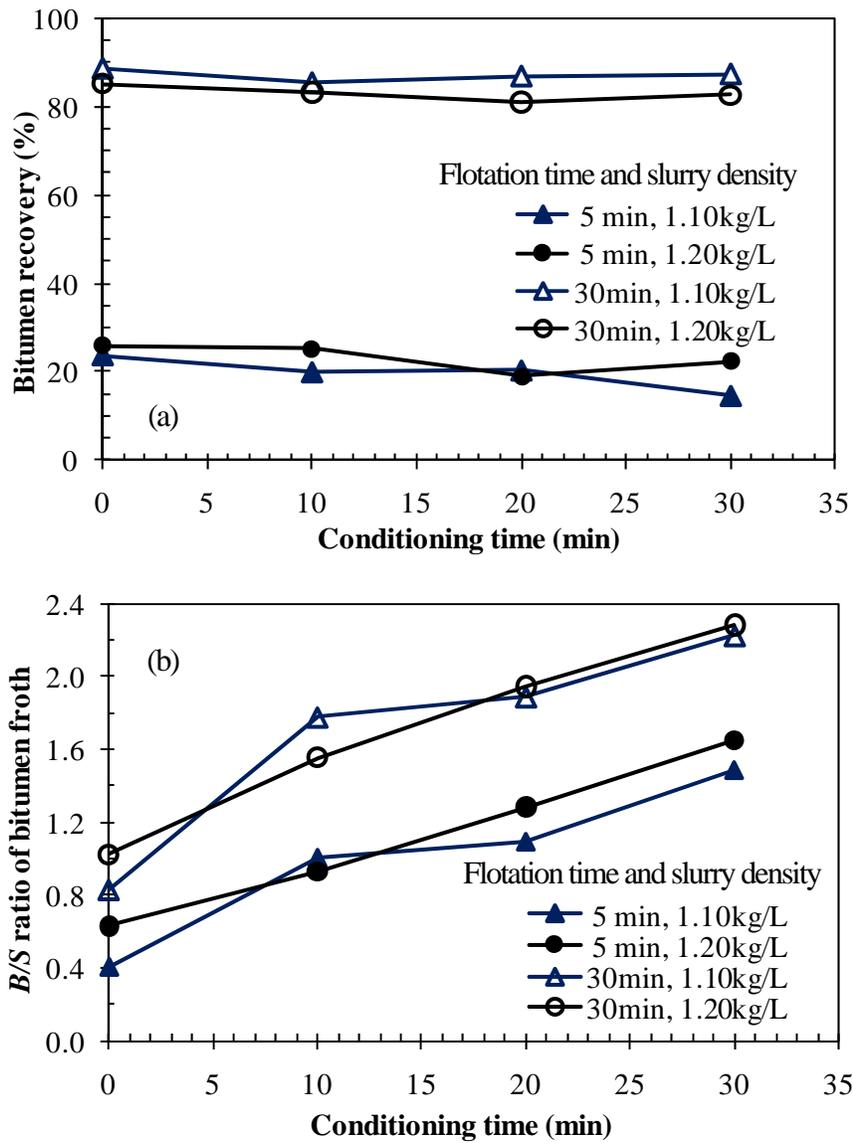
Figure 3.18 Effect of slurry density on (a) bitumen recovery and (b) *B/S* ratio of bitumen froth for the good processing ore (AL711) tested in the LHES. Experimental conditions: 1.10 kg/L (triangles) and 1.20 kg/L (circles) slurry densities, at 45 °C, 4.5 m/s slurry velocity and air injection rate 500 mL/min for 5 min (solid symbols) and 30 min (open symbols).
