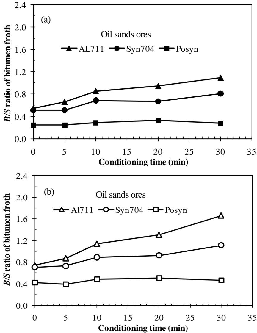
Figure E.1B Effect of conditioning time on  $B/S$  ratio of bitumen froth for good (AL711), transition (Syn704) and poor (Posyn) processing ores tested in the LHES at 45 °C, 3.0 m/s and 500 mL/min for flotation time of (a) 5 min (solid symbols) and (b) 30 min (open symbols).
