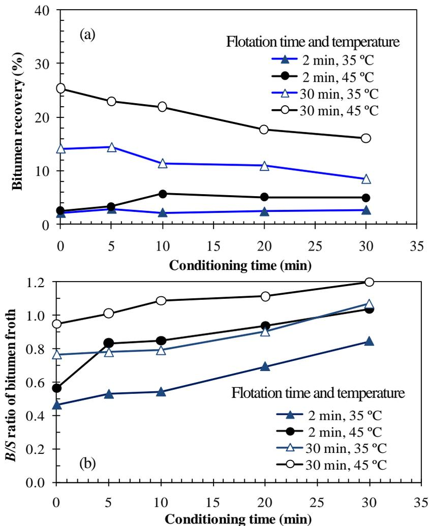
Figure 3.10 Effect of slurry temperature on (a) bitumen recovery and (b) *B/S* ratio of bitumen froth for transition ore (Syn704) tested in the LHES, using 1 kg ore tested at 35 °C (triangles) or 45 °C (circles) and 3.0 m/s with air injection rate 200 mL/min for 2 min (solid symbols) and 30 min (open symbols).
