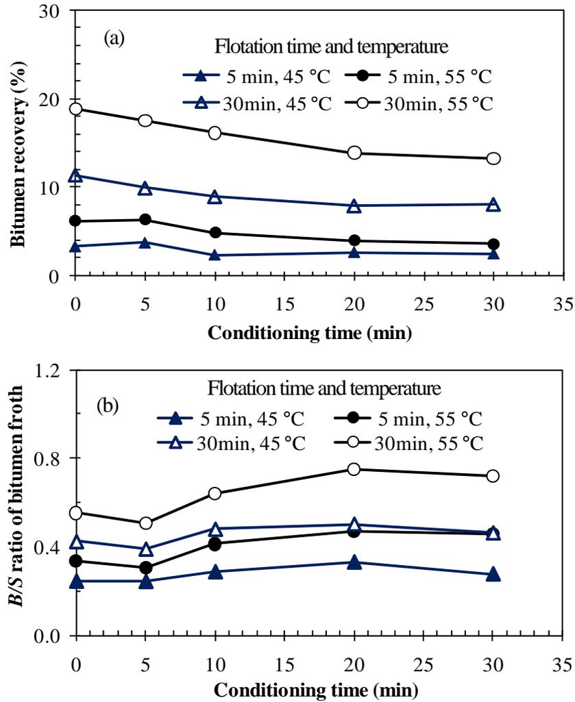
Figure 3.13 Effect of slurry temperature on (a) bitumen recovery and (b) *B/S* ratio of bitumen froth for the poor processing ore (Posyn) tested in the LHES. Experimental conditions: 1 kg ore tested at 45 °C (triangles) or 55 °C (circles) and 3.0 m/s slurry flow velocity with air injection at 500 mL/min for 5 min (solid symbols) and 30 min (open symbols).
