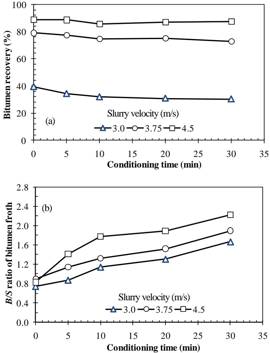
Figure 3.16 Effect of slurry velocity on (a) bitumen recovery and (b)  $B/S$  ratio of bitumen froth for the good processing ore (AL711) tested in the LHES, using 1 kg ore tested at 45 °C and 3.0 m/s (triangles), 3.75 m/s (circles) or 4.5 m/s (squares) slurry flow velocity and with 500 mL/min air injection for 30 min.
