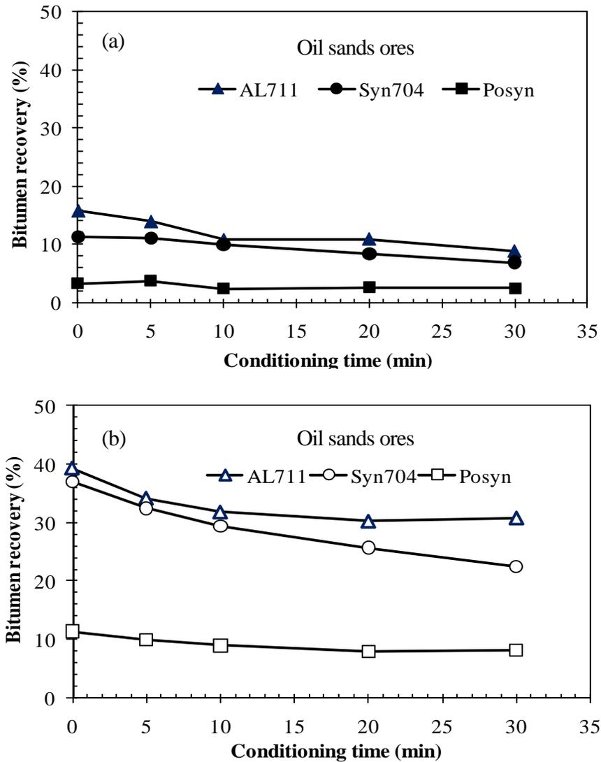
Figure E.1A Effect of conditioning time on bitumen recovery of good (AL711), transition (Syn704) and poor (Posyn) processing ores tested in the LHES at 45 °C, 3.0 m/s and 500 mL/min for flotation time of (a) 5 min (solid symbols) and (b) 30 min (open symbols).
