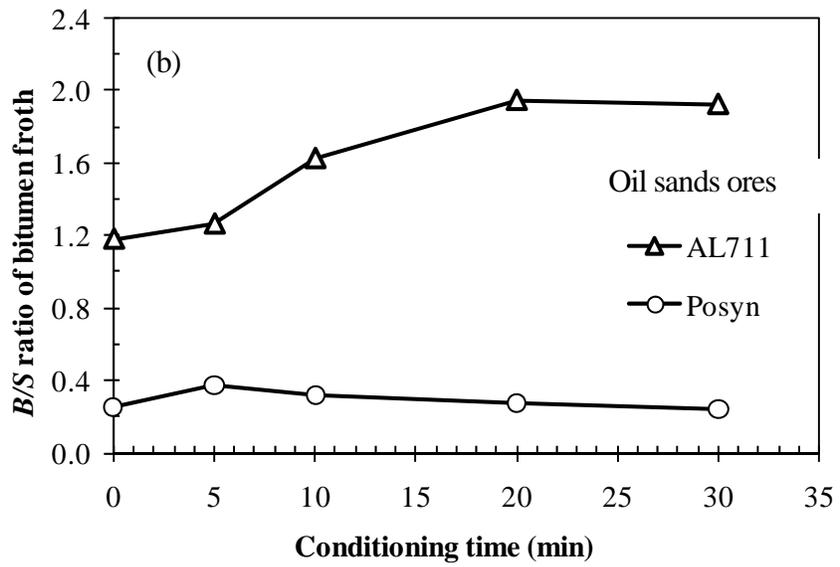
Figure G.2B Effect of conditioning time on *B/S* ratio of bitumen froth for good (AL711) and poor (Posyn) processing ores tested in Denver flotation cell at 45 °C and 1500 rpm with sealed cell conditioning prior to flotation at air injection rate of 75 mL/min for (a) 5 min (solid symbols) and (b) 20 min (open symbols).
