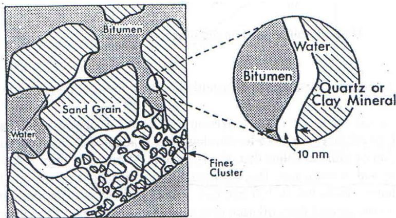
Figure 1.1 A refined schematic structure model of Athabasca oil sands (Takamura, 1982).
