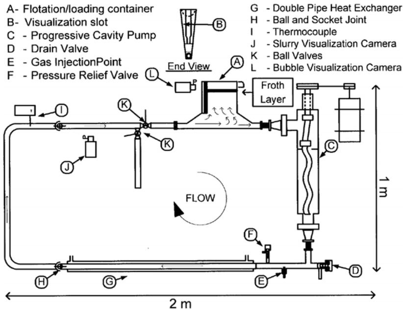
Figure 2.2 Schematic of the laboratory hydrotransport extraction system (LHES) (Wallwork, 2003).
