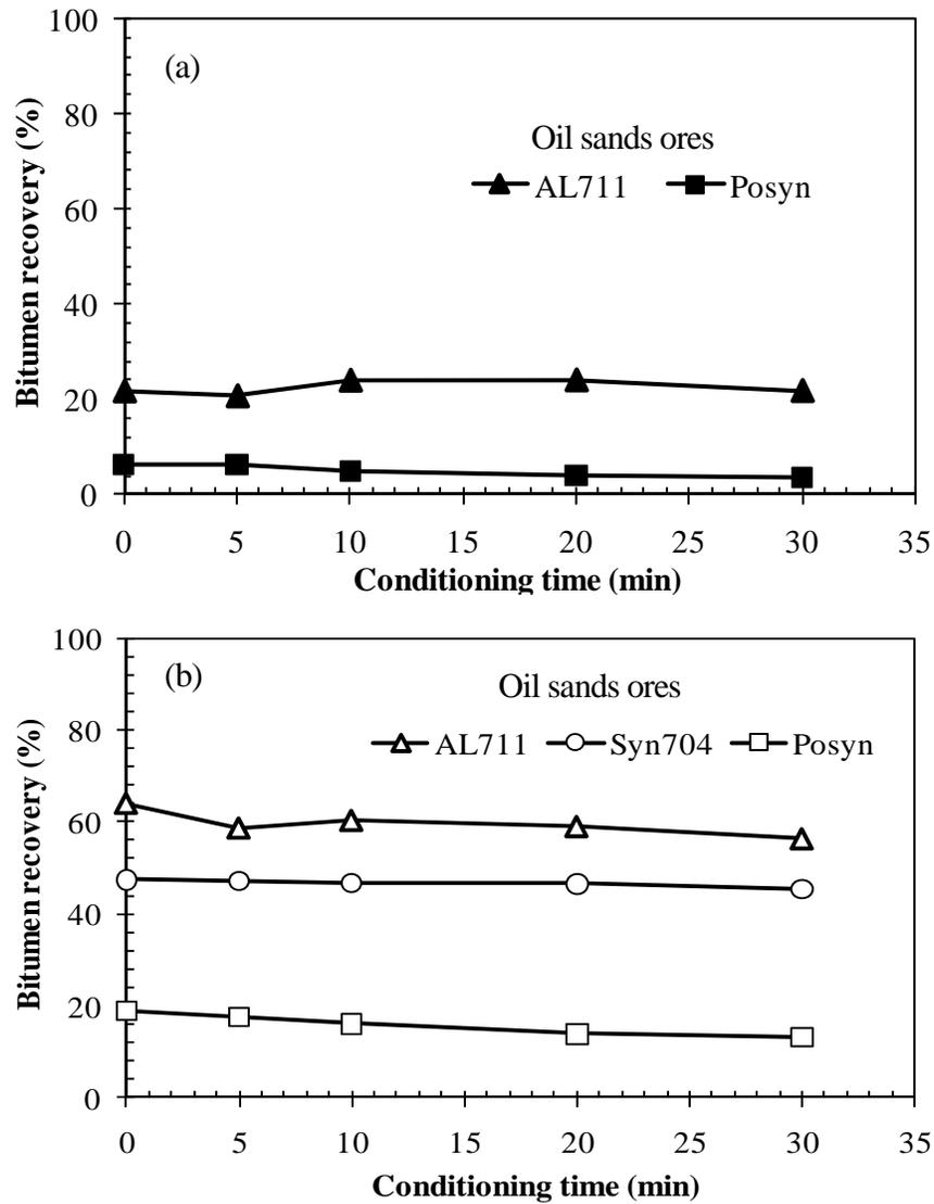
Figure E.3A Effect of conditioning time on bitumen recovery of good (AL711), transition (Syn704) and poor (Posyn) processing ores tested in the LHES at 55 °C, 3.0 m/s and 500 mL/min for flotation time of (a) 5 min (solid symbols) and (b) 30 min (open symbols).
