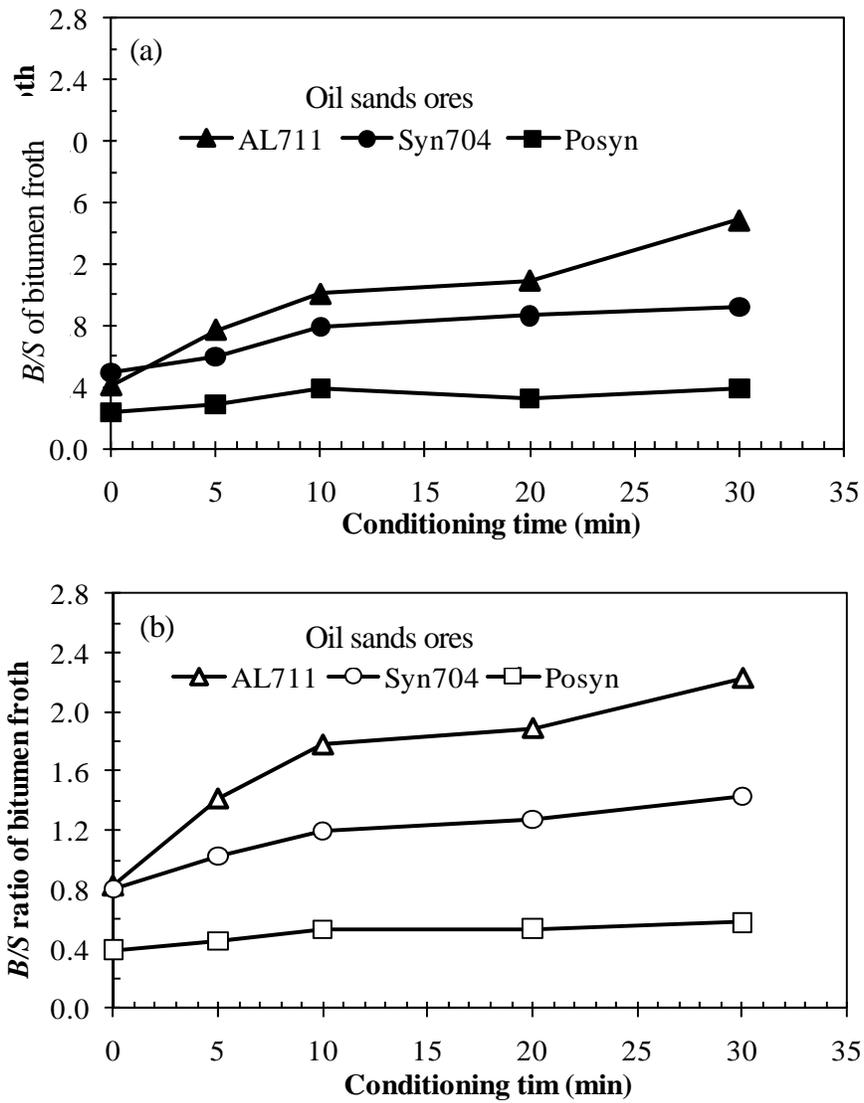
Figure E.2B Effect of conditioning time on  $B/S$  ratio of bitumen froth for good (AL711), transition (Syn704) and poor (Posyn) processing ores tested in the LHES at 45 °C, 4.5 m/s and 500 mL/min for flotation time of (a) 5 min (solid symbols) and (b) 30 min (open symbols).
