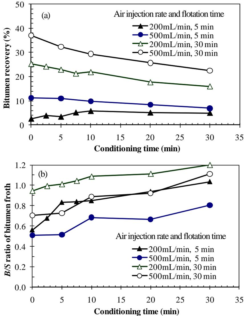
Figure 3.7 Effect of air injection rate on (a) bitumen recovery and (b) *B/S* ratio of bitumen froth for the transition ore (Syn704) tested in the LHES. Experimental conditions: 1 kg ore tested at 45 °C and 3.0 m/s slurry flow velocity with slurry conditioning prior to flotation for 5 min (solid symbols) and 30 min (open symbols) at an air injection rate of 200 mL/min (triangles) or 500 mL/min (circles).
