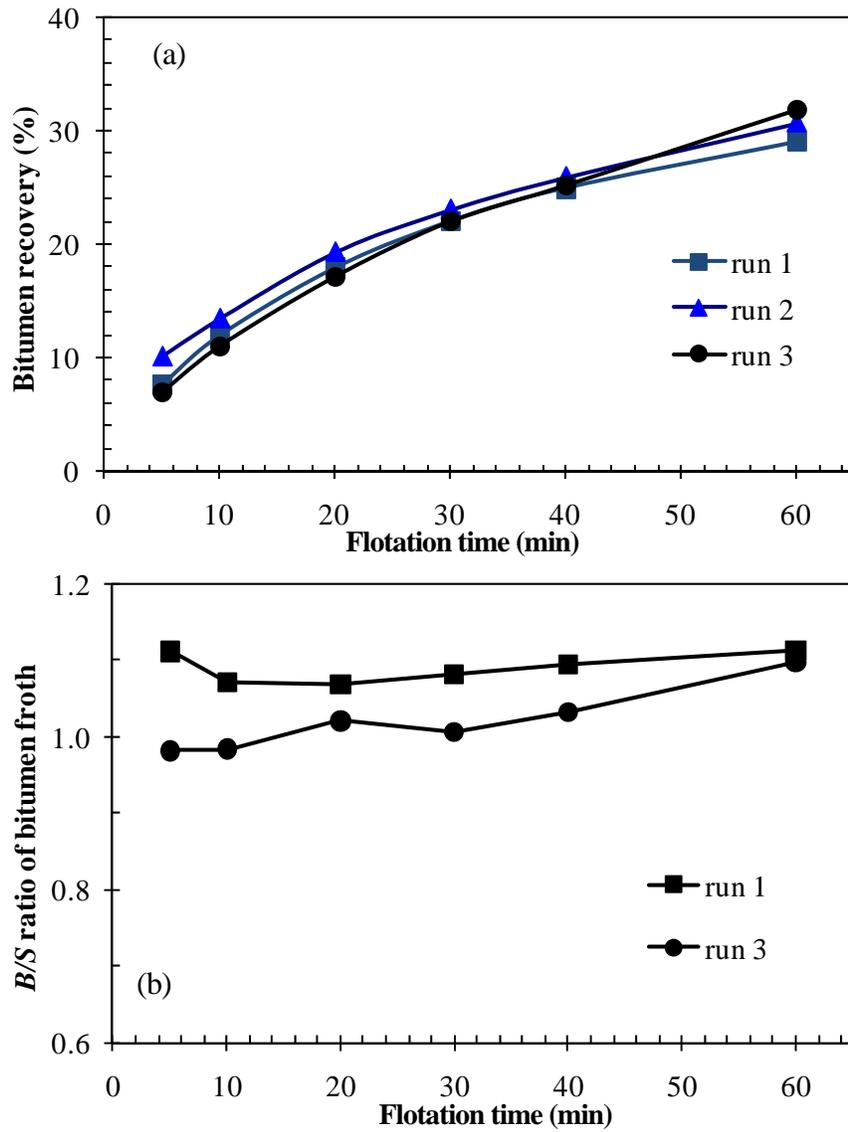
Figure D.2 Repeatability of the flotation tests on the LHES: (a) bitumen recovery and (b) *B/S* ratio of bitumen froth, using 1 kg Syn704 ore, 45 °C, 3.0 m/s, closed conditioning for 10 min prior to flotation at air injection rate of 200 mL/min.
