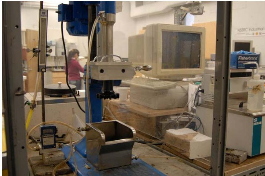
Figure F.1 Photograph of Denver flotation cell set-up.
