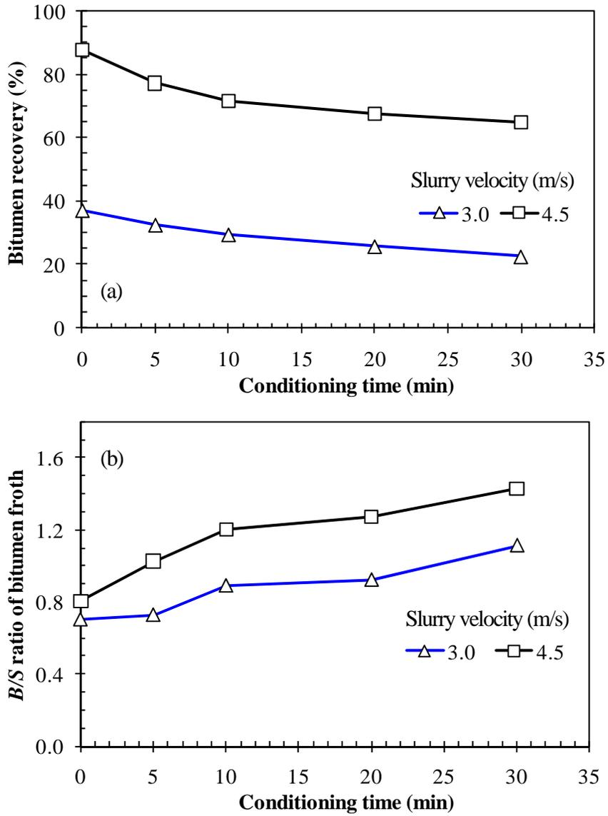
Figure 3.15 Effect of slurry velocity on (a) bitumen recovery and (b)  $B/S$  ratio of bitumen froth for the transition ore (Syn704) tested in the LHES. Experimental conditions: 1 kg ore tested at 45 °C and 3.0 m/s (triangles) or 4.5 m/s (squares) slurry flow velocity with air injection for 30 min at 500 mL/min.
