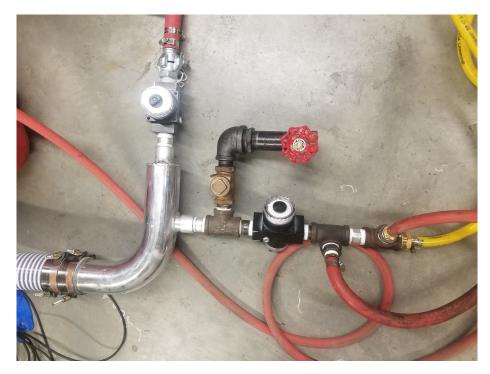
Figure 3.7: Image of the intake collector where building air is regulated to engine intake pressure.
