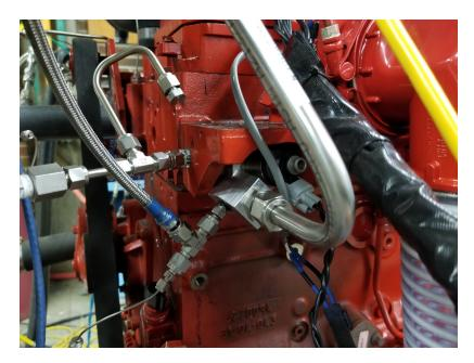
Figure 3.3: Image of the populated holes bored into the head for intake port temperature monitoring and hydrogen injector installation with mounted items.
