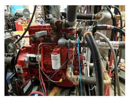
Figure 3.2: Image of the exhaust side of the tested engine.
