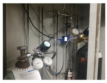
Figure 3.8: Image of the hydrogen gas cabinet.
