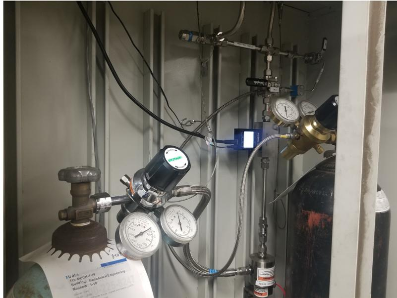
Figure 3.8: Image of the hydrogen gas cabinet.
