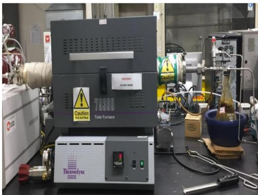
Figure 3.6: Thermolyne 79300 tube furnace
