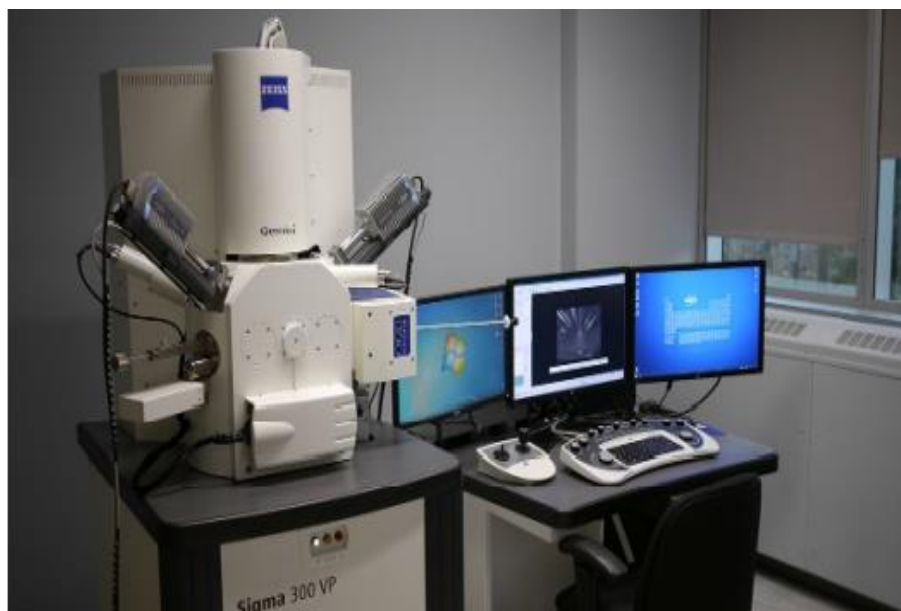
Figure 3.7: Zeiss Sigma 300 VP-FESEM
