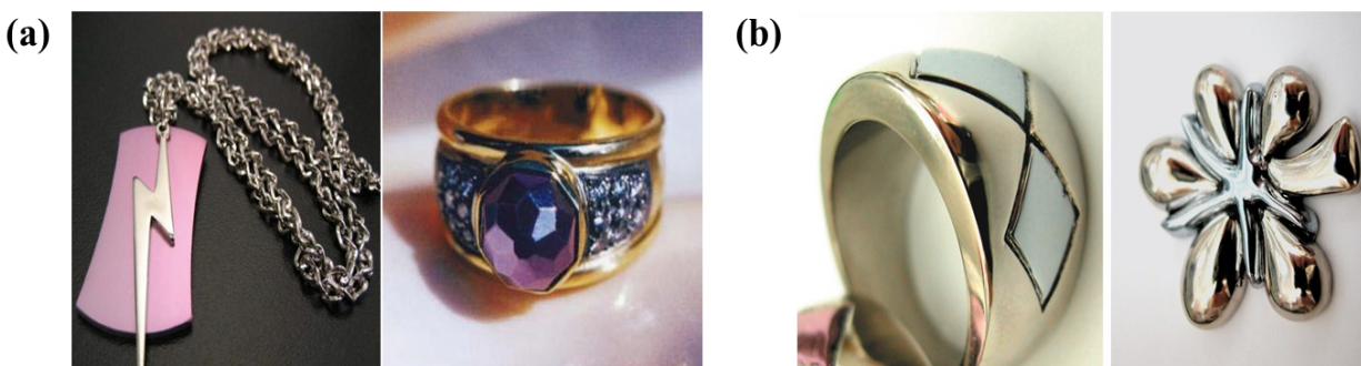
Figure 1-1. Jewellery items produced by (a) purple gold \text{AuAl}_2 and (b) blue gold \text{AuGa}_2 coating.
