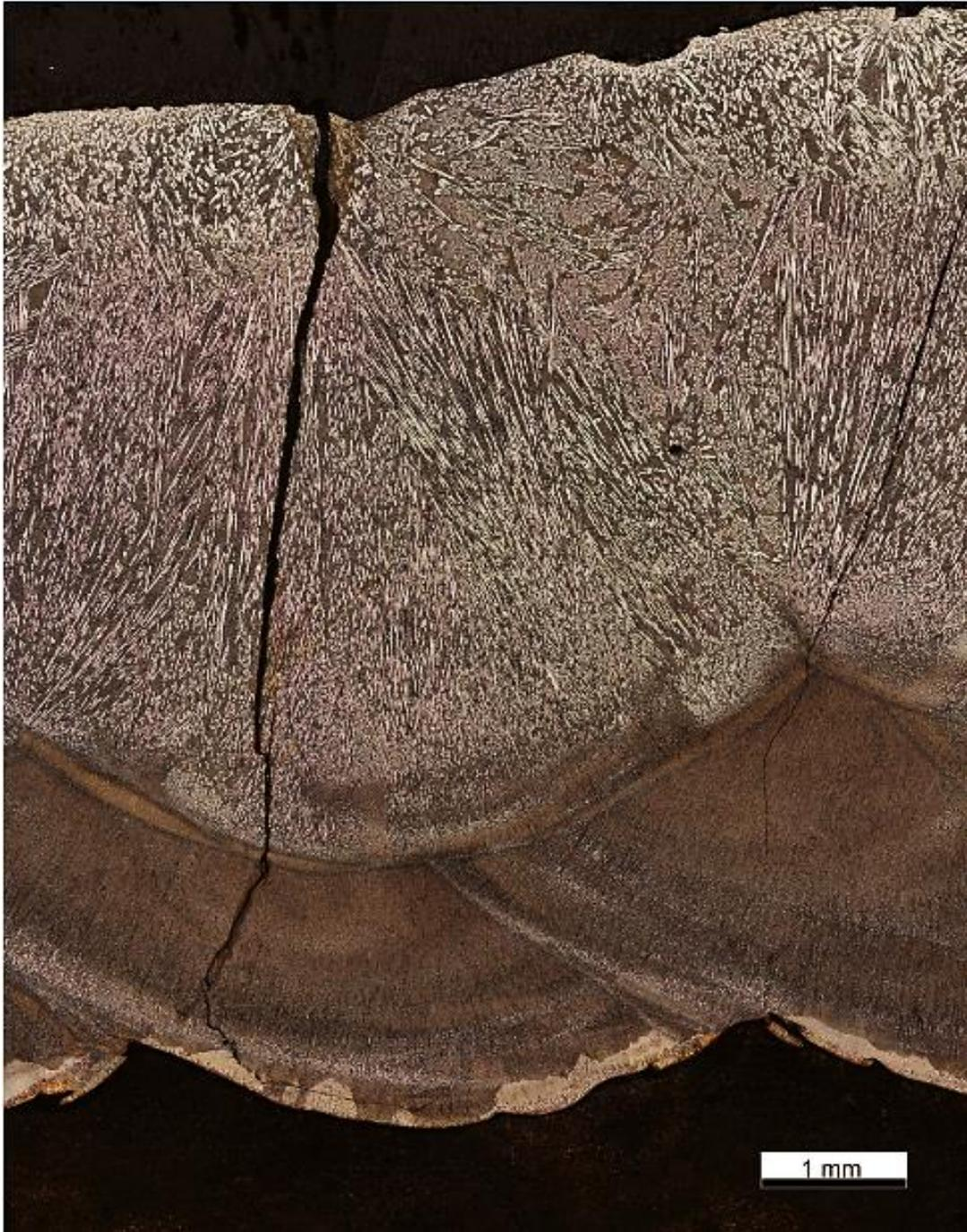
**Figure 7-6: GMAW overall micrograph of CCO-1**
