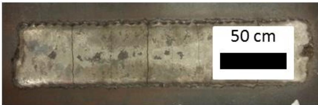
**Figure 7-4: Weld appearance of SAW 100C CCO**
