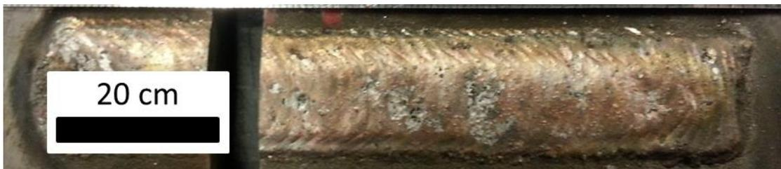
**Figure 7-3: Weld bead appearance of single pass PTAW CCO at 180 A**
