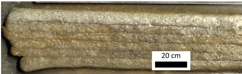
Figure 7-1 Weld bead appearance of double-layered GMAW chromium carbide overlay GMAW1
