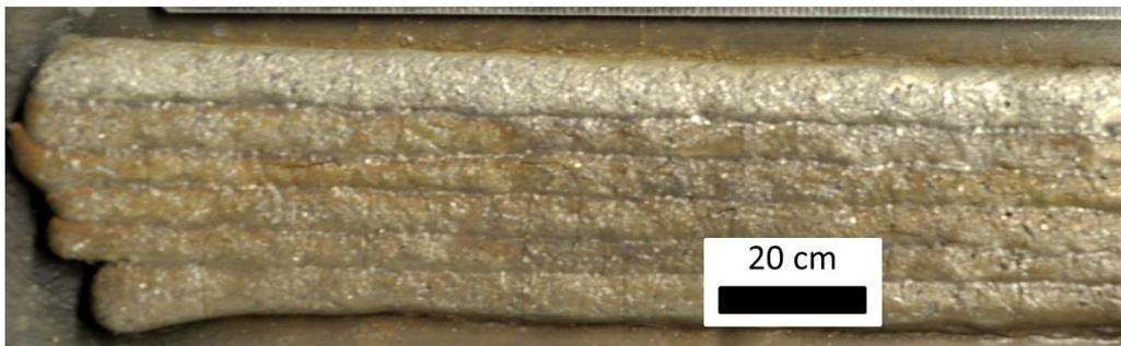
Figure 7-1 Weld bead appearance of double-layered GMAW chromium carbide overlay GMAW1
