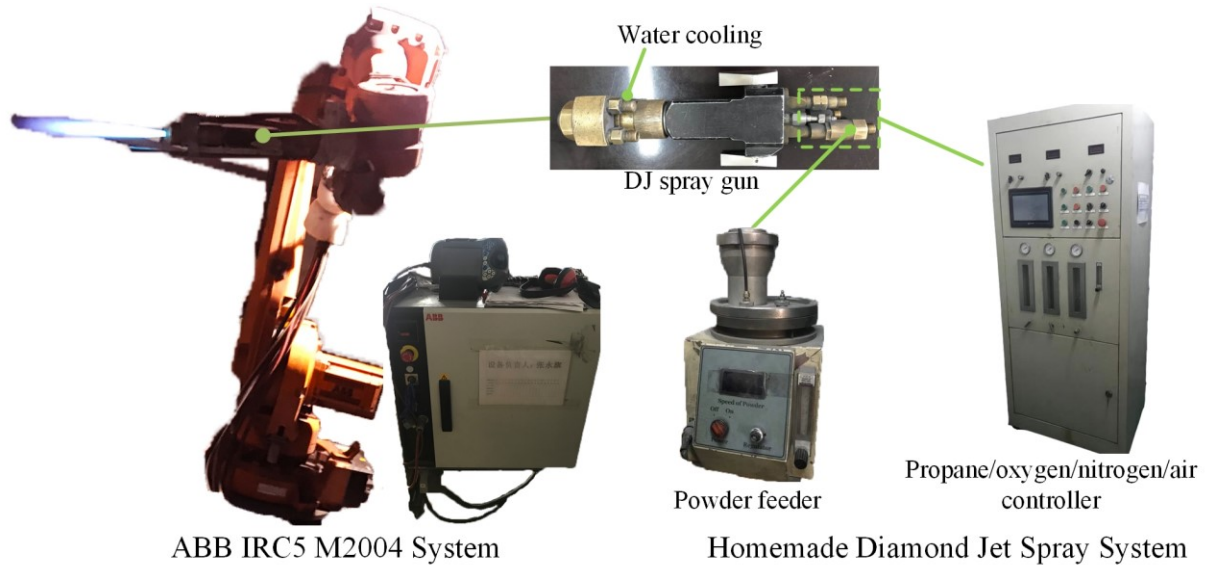
Figure 4.5 A homemade Diamond Jet spray system.
