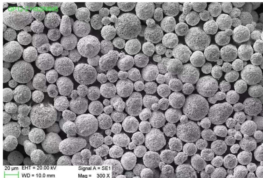
Figure 5.3 SEM image of the WC-12Co powder particles.
