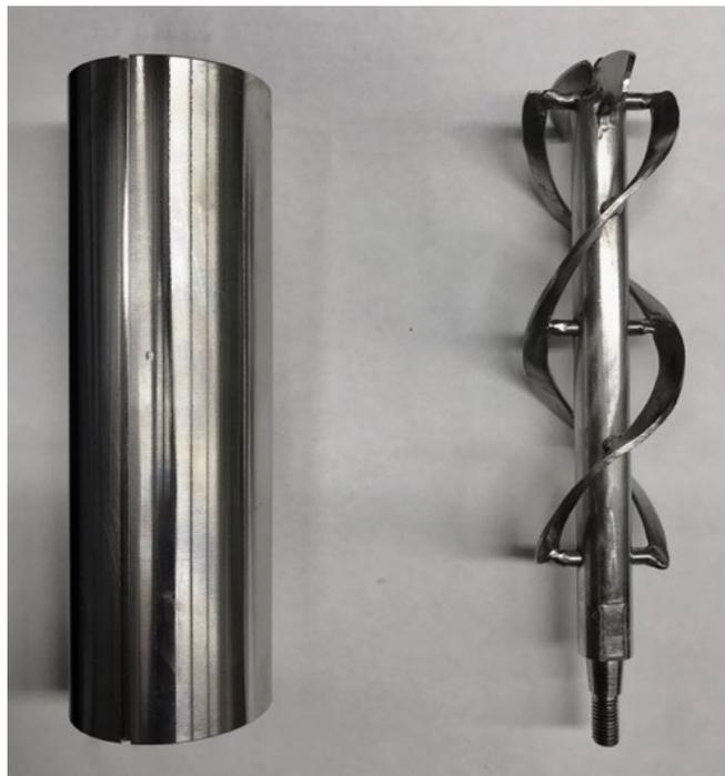
Figure 8. The stainless-steel extraction vessel sleeve (left) and the detached stainless-steel helical impeller (right).
