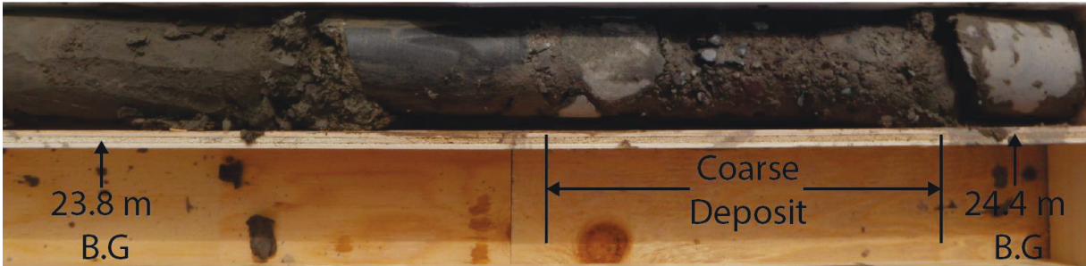
Figure 3-2 Coarse deposit within glaciolacustrine deposits at the Ripley Landslide
