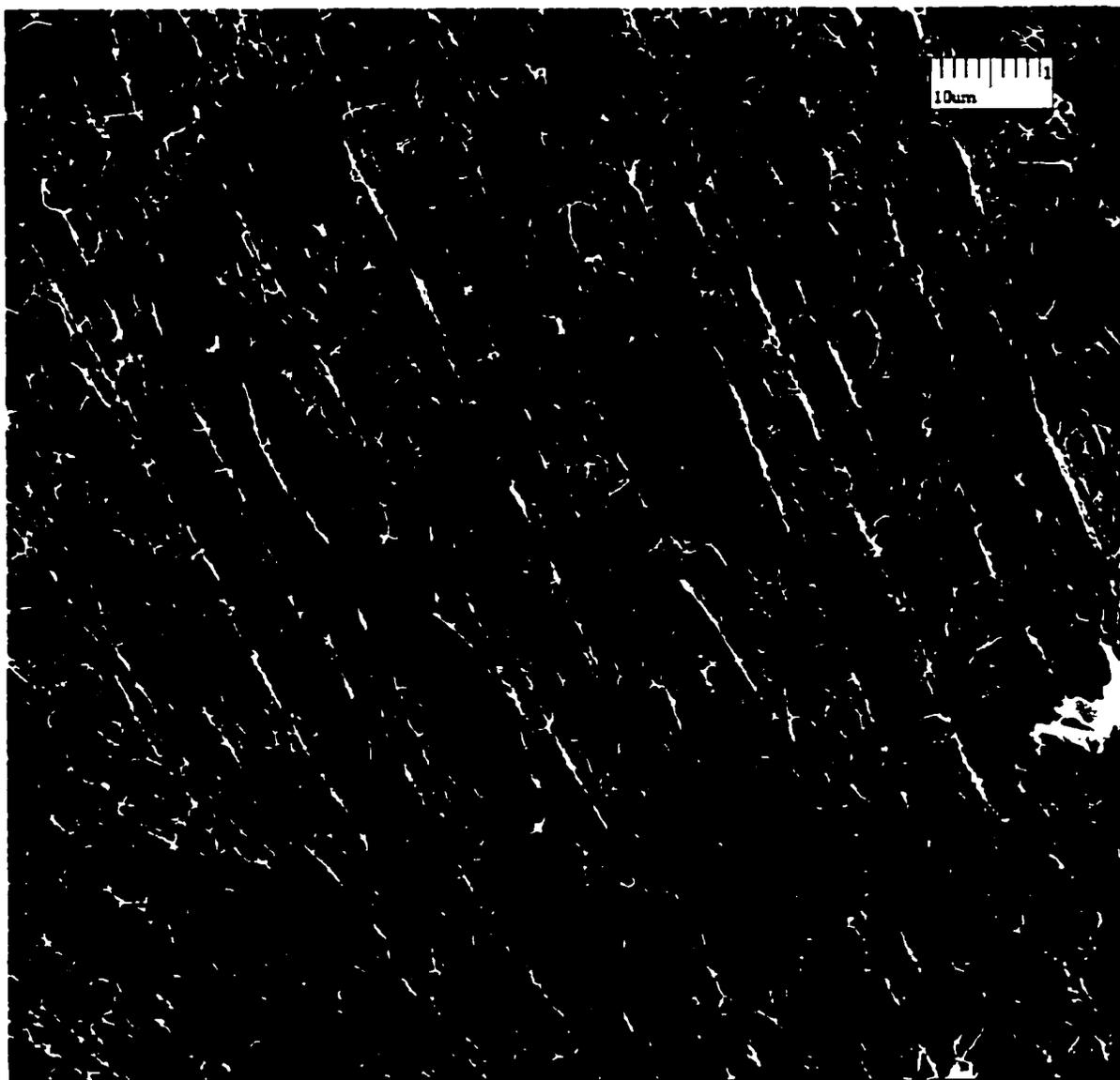
**Figure 5.8.** Scanning electron micrograph of 1% (w/w) fresh LAB solution ( $\times 1000$ ).
