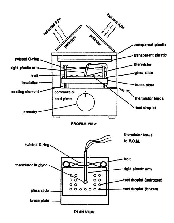
Figure 3.1: Schematic of equipment used in bulk nucleation experiments.
