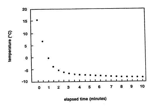
Figure 3.2: Cooling curve for the bulk nucleation apparatus diagrammed in Figure 3.1.
