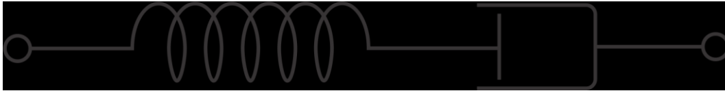
Figure 3.5: The Maxwell viscoelastic model, with spring (elastic component) and dashpot (viscous component) connected in series
