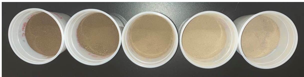
Figure 11. From left to right, DSBS with 2.0, 1.5, 1.0, 0.5 and 0 wt.% Bit. C.
