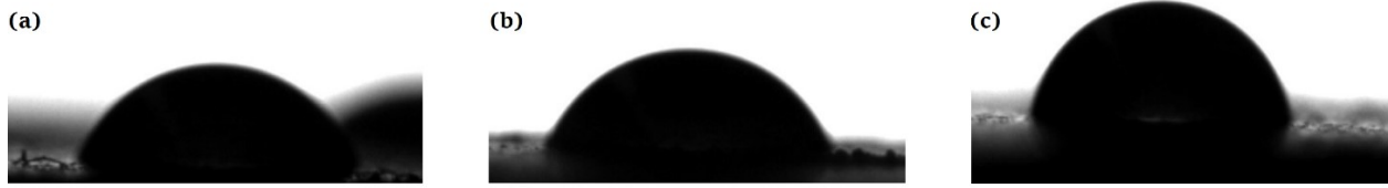
Figure 13. Photographs of water on pellets of boric acid and DSBS with (a) 0% (b) 10% and (c) 20% fines content.
