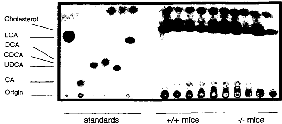
Fig. 6-8 Speciation of bile acids isolated from ilbp +/+ and ilbp -/- mice. Bile acids were extracted from the liver, gall bladder and small intestine of ilbp +/+ and ilbp -/- mice. Equivalent volumes of the extracts were spotted from 5 different mice in each group and resolved by HPTLC as detailed in Section 6.2.4. A. ilbp -/- mice produced a normal complement of conjugated bile acids (taurine to glycine) as compared to wild type mice. B. Free bile acids constituted a small portion of the bile acid pool of both ilbp +/+ and ilbp -/- mice, indicating that bile acids were metabolize in a similar manner in both strains. Spots running above or below the bile acid standards represent other lipid species (e.g. neutral lipids and phospholipids).
