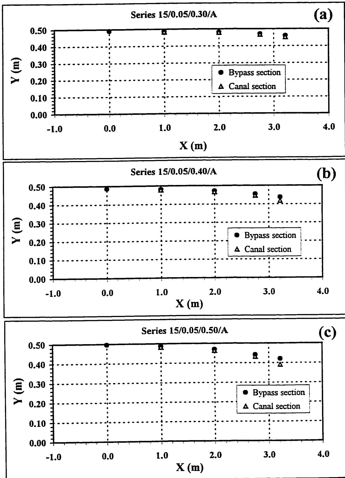
A-2.3(a-c): Depth Profiles of Bypass Section and Canal Section.
