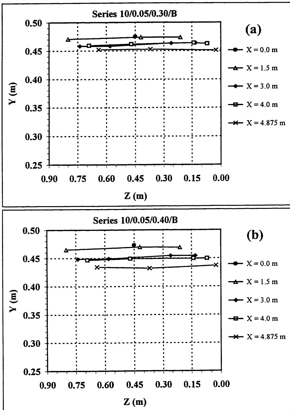
A-1.2(a-b): Depth Profiles of Bypass Section and Canal Section.
