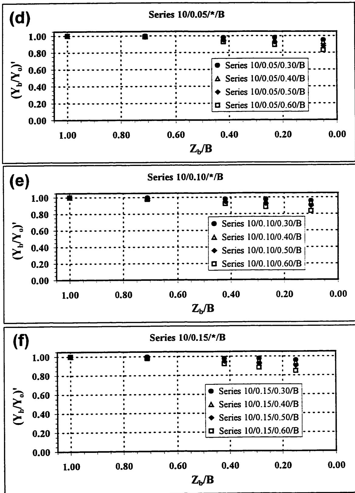
**Figures 9(d-f): Averaged Normalized Flow Depth versus Proportional Bypass Width.**
