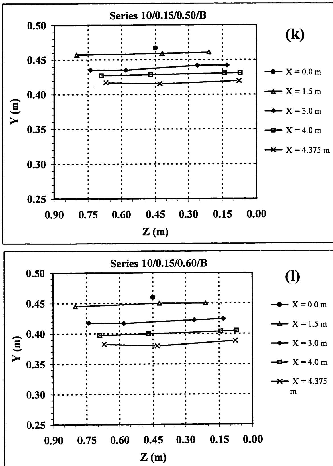
A-1.2(k-l): Depth Profiles of Bypass Section and Canal Section.
