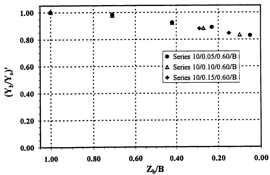
Figures 10(g-h): Averaged Normalized Flow Depth versus Proportional Bypass Width.
