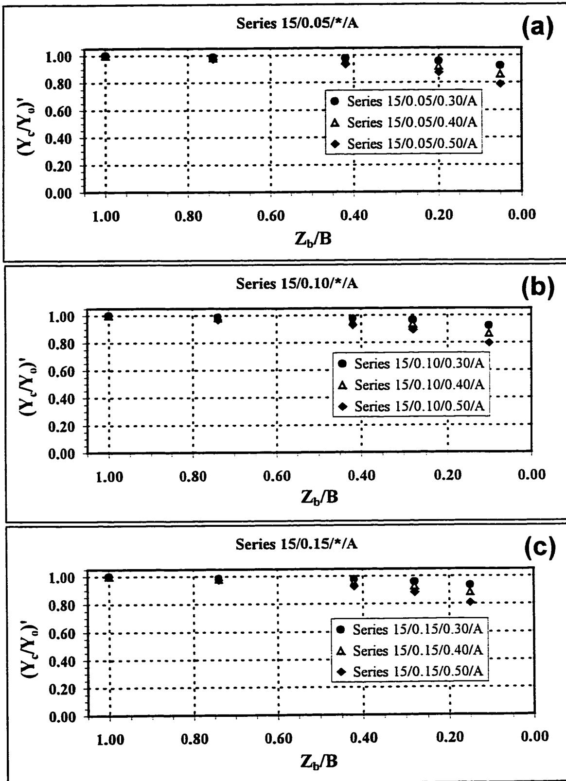
**Figures 15(a-c): Averaged Normalized Flow Depth versus Proportional Bypass Width.**
