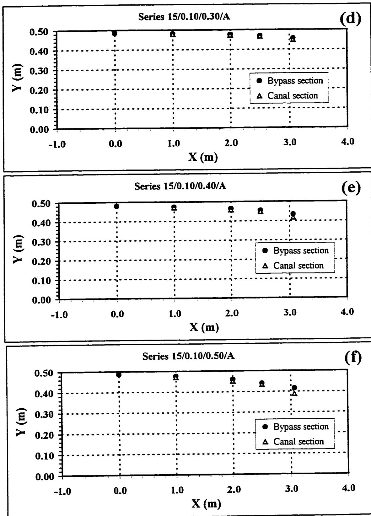
A-2.3(d-f): Depth Profiles of Bypass Section and Canal Section.
