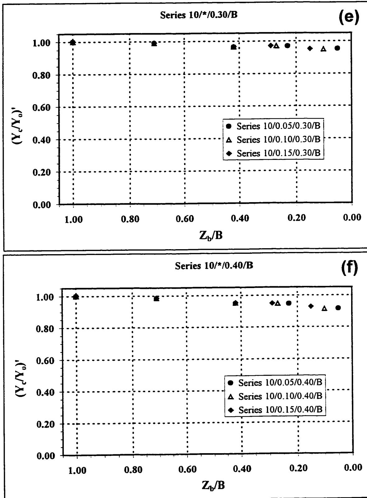
**Figures 12(e-f): Averaged Normalized Flow Depth versus Proportional Bypass Width.**
