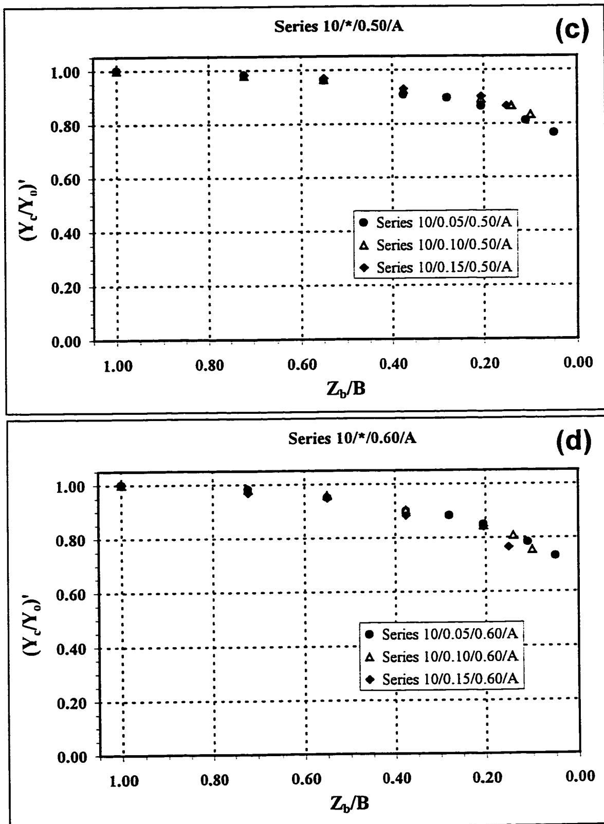
**Figures 12(c-d): Averaged Normalized Flow Depth versus Proportional Bypass Width.**
