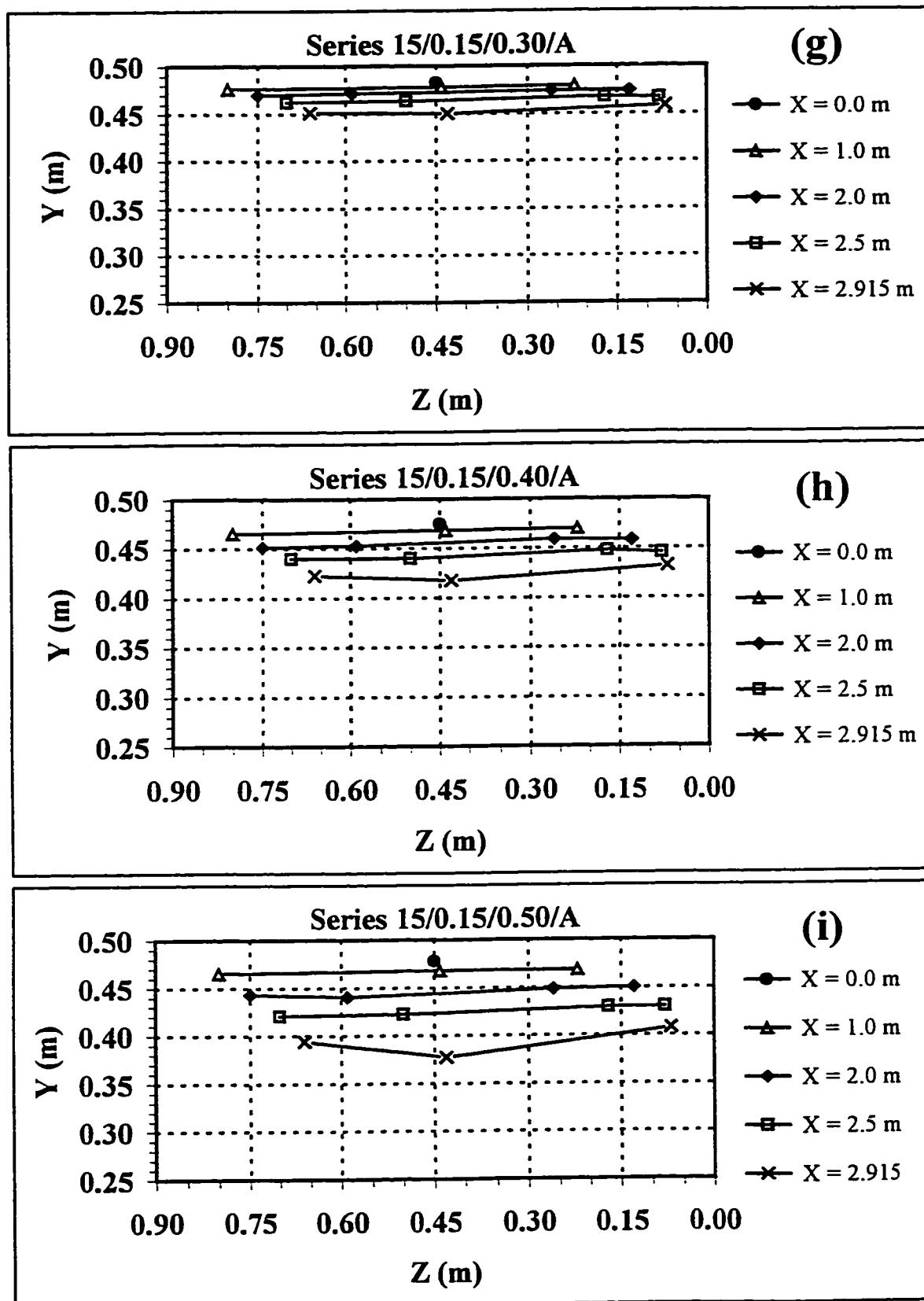
A-1.3(g-i): Depth Profiles of Bypass Section and Canal Section.
