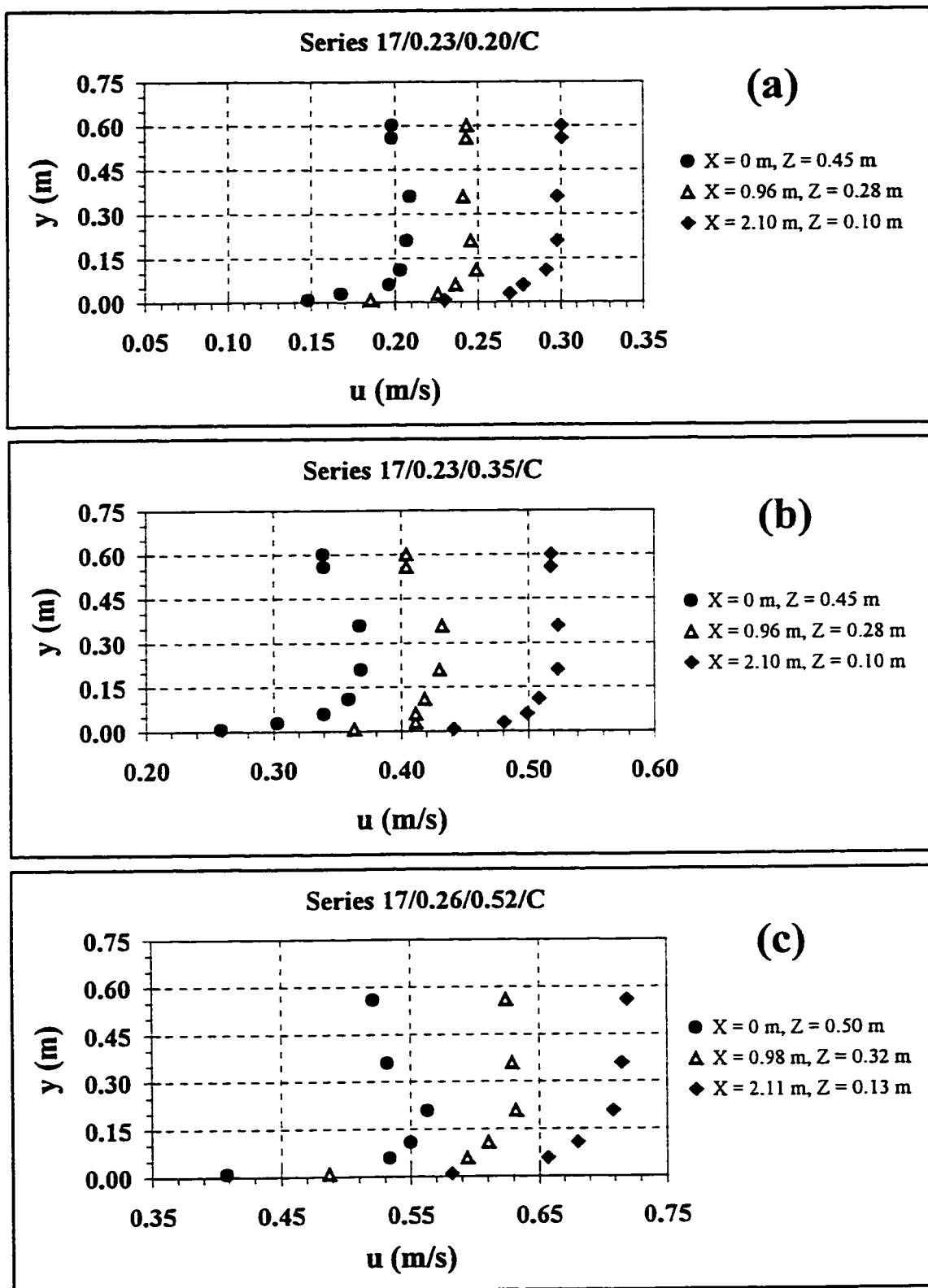
**Figures 18(a-c): Center-Plane Velocity Profiles Within the Fish Bypass Section.**
