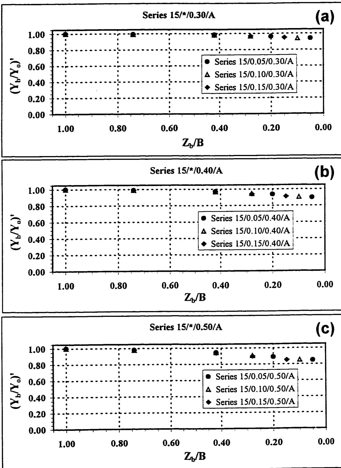
**Figures 14(a-c): Averaged Normalized Flow Depth versus Proportional Bypass Width.**
