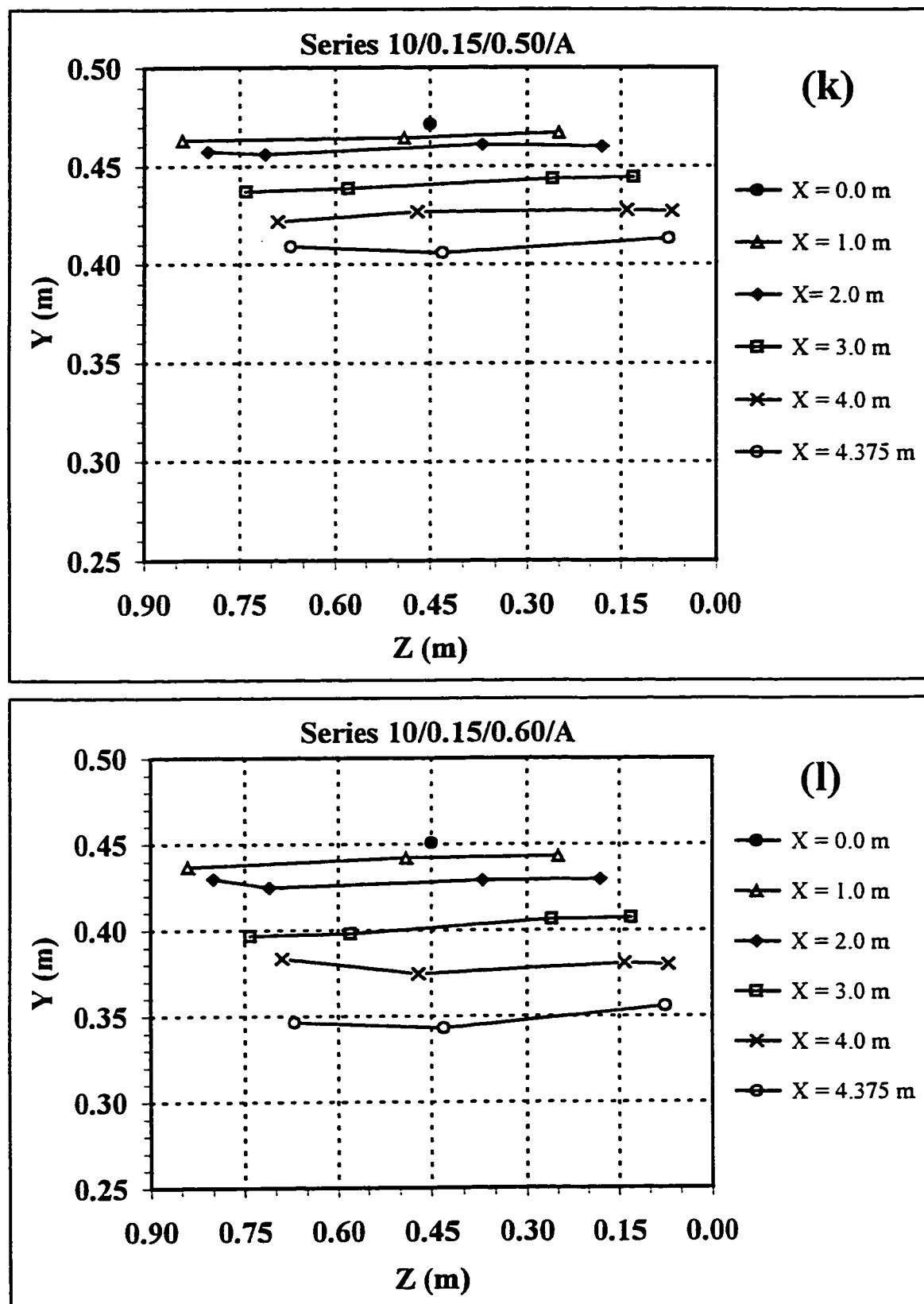
A-1.1(k-l): Depth Profiles of Bypass Section and Canal Section.
