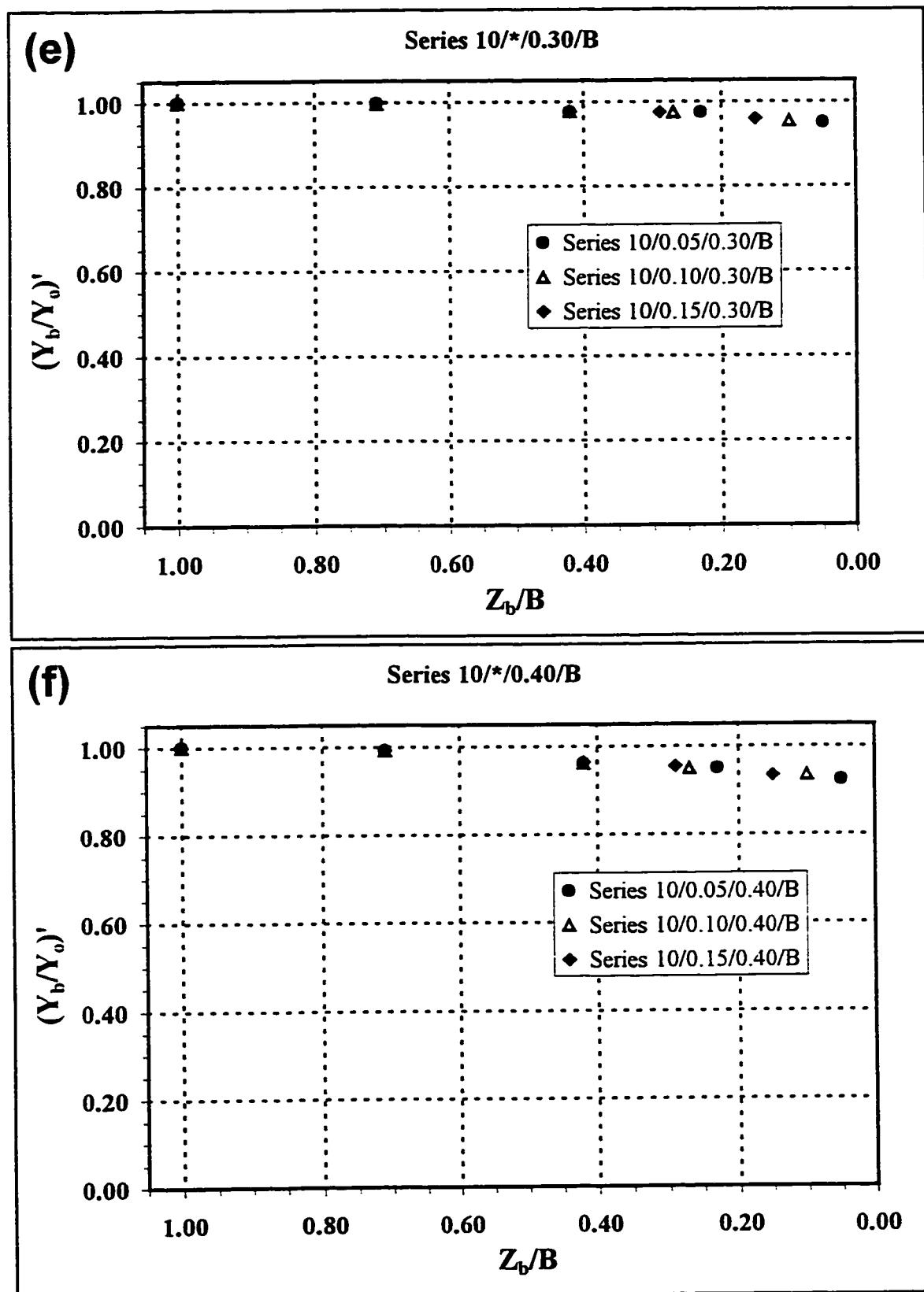
**Figures 10(e-f): Averaged Normalized Flow Depth versus Proportional Bypass Width.**
