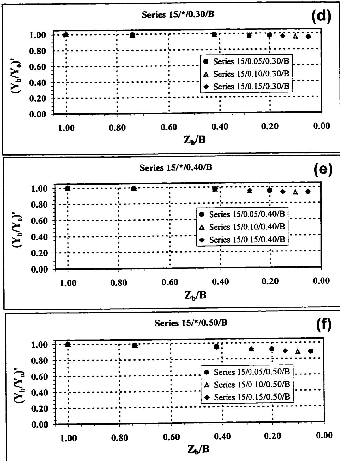
**Figures 14(d-f): Averaged Normalized Flow Depth versus Proportional Bypass Width.**
