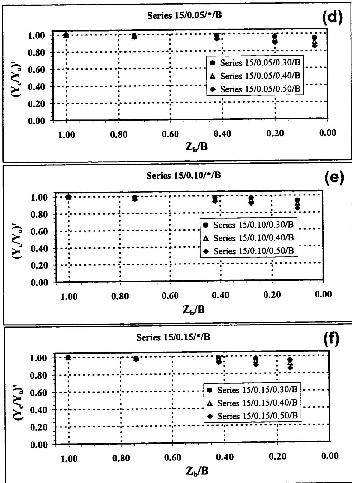
**Figures 15(d-f): Averaged Normalized Flow Depth versus Proportional Bypass Width.**
