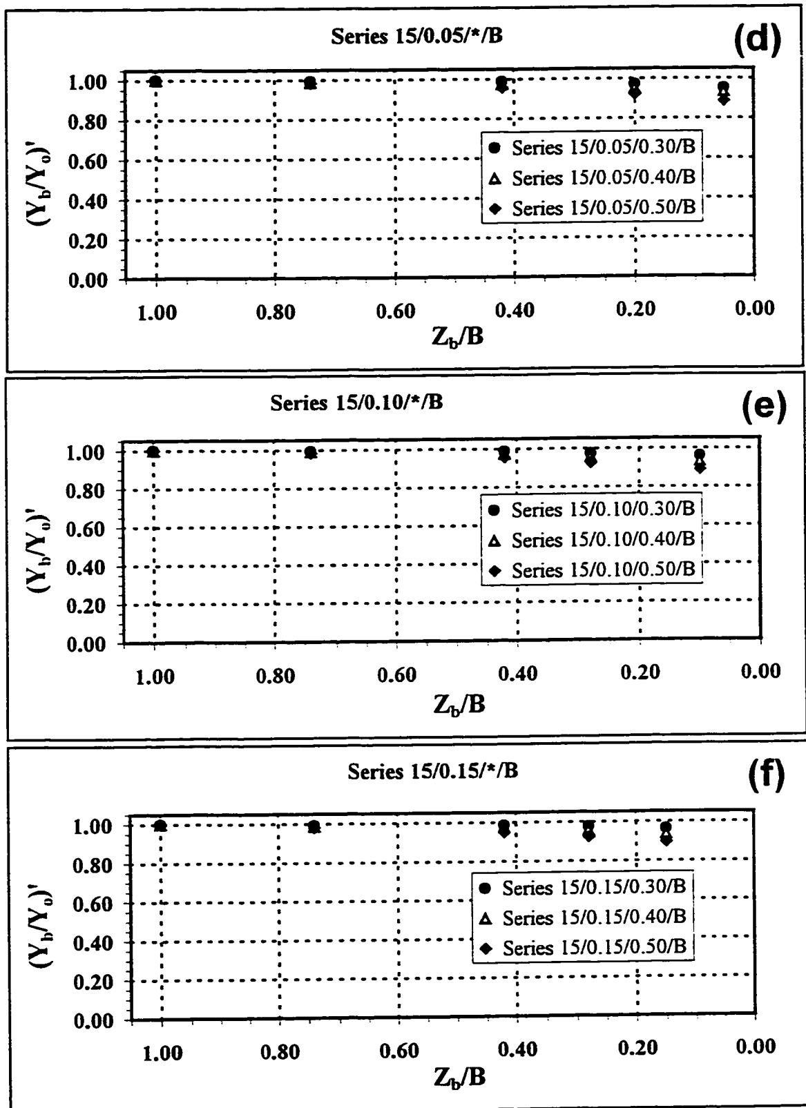
**Figures 13(d-f): Averaged Normalized Flow Depth versus Proportional Bypass Width.**
