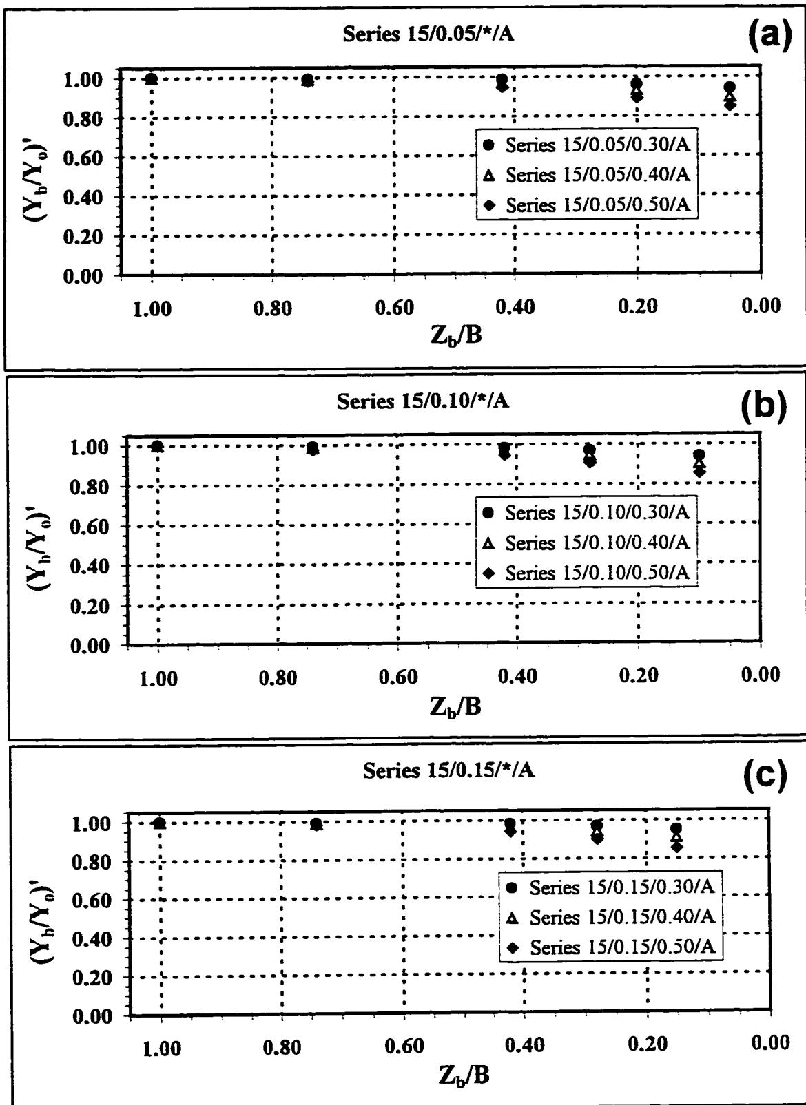
**Figures 13(a-c): Averaged Normalized Flow Depth versus Proportional Bypass Width.**
