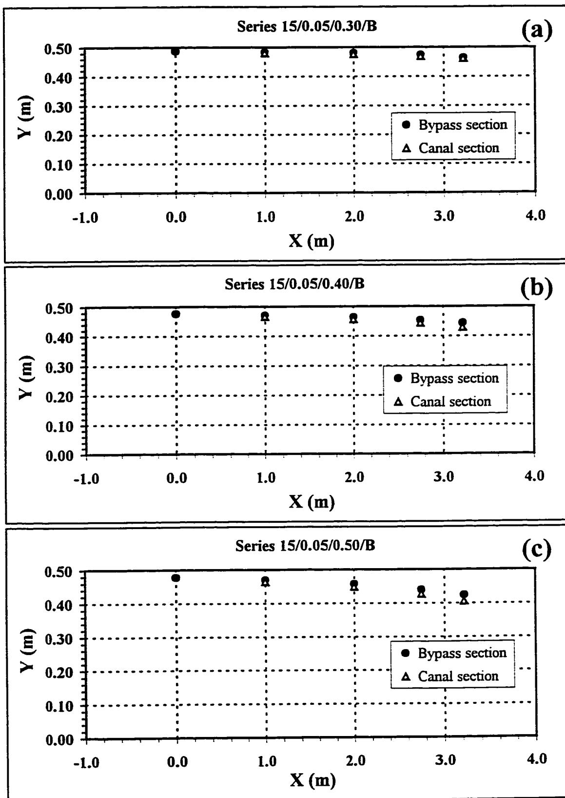
A-2.4(a-c): Depth Profiles of Bypass Section and Canal Section.
