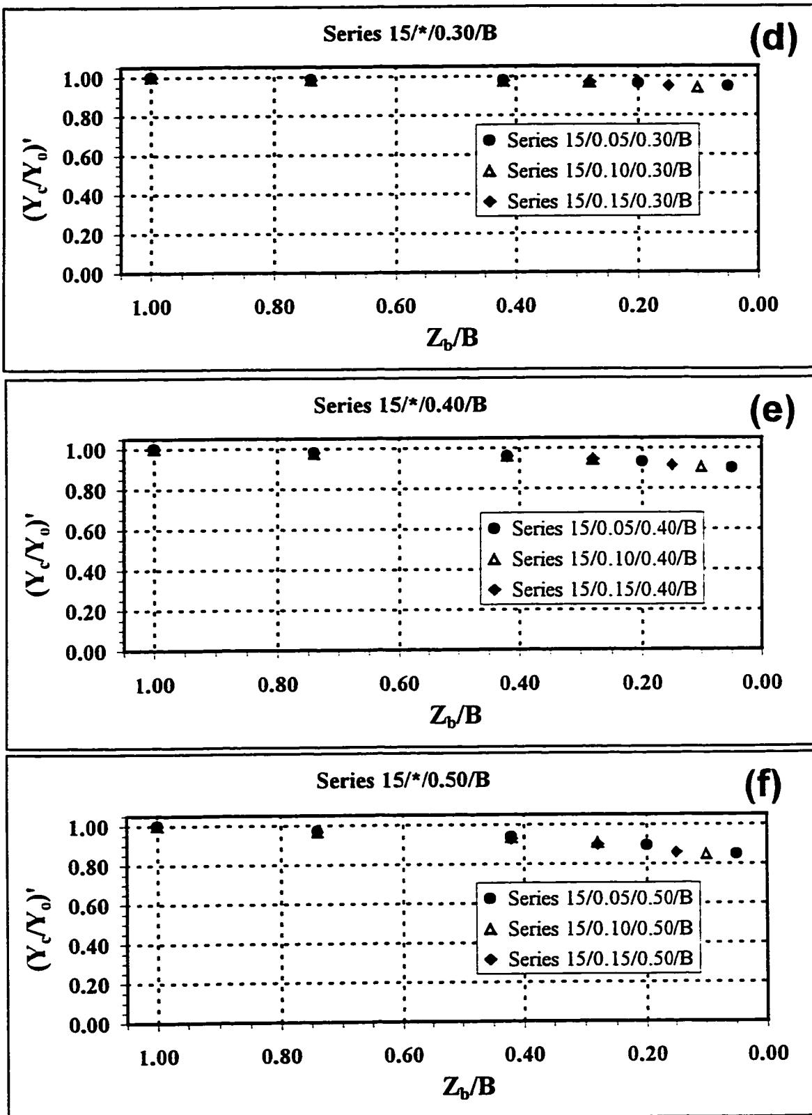
**Figures 16(d-f): Averaged Normalized Flow Depth versus Proportional Bypass Width.**
