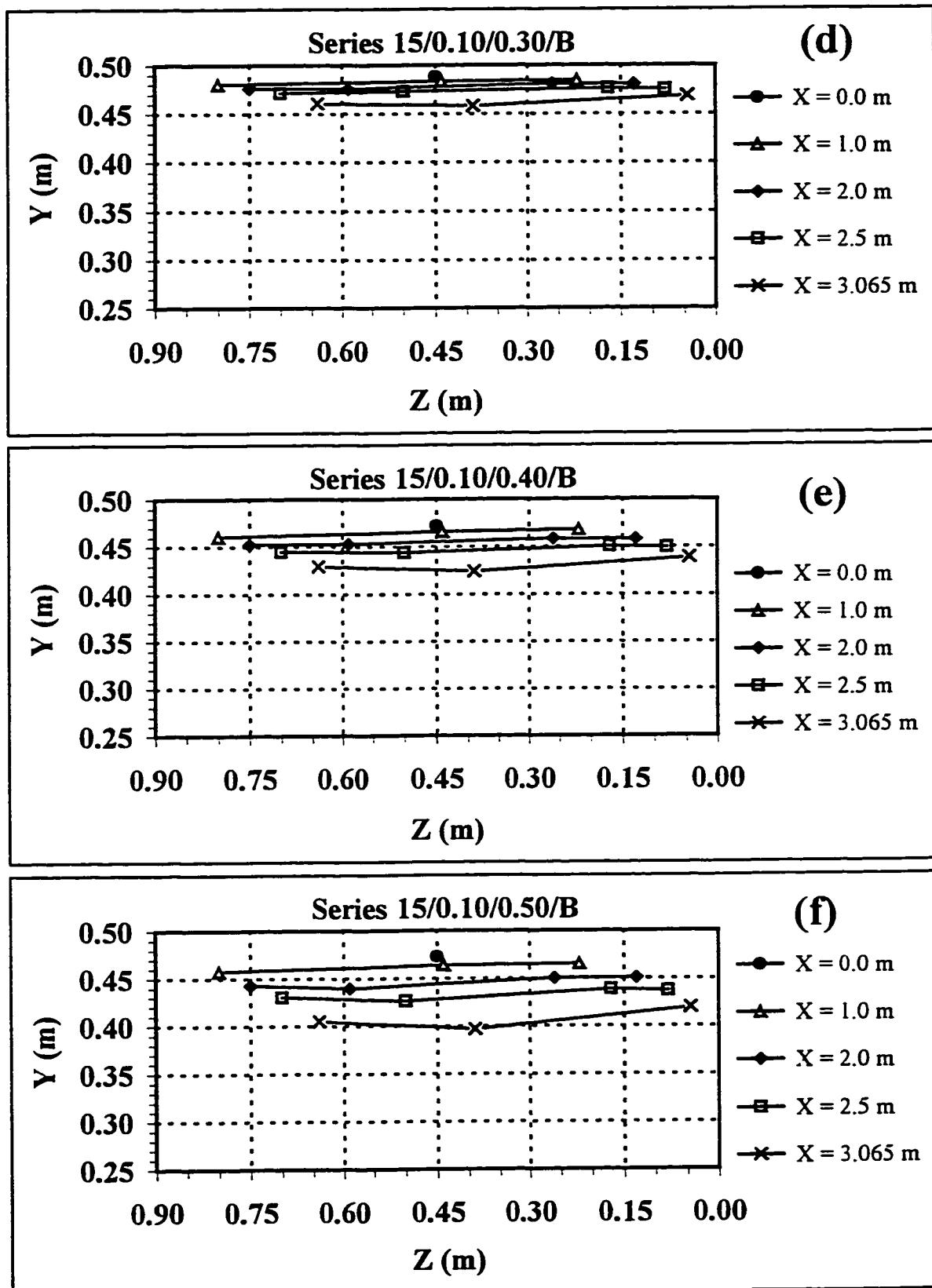
A-1.4(d-f): Depth Profiles of Bypass Section and Canal Section.
