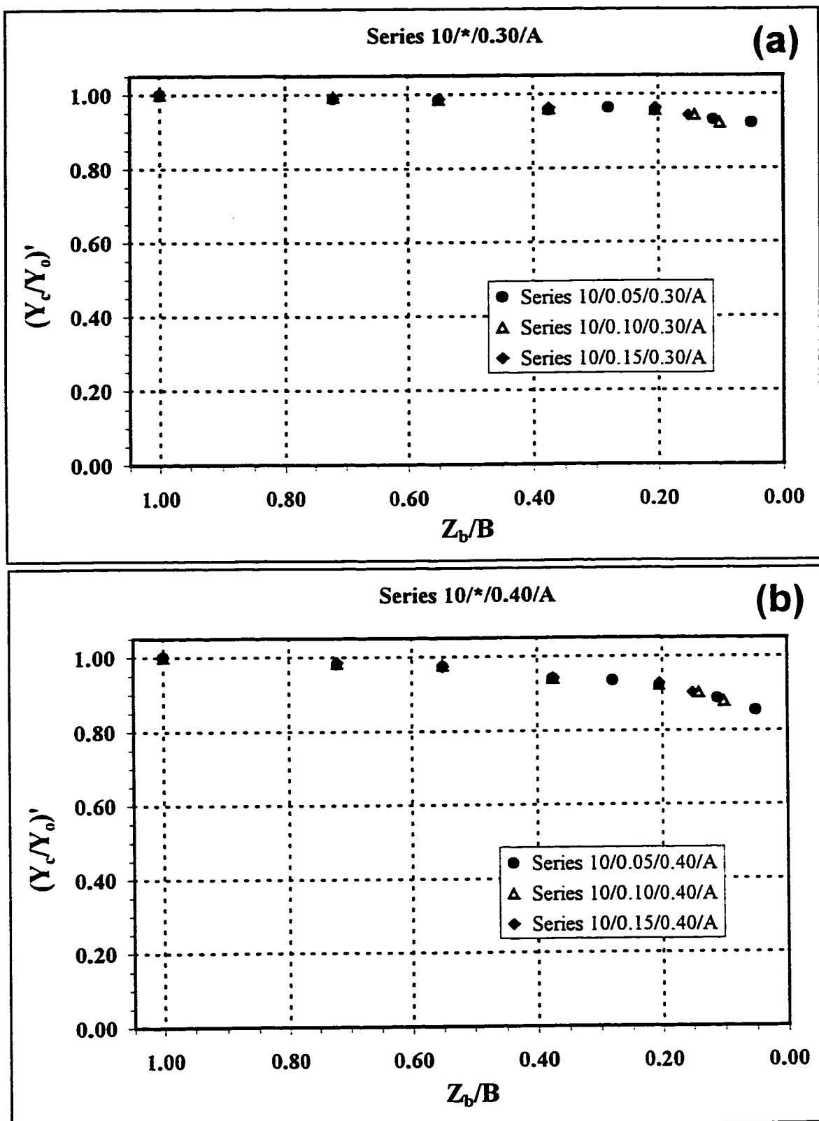
**Figures 12(a-b): Averaged Normalized Flow Depth versus Proportional Bypass Width.**
