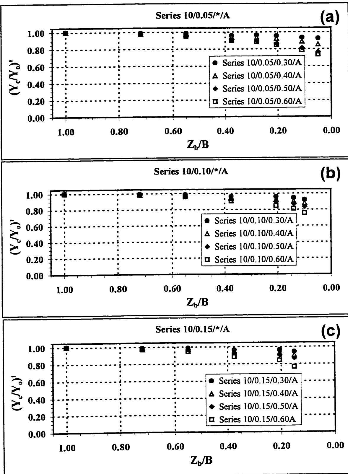
**Figures 11(a-c): Averaged Normalized Flow Depth versus Proportional Bypass Width.**
