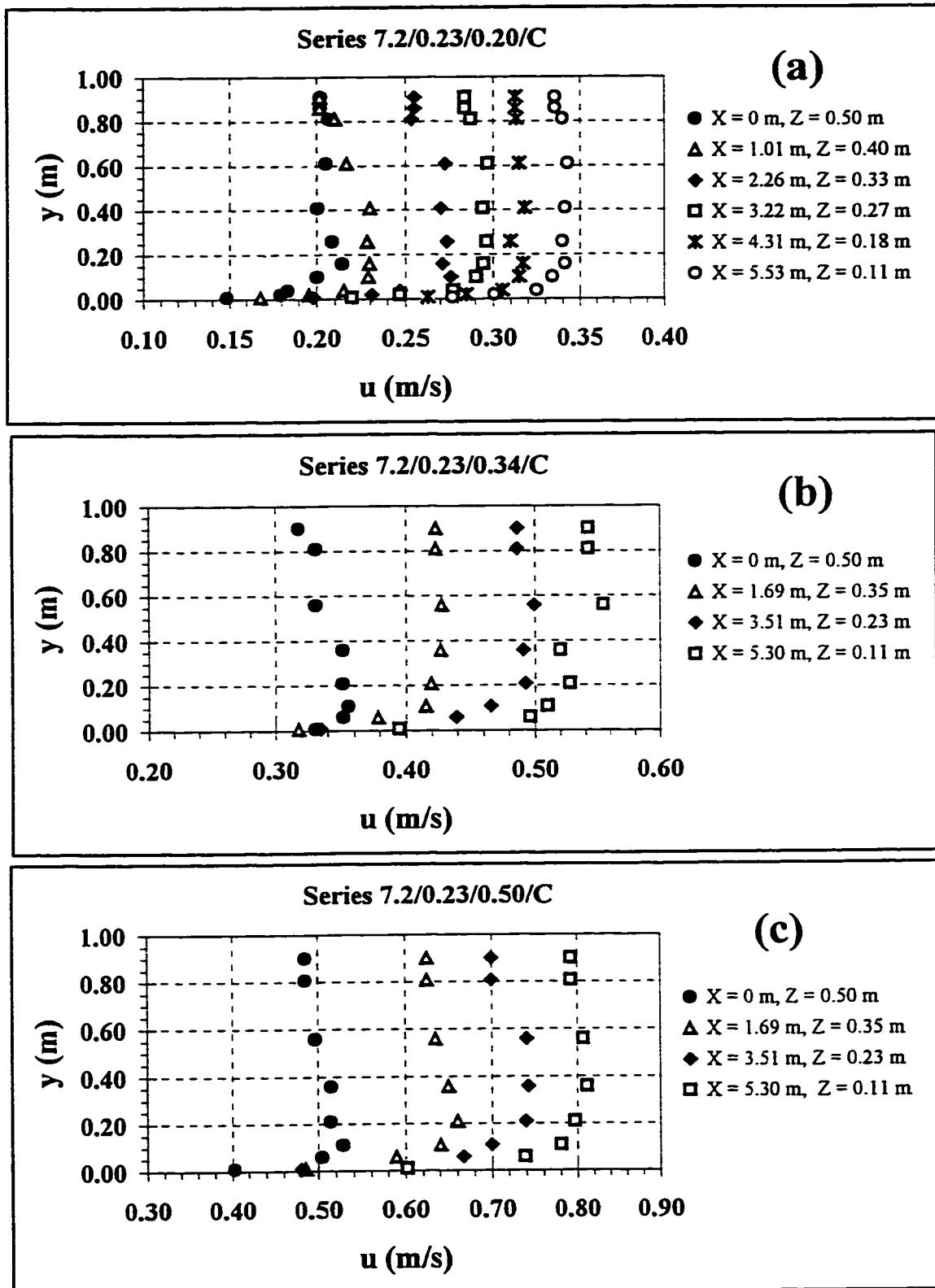
**Figures 17(a-c): Center-Plane Velocity Profiles Within the Fish Bypass Section.**
