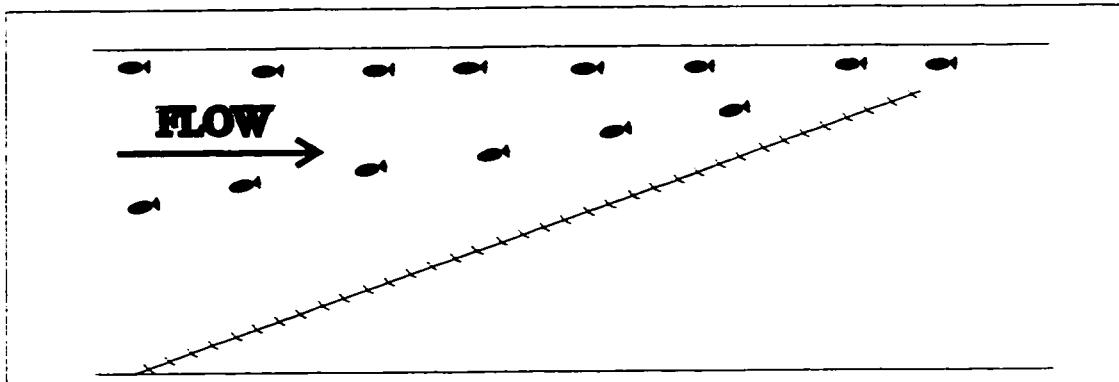
Figure 3: Representation of a typical fish movement along the louver array.
