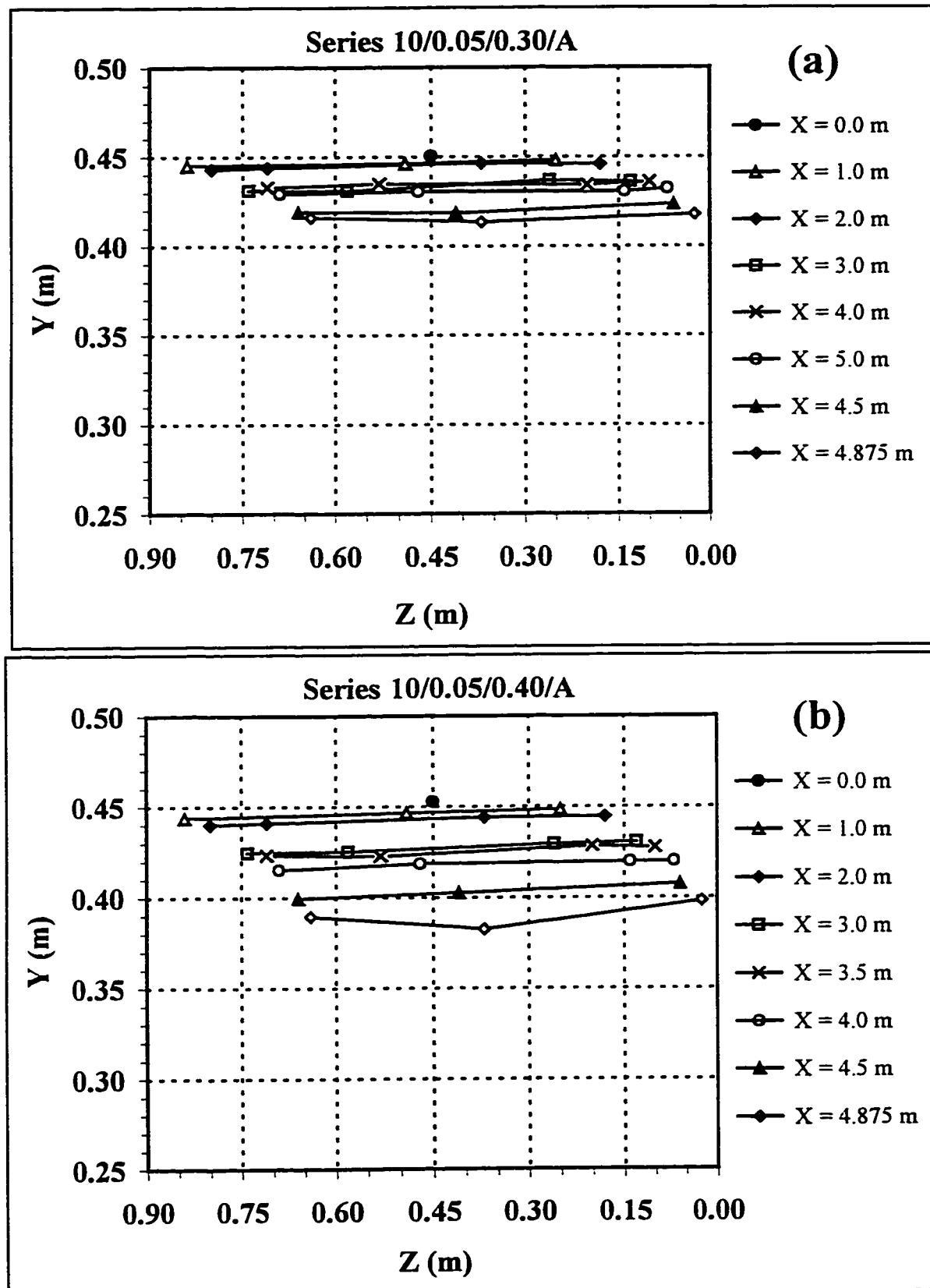
**A-1.1(a-b): Depth Profiles of Bypass Section and Canal Section.**
