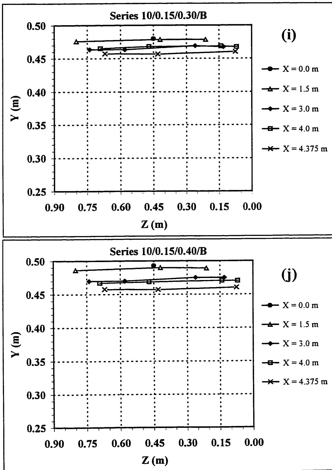
A-1.2(i-j): Depth Profiles of Bypass Section and Canal Section.
