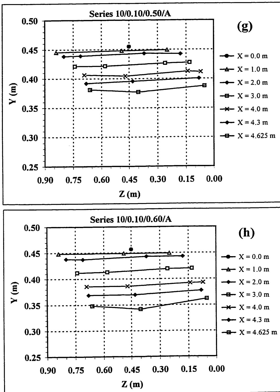
A-1.1(g-h): Depth Profiles of Bypass Section and Canal Section.
