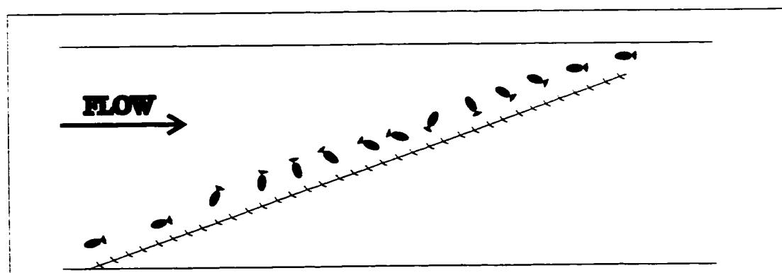
Figure 5: Representation of a typical fish movement along the louver array.
