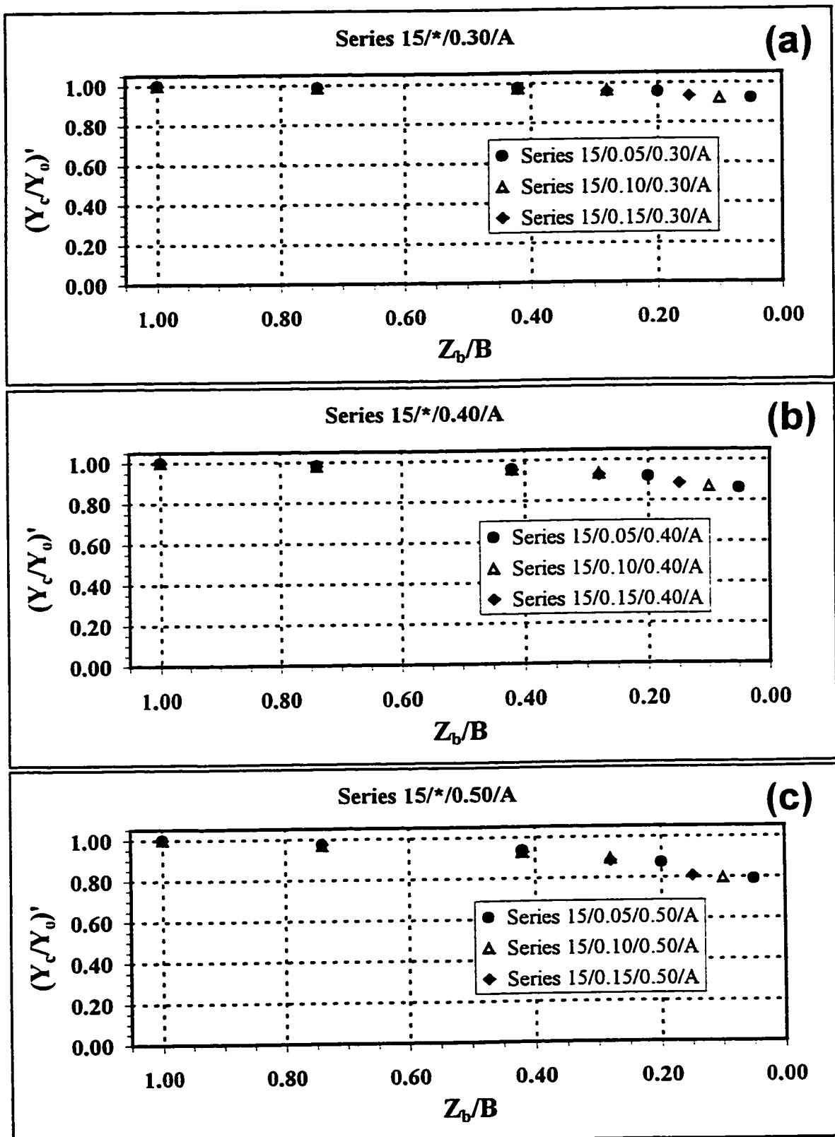
**Figures 16(a-c): Averaged Normalized Flow Depth versus Proportional Bypass Width.**
