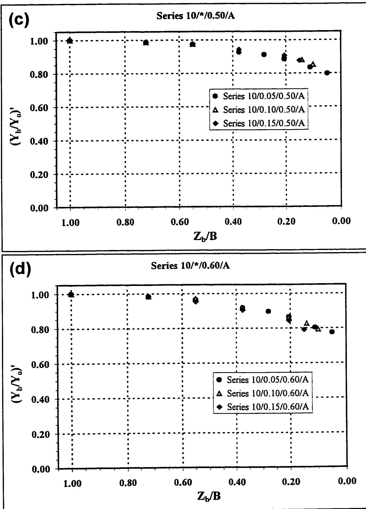
Figures 10(c-d): Averaged Normalized Flow Depth versus Proportional Bypass Width.
