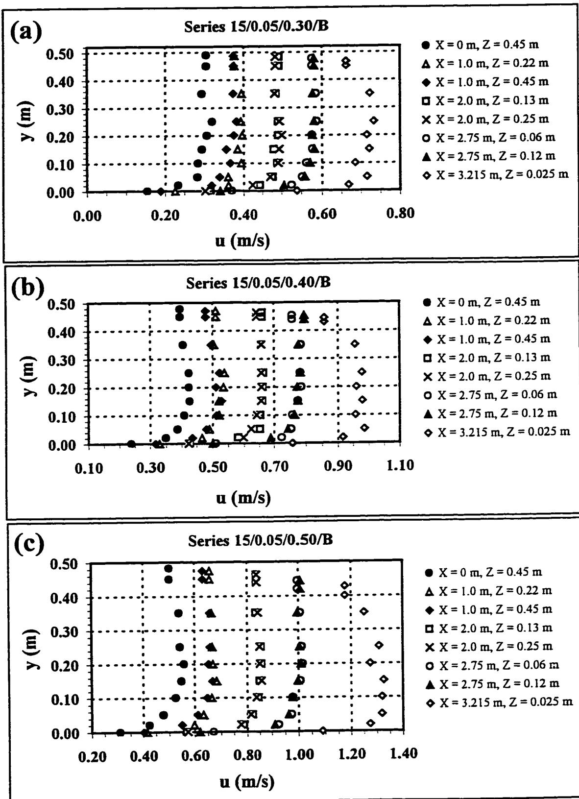
Figures 24(a-c): Velocity Profiles Within the Fish Bypass Section.
