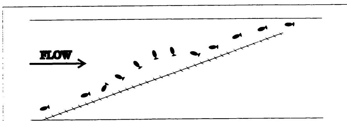
Figure 4: Representation of a typical fish movement along the louver array.
