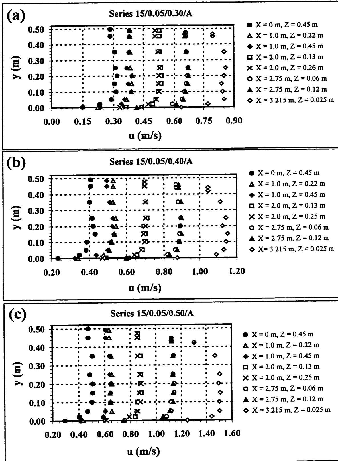
Figures 23(a-c): Velocity Profiles Within the Fish Bypass Section.
