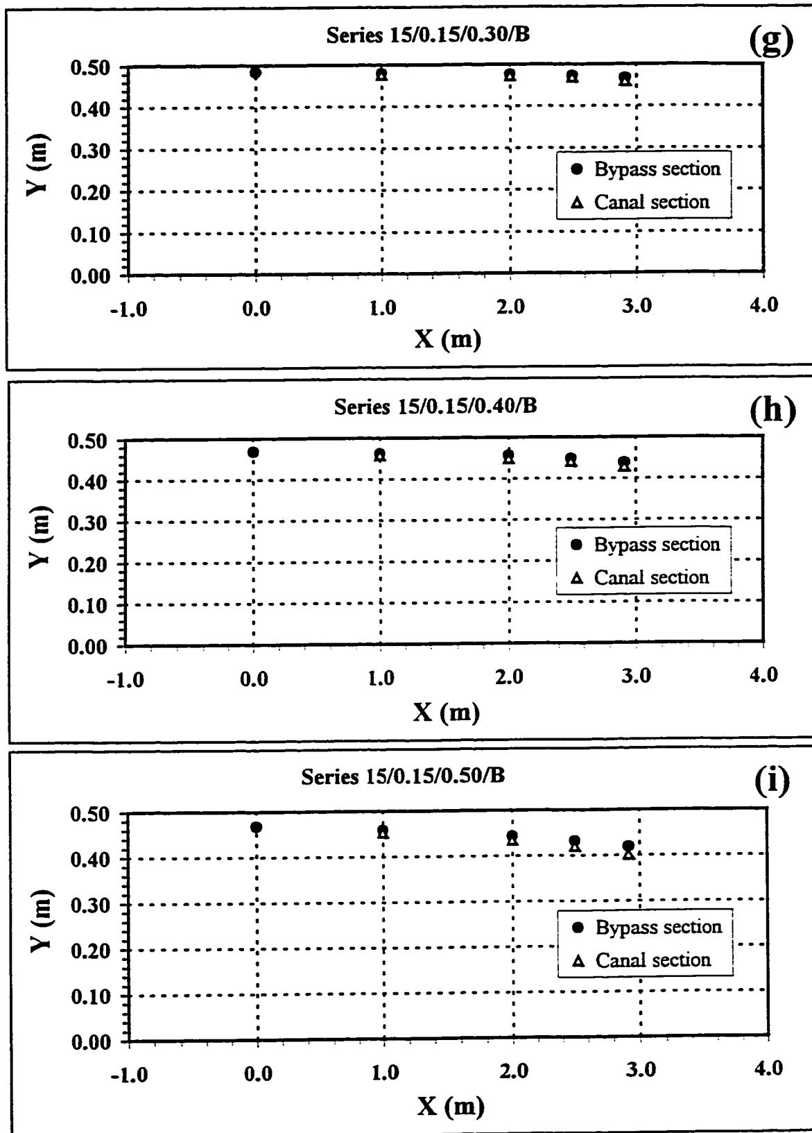
A-2.4(g-i): Depth Profiles of Bypass Section and Canal Section.
