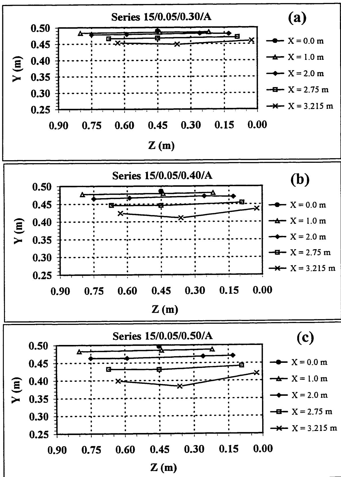
A-1.3(a-c): Depth Profiles of Bypass Section and Canal Section.
