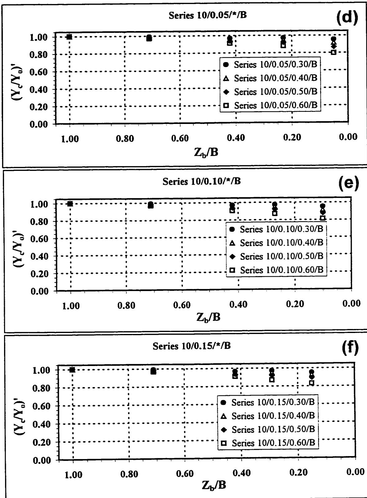
**Figures 11(d-f): Averaged Normalized Flow Depth versus Proportional Bypass Width.**
