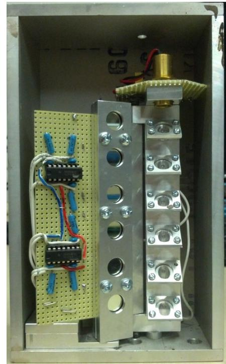
Figure 4-14 – Centrifuge sensor. Signal amplifiers on perforated board at left, and laser diode driver on perforated board at top. Detectors covered by bandpass filters at center, and glass beam splitters at right.
