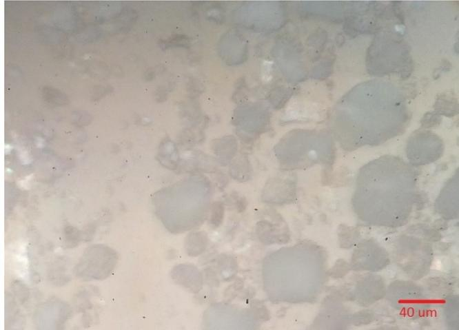
Figure 4-8 – A microscope picture taken of Kaolin powder showing range of particle sizes and irregularity of shape.
