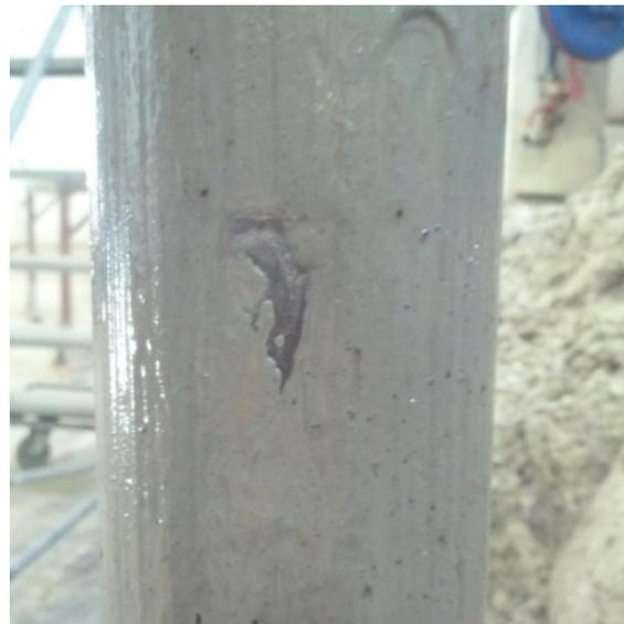
**Figure 4-24 – Clear section on the upper part of the window after the tube was removed. This is possibly caused by air bubbles, which may have affected measurements from the red laser diodes.**
