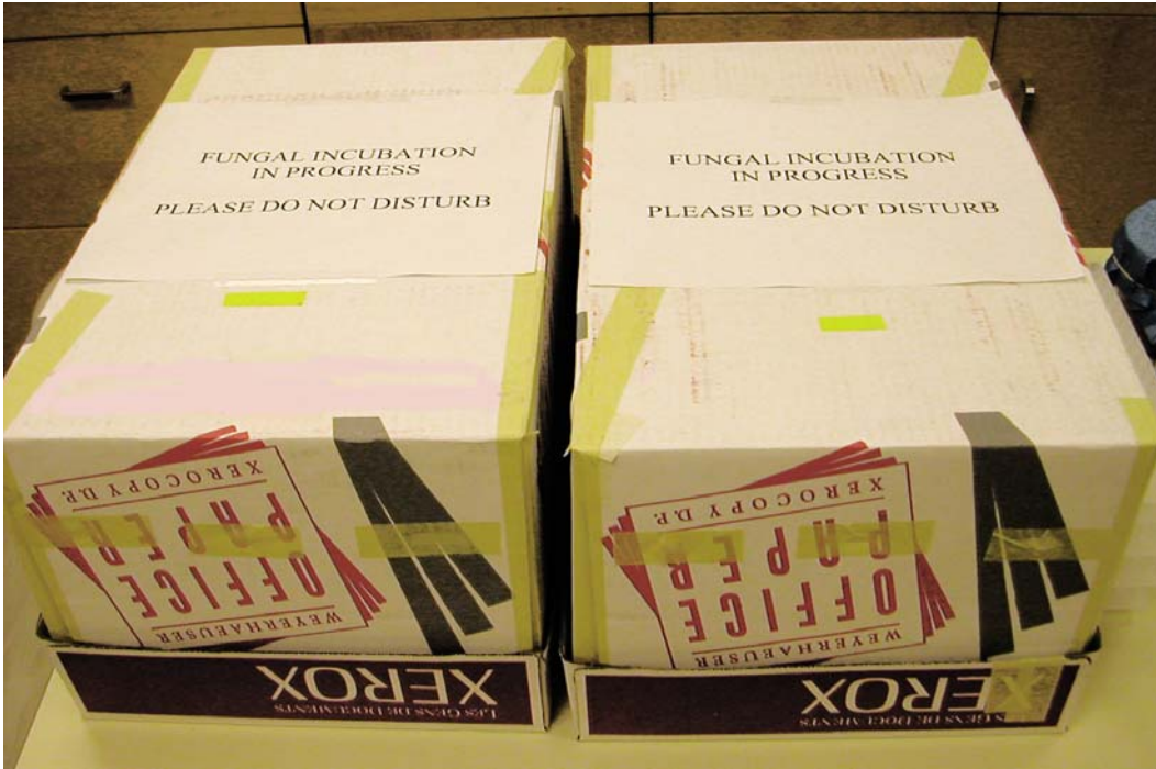
Figure 2.4. Dark incubation chambers. Interior chambers were lined with thick black construction paper and any potential light leaks were sealed with masking tape. No light penetration (zero foot-candles) was confirmed using a hand-held light meter. This and other images taken with Nikon Coolpix® 775 digital camera.
