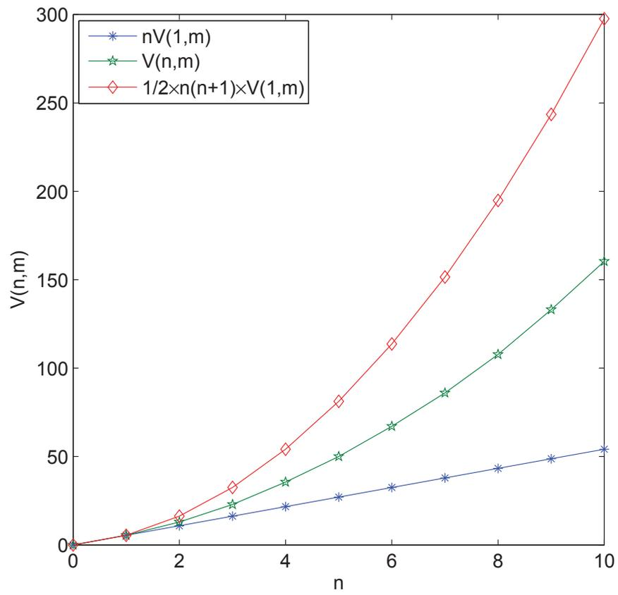
Fig. 4.3.  $V(n, m)$  and its lower and upper bounds versus  $n$  when  $m = 30$ .
