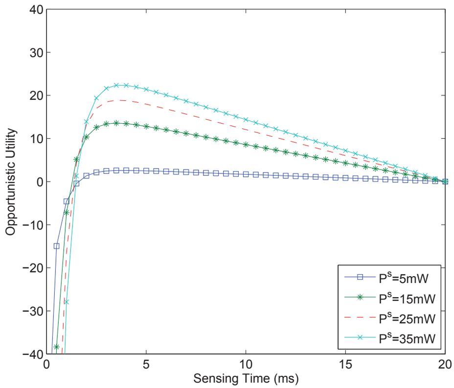
Fig. 3.5. Secondary user utility versus sensing time.
