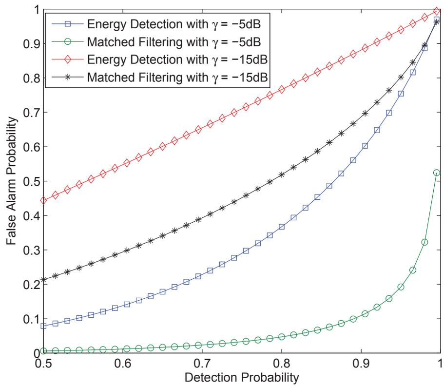
Fig. 2.1. Comparison of matched filter detection and energy detection.
