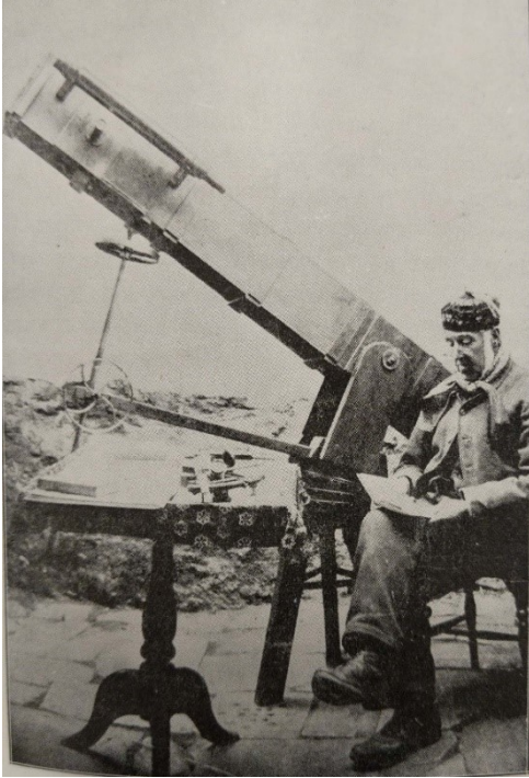
Figure 6. Jones with his 8-inch homemade reflecting telescope, Jumbo. J. Silas Evans, Seryddiaeth a Seryddwr (Cardiff: William Lewis, 1923), 273.
