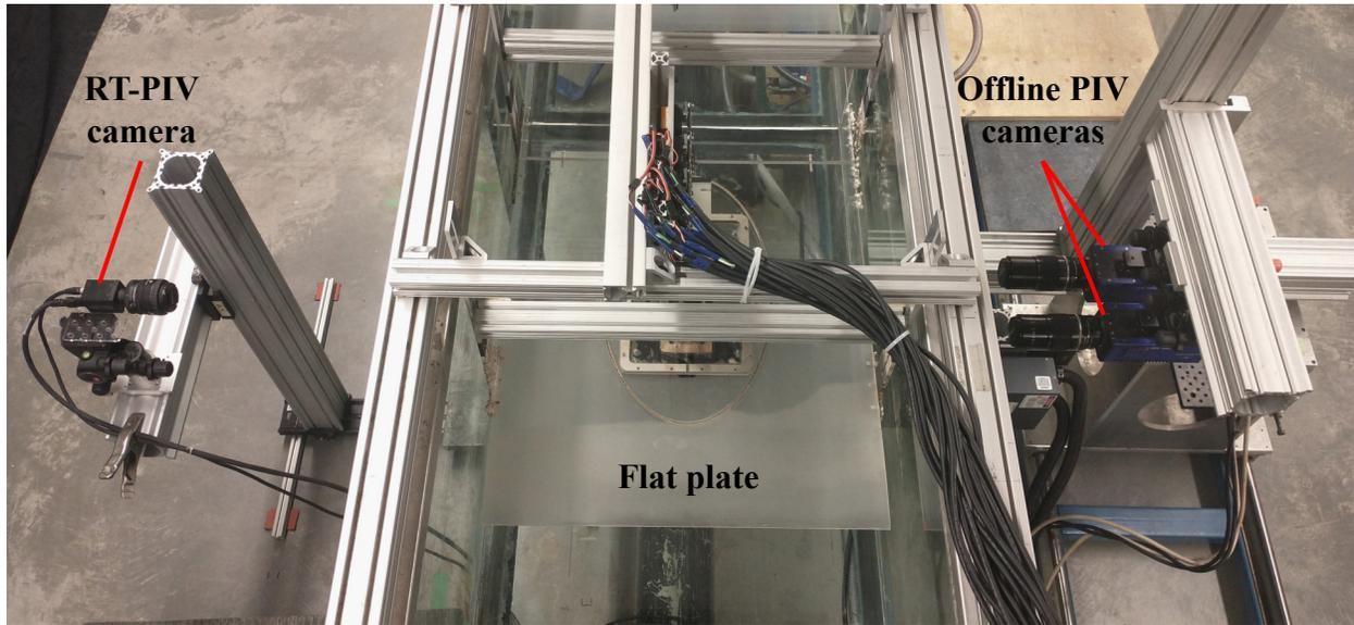
Figure 3.8: Photograph of the RT-PIV and offline PIV cameras on opposite sides of the water flume.
