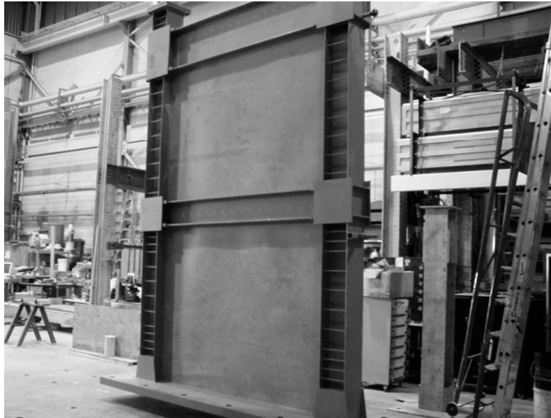
Figure 2.17: Test specimen before concrete was cast (Deng et al. 2008)
