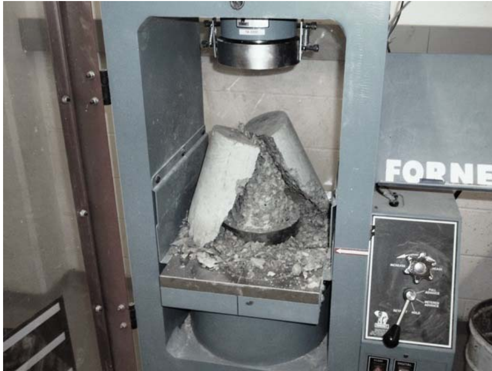
Figure 4.22: “Split and cone” type of failure of the concrete cylinder in compression test
