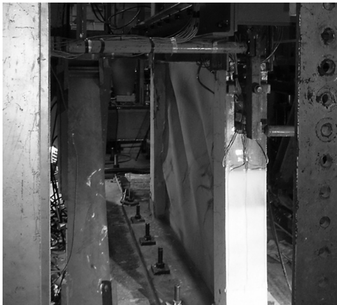
Figure 6.8: Effect of the vertical tear in the infill plate, adjacent to south column, on the buckled shape of the infill plate of the first story during cycle 25 (from north).
