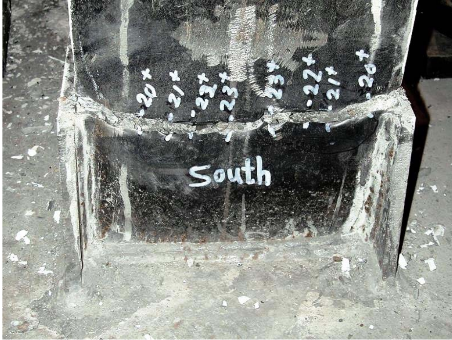
Figure 5.7: Outer flange of the south column at the base in cycle 24
