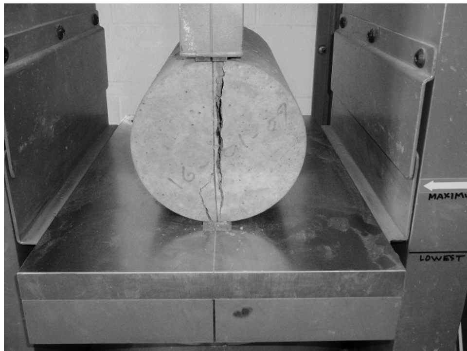
Figure 4.23: The concrete split cylinder test to determine the tensile strength of concrete
