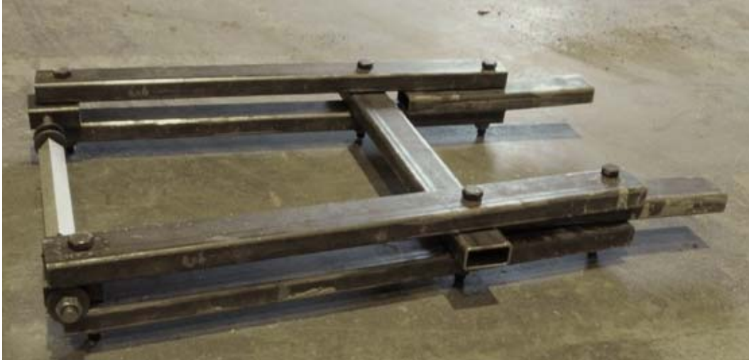
Figure 4.15: Hand-made formwork clamps
