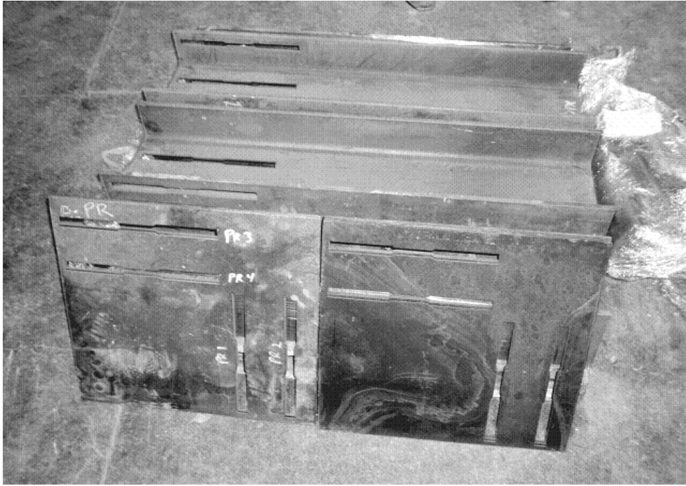
Figure 4.20: Remaining material after the coupons were removed
