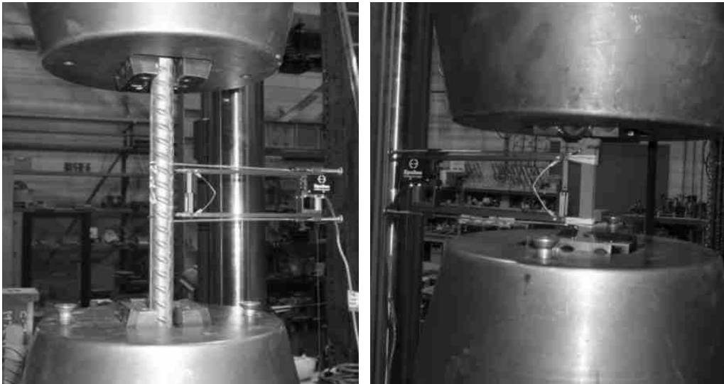
Figure 4.21: Tension test of the coupons taken from the 25M rebar (left) and the column plate (right)
