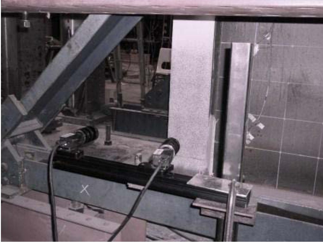
Figure 4.14: One set of cameras, monitoring the concrete face of PEC column at base
