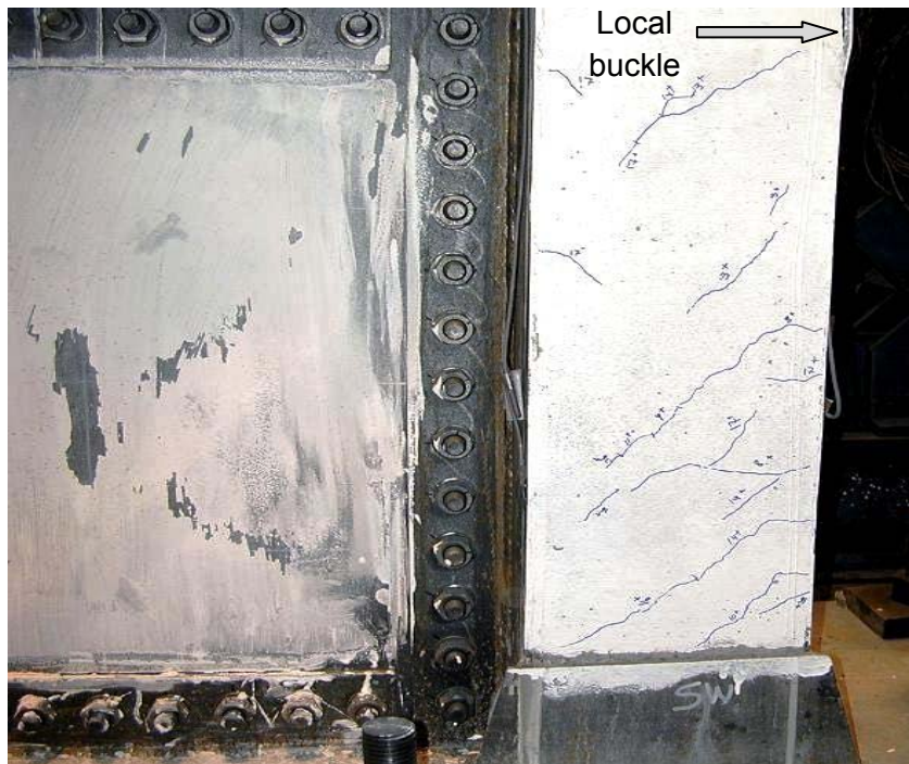
Figure 5.4: Base of the south column during cycle 17
