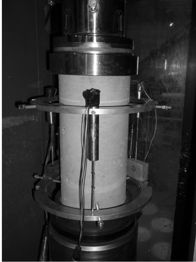
Figure 4.24: Compression test to obtain the stress vs. strain material properties of the concrete cylinder
