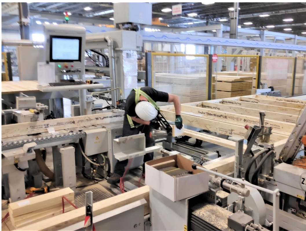
Figure 4-3. Framing station (installation of studs between top and bottom plates)
