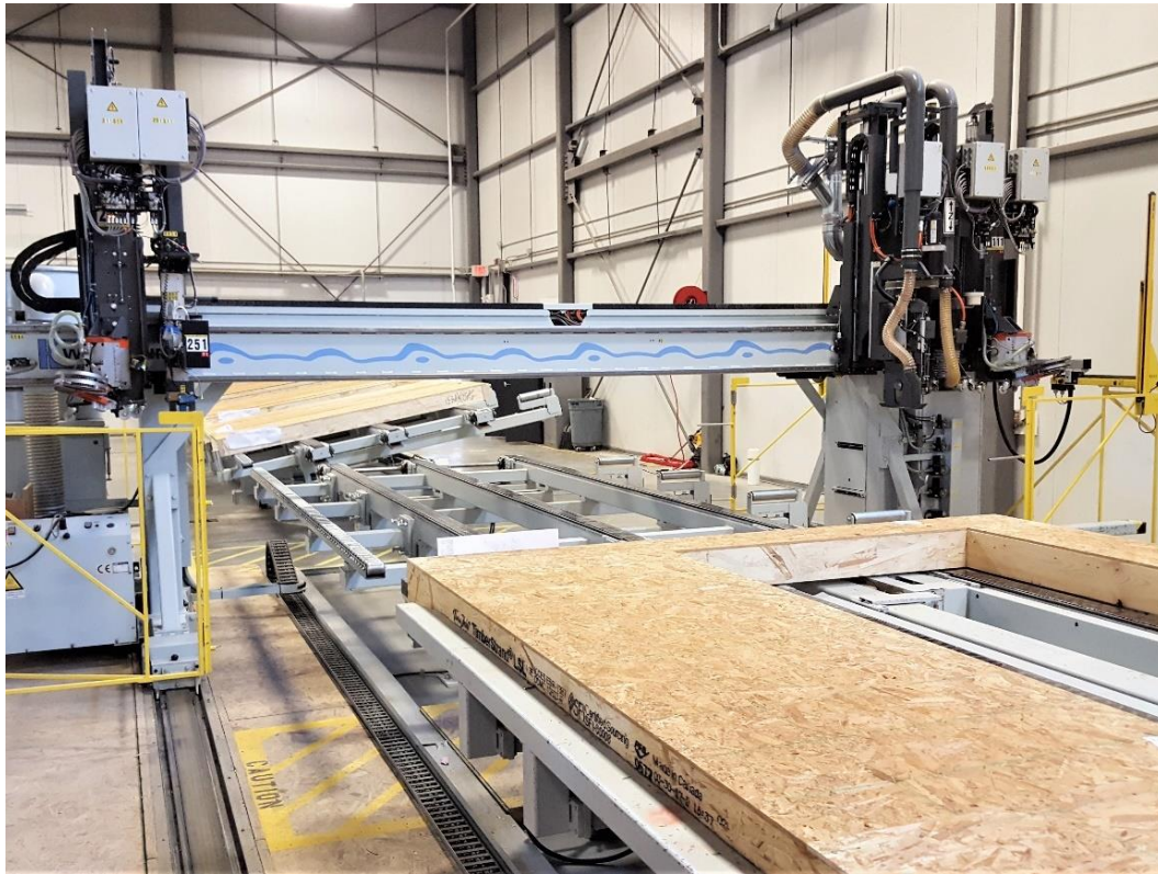
Figure 4-5. Multifunction bridge (at initial position when receiving a wall panel)
