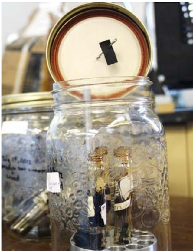
**Figure 3-2:** Photo of a setup for activated carbon strip extraction of volatile components from simulated arson debris.
