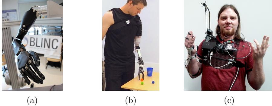
Figure 3.1: Prostheses examples: (a) robotic upper-limb prosthetic, (b) human using a research prosthesis (Dawson et al., 2014), (c) human using a supernumerary limb (A. S. R. Parker et al., 2019a).
