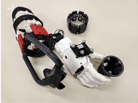
Figure 7.1: The brace restricts motion of the wearer’s wrist, which encourages isometric contraction to “simulate” muscles in a residual limb. The brace also allows the robot hand to be placed in front of the user’s biological hand. Reusable cups 3D printed from NinjaFlex with the same shape but different stiffnesses. EMG signals were captured using the Myo armband.
