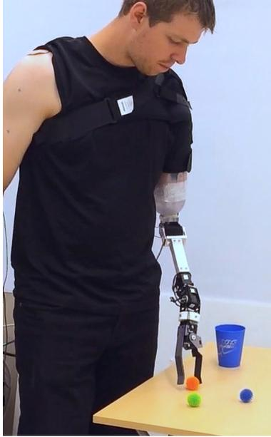
Figure 2.2: An individual with an amputation interacting with their environment in collaboration with an electromechanical prosthesis—in this case the Bento Arm (Dawson et al., 2014) and brachi/Oplexus software (Dawson et al., 2020), a robotic limb suite integrating reinforcement learning algorithms and classical prosthetic control solutions.
