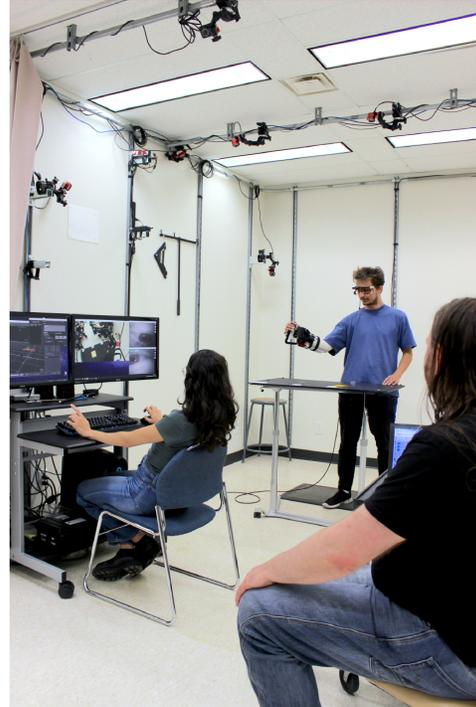
Figure 7.2: Gaze and Movement Analysis (GaMA) combines gaze vector and motion capture data. The participant wears glasses with eye-tracking cameras, and fixed motion capture cameras record the motion capture markers on lab equipment. The laptop is running the robot software. All three data streams are recorded and synchronized using Lab Streaming Layer.
