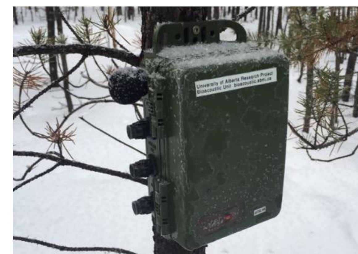
Figure 3: An acoustic monitoring device set up to record sounds in Cooking Lake-Blackfoot Provincial Recreation Area (photo: Jeremiah Kennedy)
